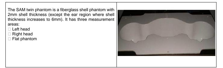
The bottom plate contains three pair of bolts for locking the device holder. The device holder positions are adjusted to the standard measurement positions in the three sections. A white cover is provided to tap the phantom during off-periods to prevent water evaporation and changes in the liquid parameters. On the phantom top, three reference markers are provided to identify the phantom position with respect to the robot.
