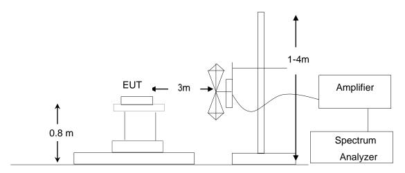
RADIATED EMISSION TEST SETUP ABOVE 1000MHz
