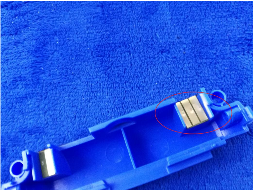
GSM/PCS/UMTS-FDD/LTE Antenna View
