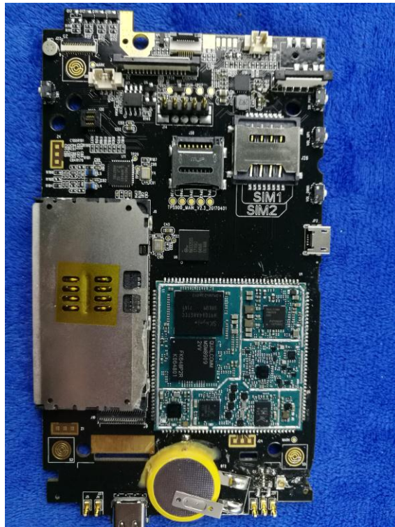
Mainboard without Shielding - Front View
