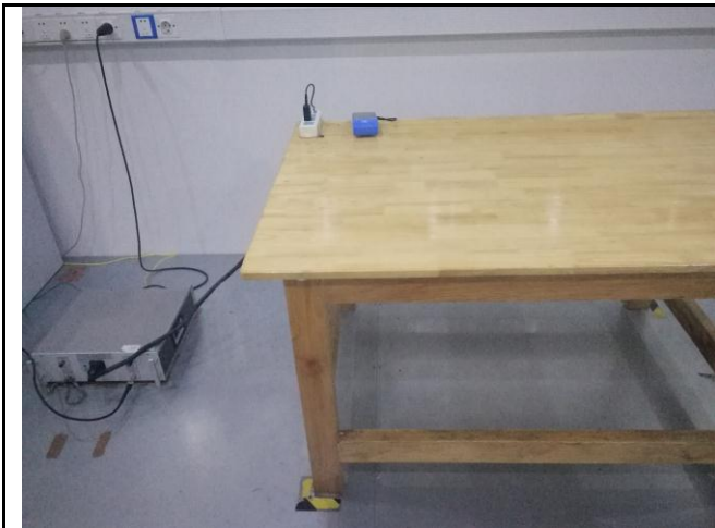
Conducted Emissions Test Setup Front View
