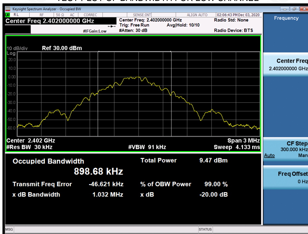
TEST PLOT OF BANDWIDTH FOR LOW CHANNEL
