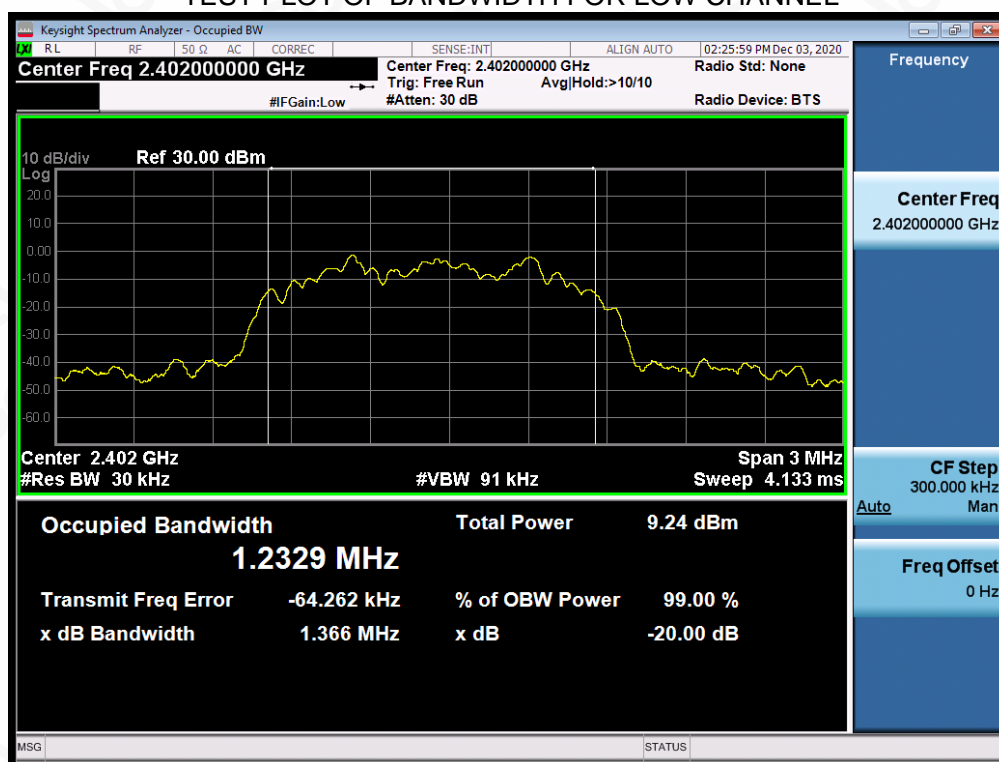
TEST PLOT OF BANDWIDTH FOR LOW CHANNEL
