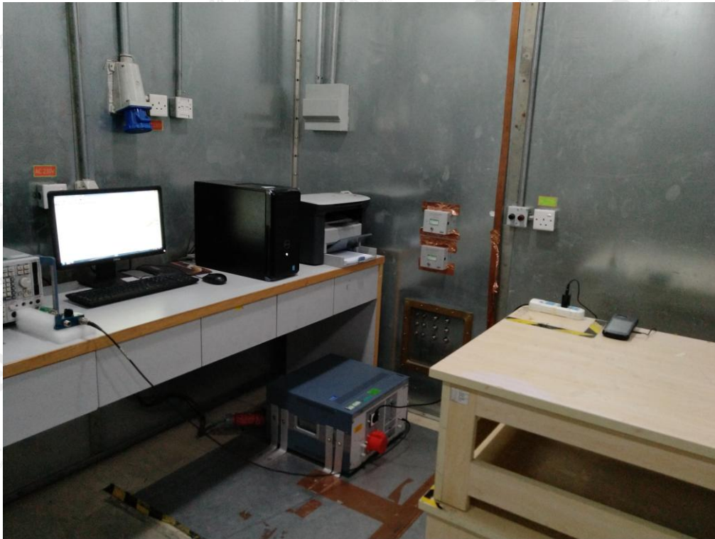
RADIATED EMISSION TEST SETUP
