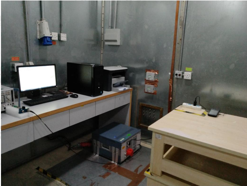
RADIATED EMISSION TEST SETUP
