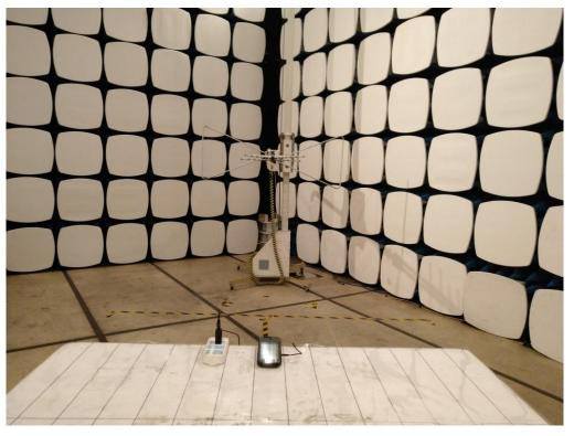
RADIATED EMISSION ABOVE 1G TEST SETUP
