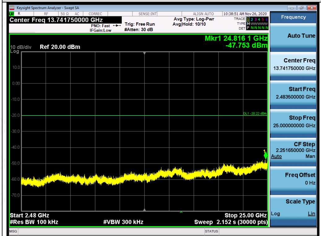
Test_Graph_802.11n20_ANT1_2412_MCS0_Higher Band Emissions
