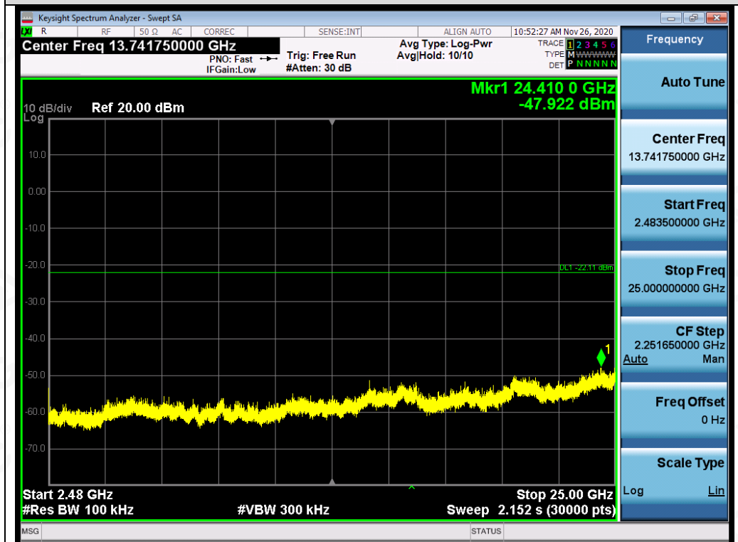
Test_Graph_802.11n40_ANT1_2437_MCS0_Higher Band Emissions
