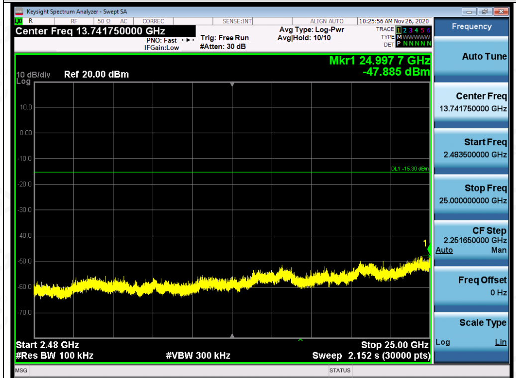
Test_Graph_802.11b_ANT1_2437_1Mbps_Higher Band Emissions
