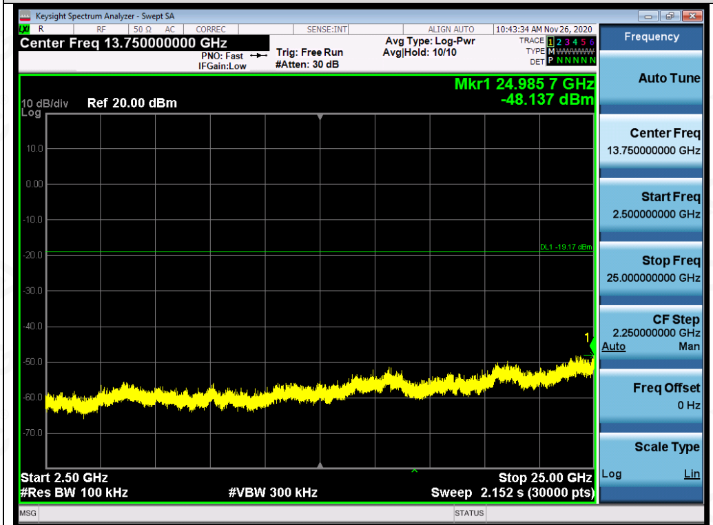
Test_Graph_802.11n20_ANT1_2462_MCS0_Higher Band Emissions
