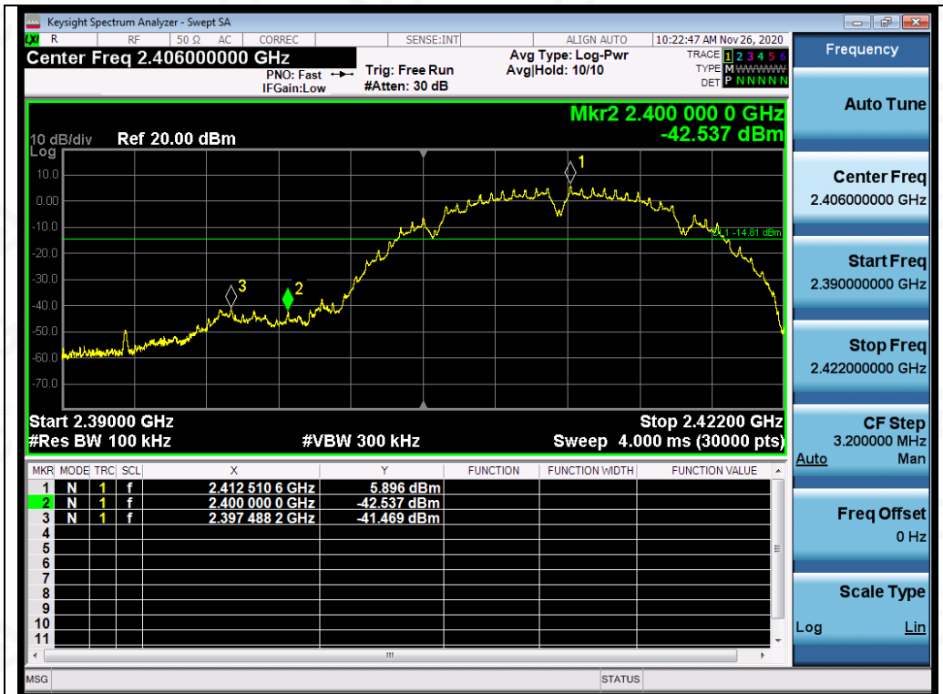
Test_Graph_802.11b_ANT1_2412_1Mbps_Lower Band Edge Emissions
