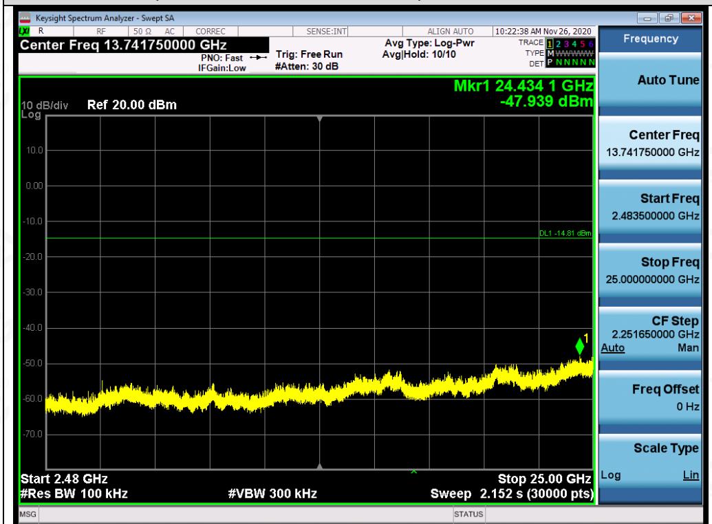
Test_Graph_802.11b_ANT1_2412_1Mbps_Higher Band Emissions
