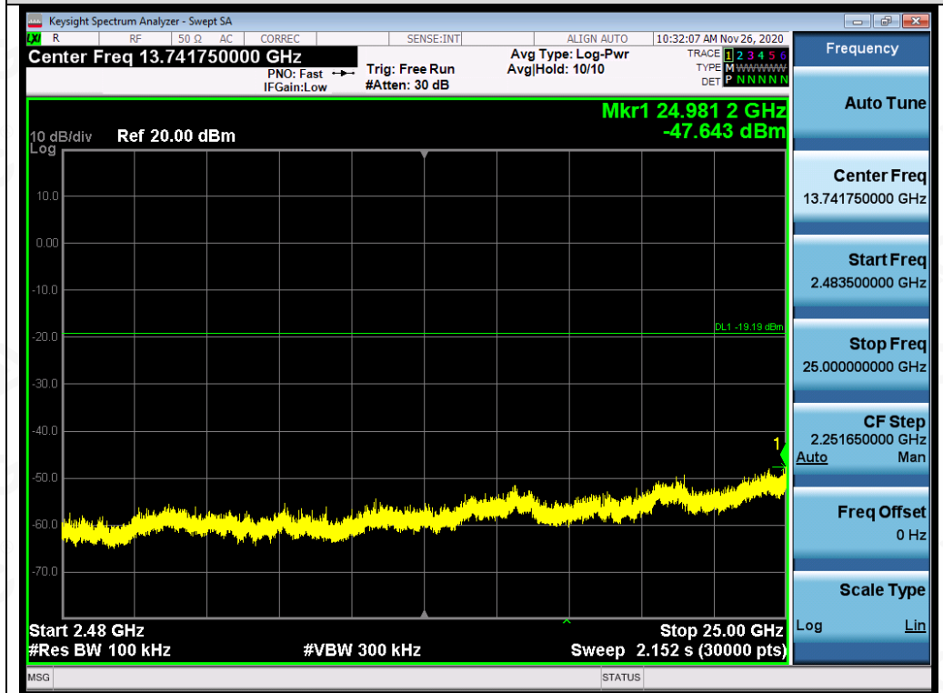
Test_Graph_802.11g_ANT1_2412_6Mbps_Higher Band Emissions
