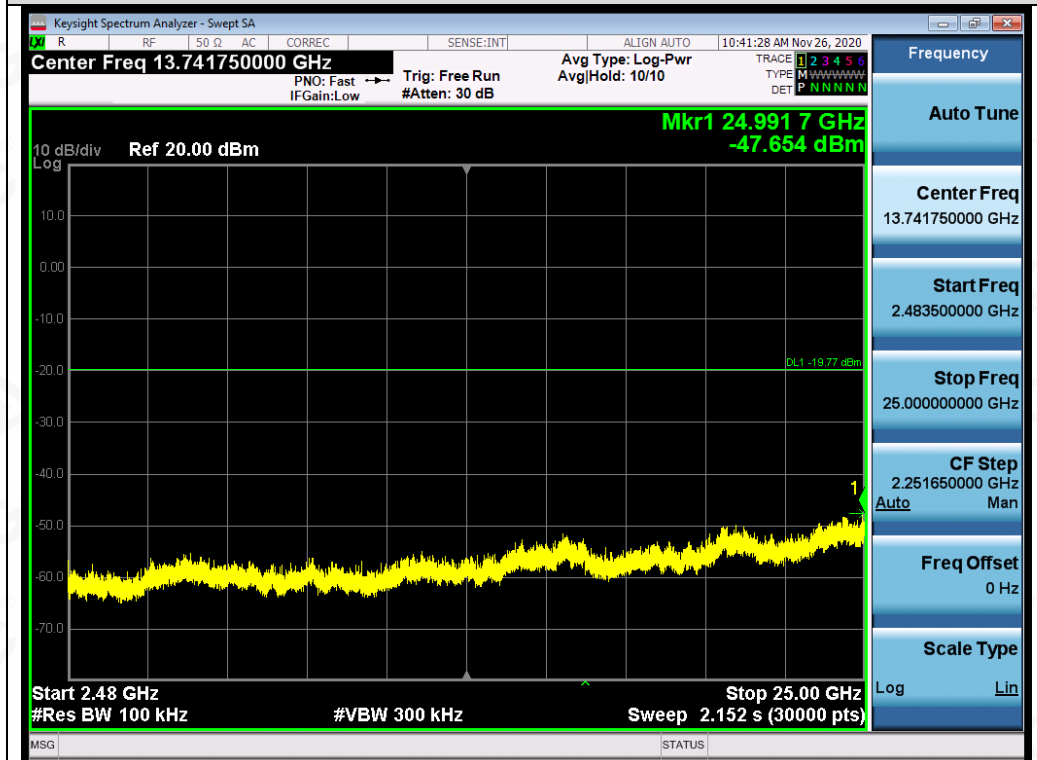
Test_Graph_802.11n20_ANT1_2437_MCS0_Higher Band Emissions
