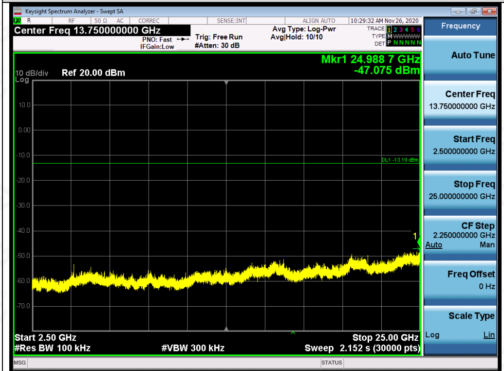
Test_Graph_802.11b_ANT1_2462_1Mbps_Higher Band Emissions
