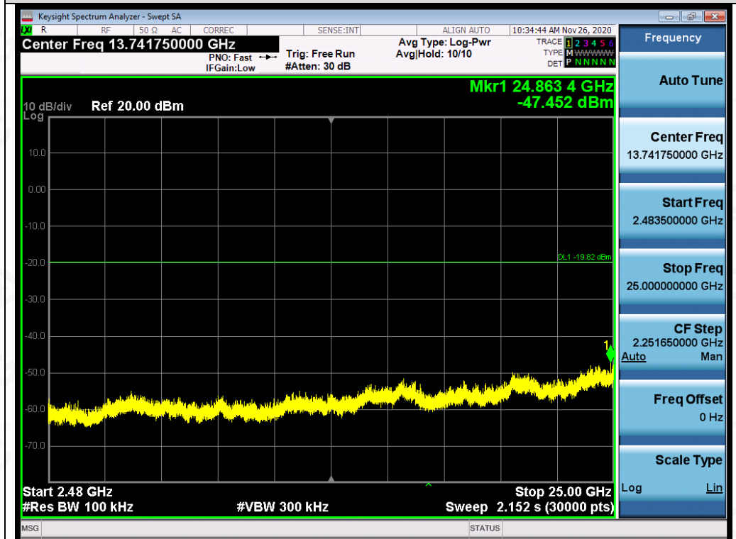
Test_Graph_802.11g_ANT1_2437_6Mbps_Higher Band Emissions
