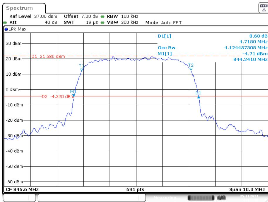
**26 dB Emissions &99% Occupied Bandwidth for HSUPA (BPSK) Mode, Low channel**
