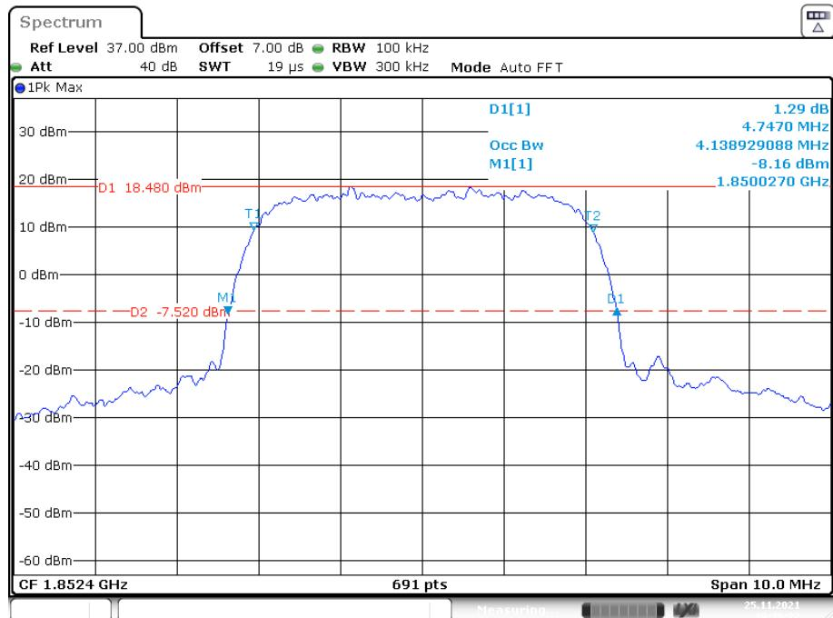
**26 dB Emissions & 99% Occupied Bandwidth for RMC (BPSK) Mode, Middle channel**
