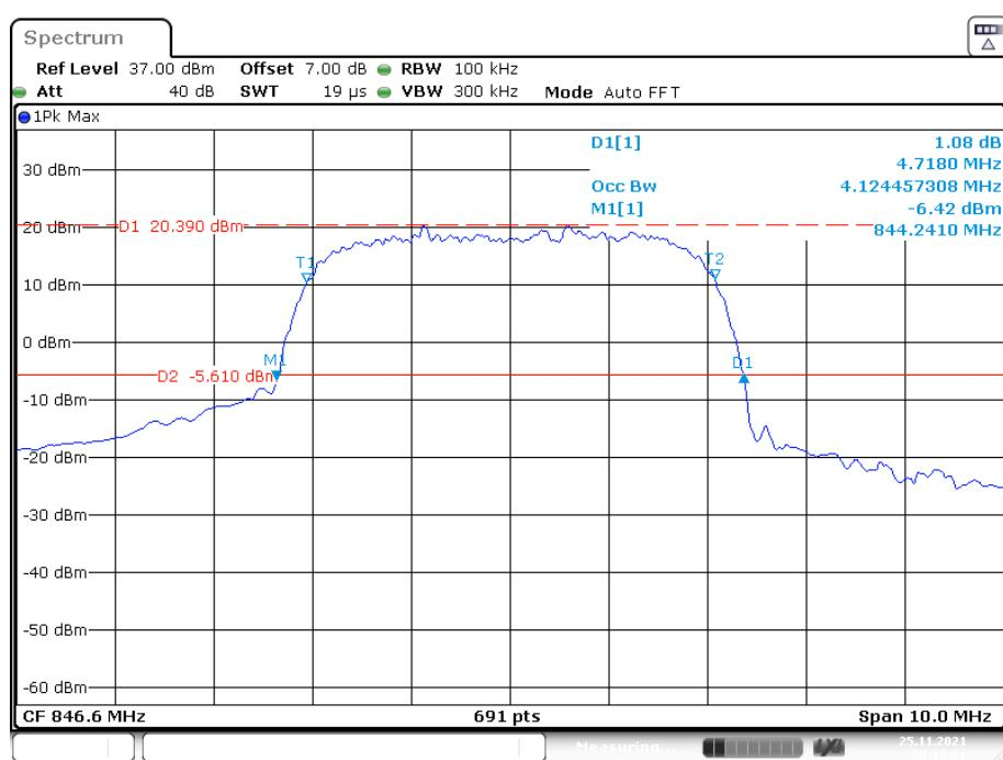
**26 dB Emissions &99% Occupied Bandwidth for HSDPA (16QAM) Mode, Low channel**
