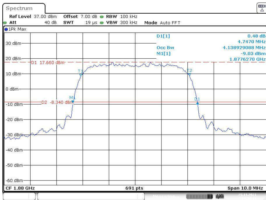
**26 dB Emissions &99% Occupied Bandwidth for HSDPA (16QAM) Mode, High channel**
