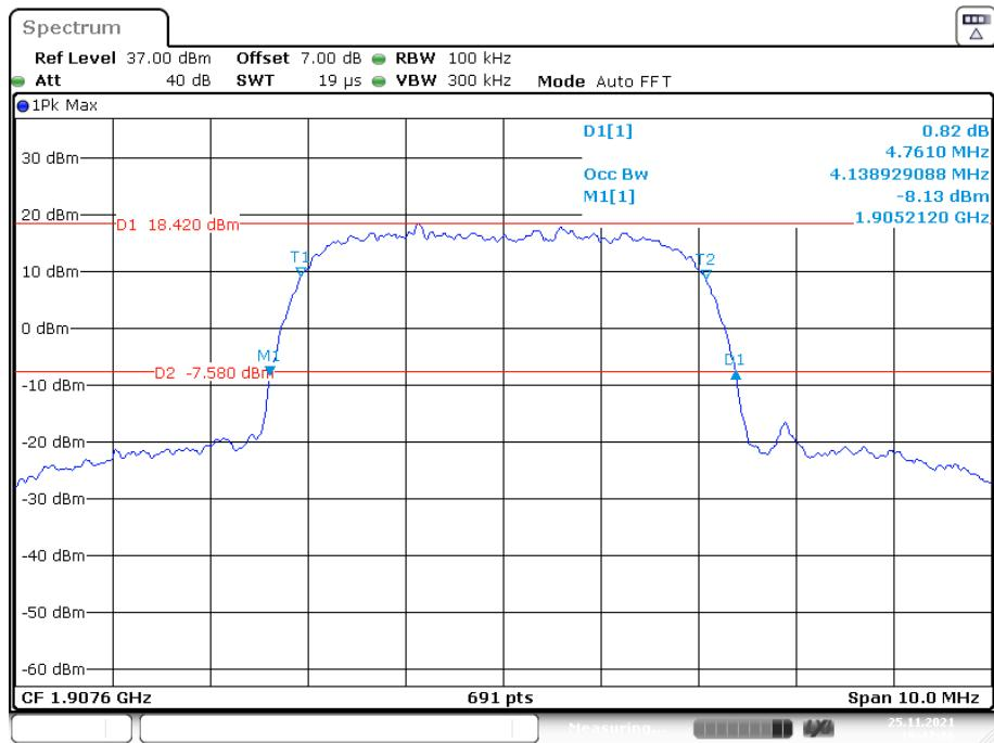
**26 dB Emissions &99% Occupied Bandwidth for HSUPA (BPSK) Mode, Low channel**
