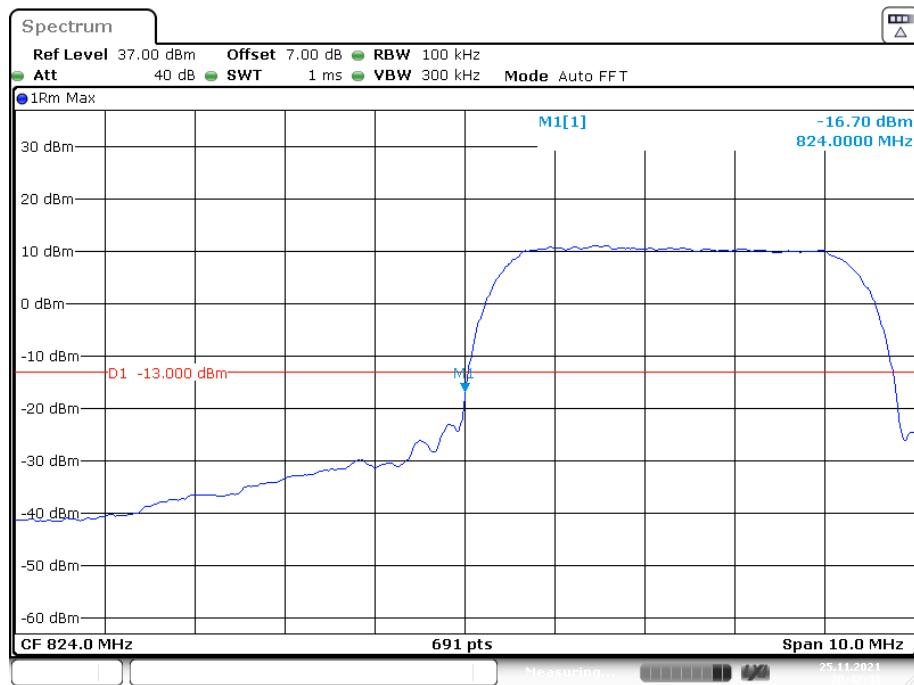
**Cellular Band, Right Band Edge for HSDPA (16QAM) Mode**
