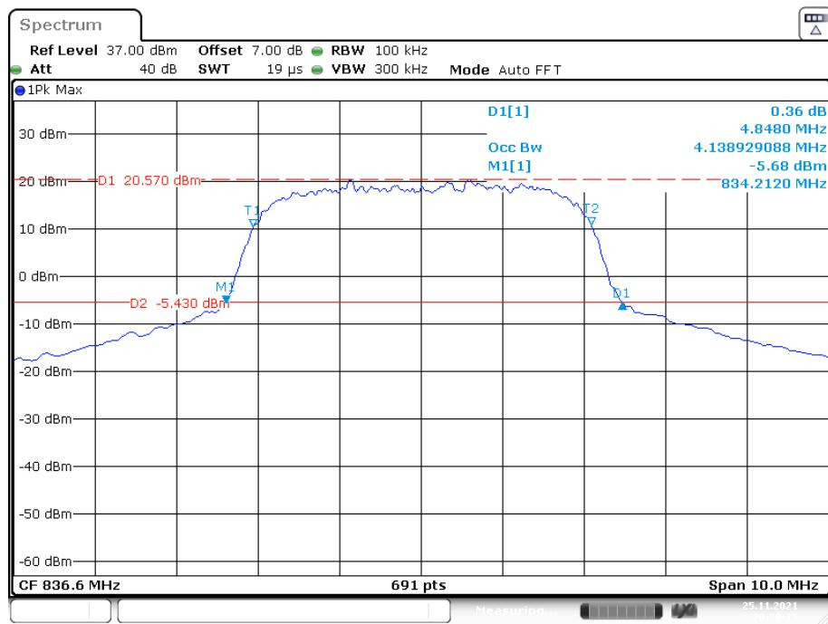
**26 dB Emissions &99% Occupied Bandwidth for HSUPA (BPSK) Mode, High channel**
