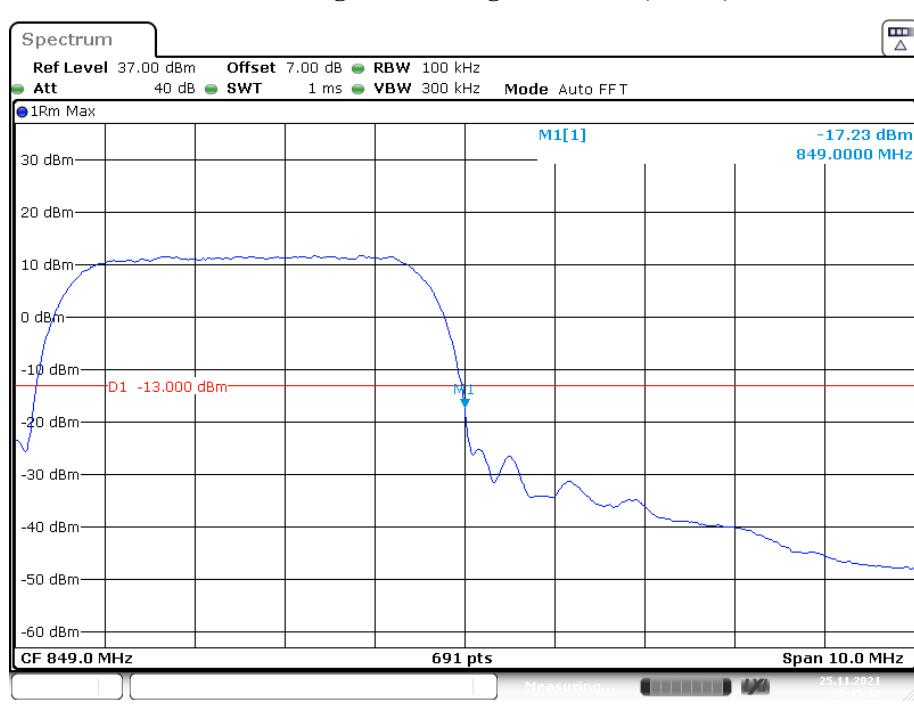
**Cellular Band, Left Band Edge for HSDPA(16QAM) Mode**
