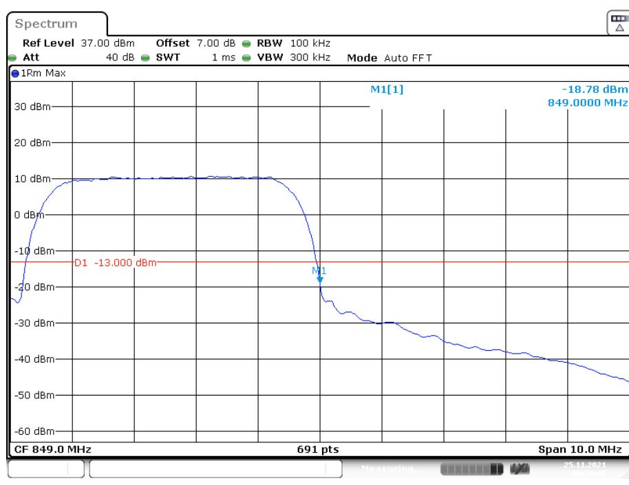
**Cellular Band, Left Band Edge for HSUPA (BPSK) Mode**
