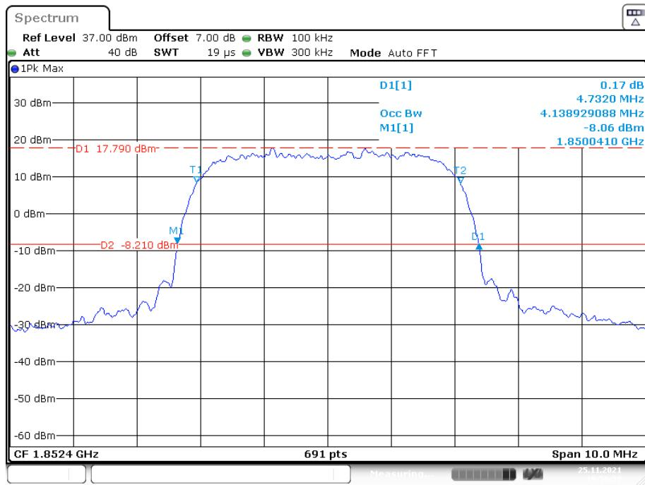
**26 dB Emissions &99% Occupied Bandwidth for HSDPA (16QAM) Mode, Middle channel**
