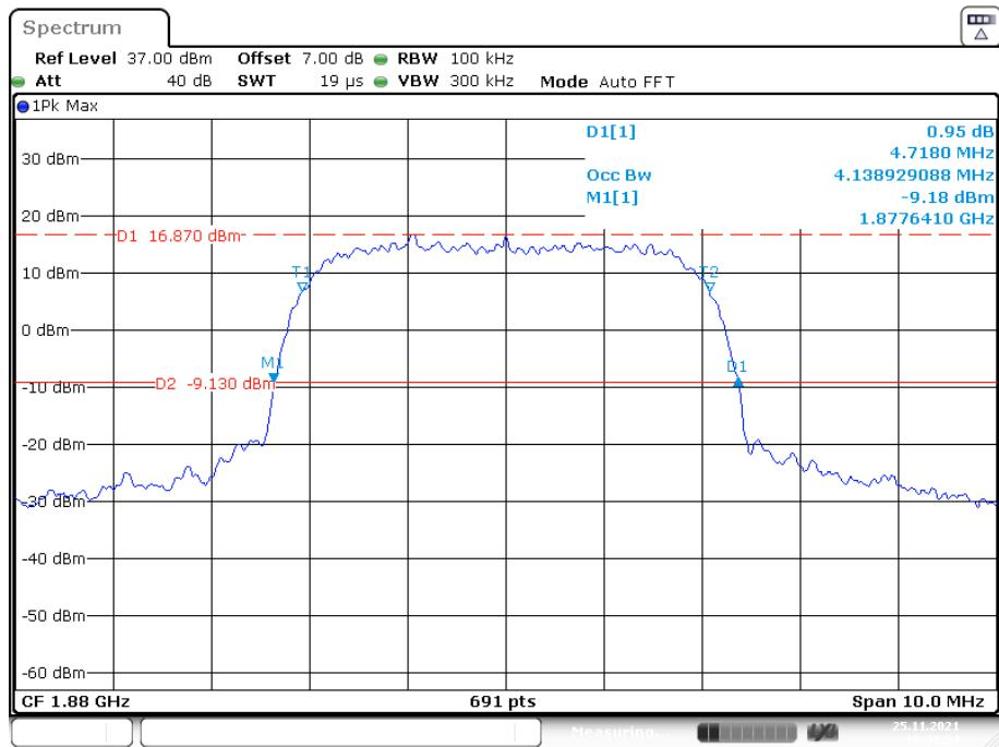
**26 dB Emissions &99% Occupied Bandwidth for HSUPA (BPSK) Mode, High channel**
