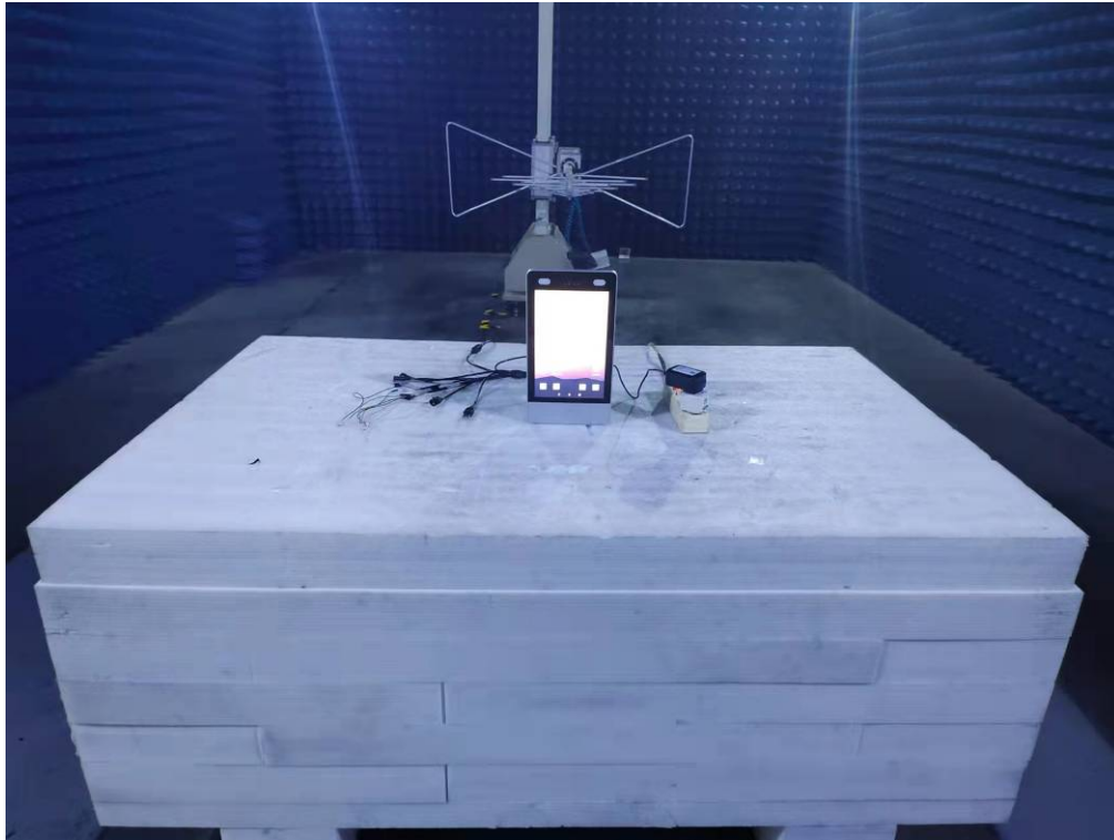
Photo of Radiated Emission Measurement (Above 1G)
