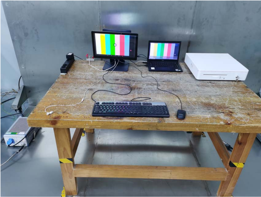
Conducted Emissions Side View
