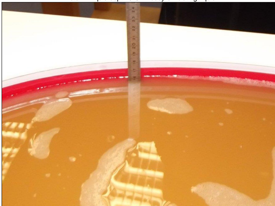
Photo 2: Liquid depth 5 GHz body simulating liquid
