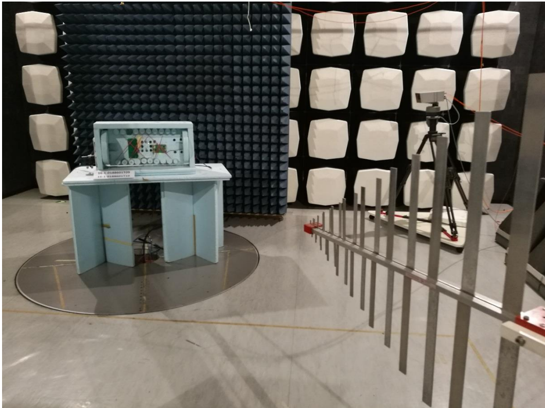
Photograph 3: Set Up 1-overall view-30 MHz-1 GHz
