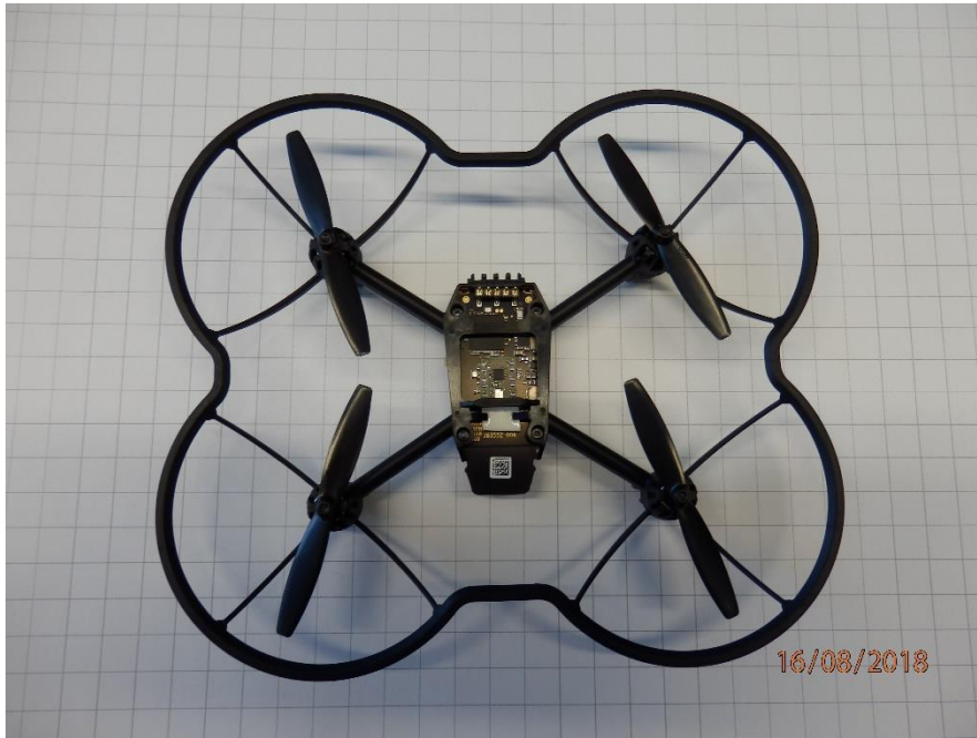
Figure 1: PCB Stack in Drone from top, grid 1cm x 1cm
