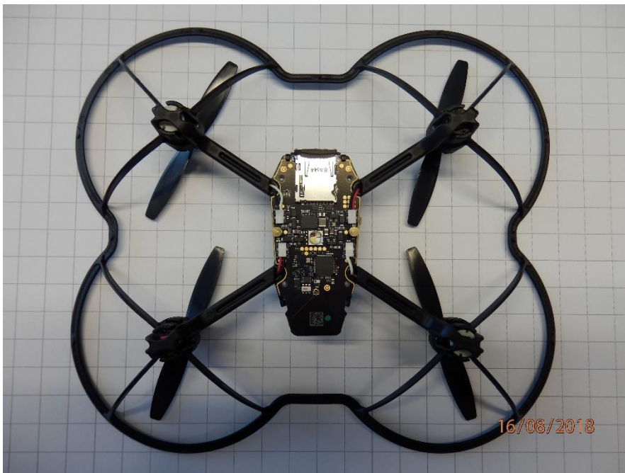
Figure 2: PCB Stack in Drone from bottom, grid 1cm x 1cm
