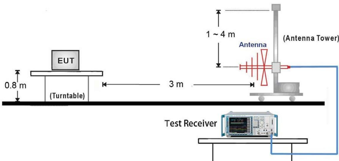
1GHz ~ 25GHz Test Setup:
