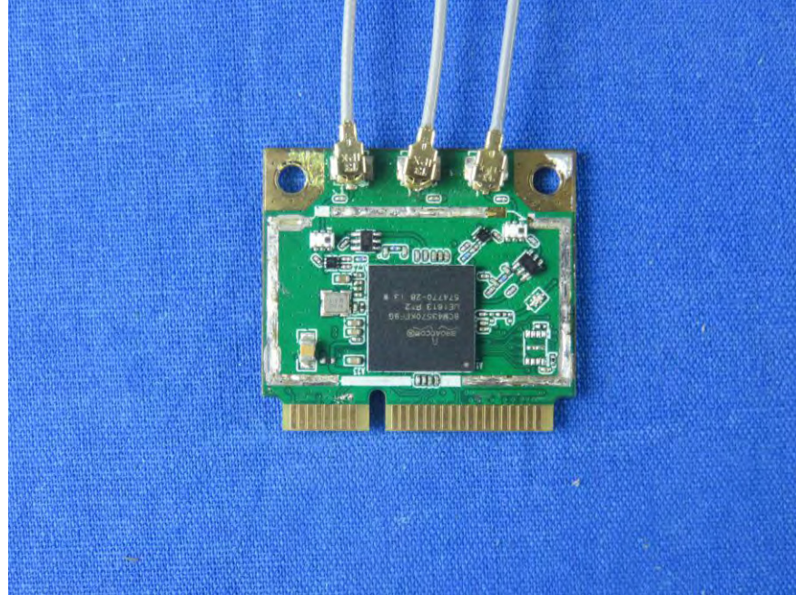
5. Figure PCB of the EUT-Front View
