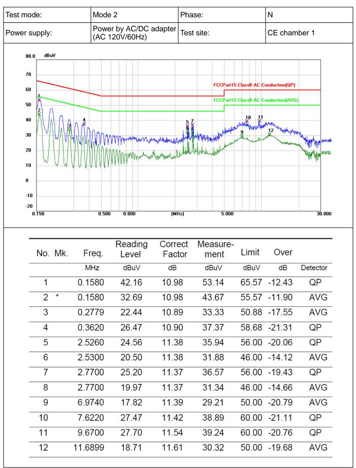
Note: EUT has two different voltage supports, reporting only the worst voltage mode.
