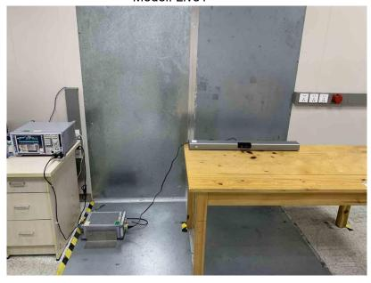
Radiated Spurious Emissions From 30MHz-1000MHz
