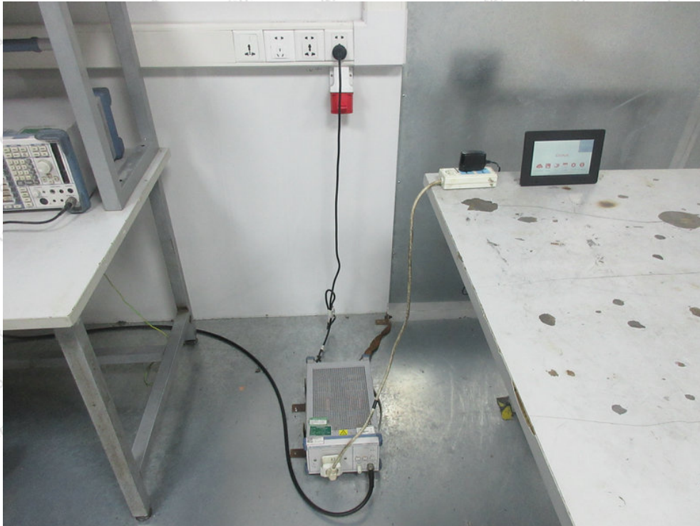
Photo of Power Line Conducted Emission Test
