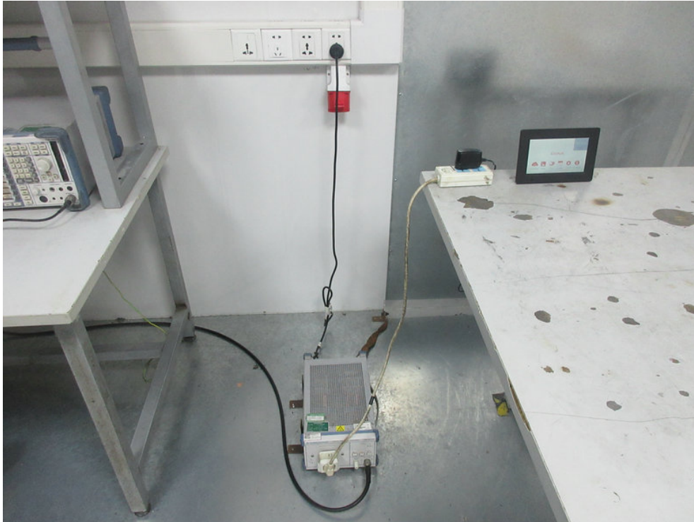
Photo of Conducted Emission Measurement
