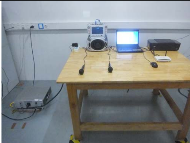
Conducted Emissions Test Setup – Front View
