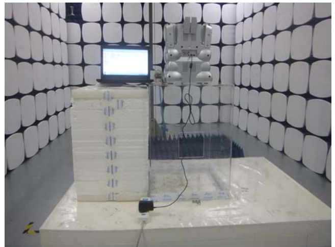
Radiated Spurious Emissions Test Above 1GHz
