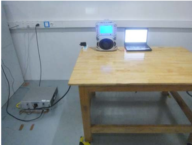
Conducted Emissions Test Setup – Front View
