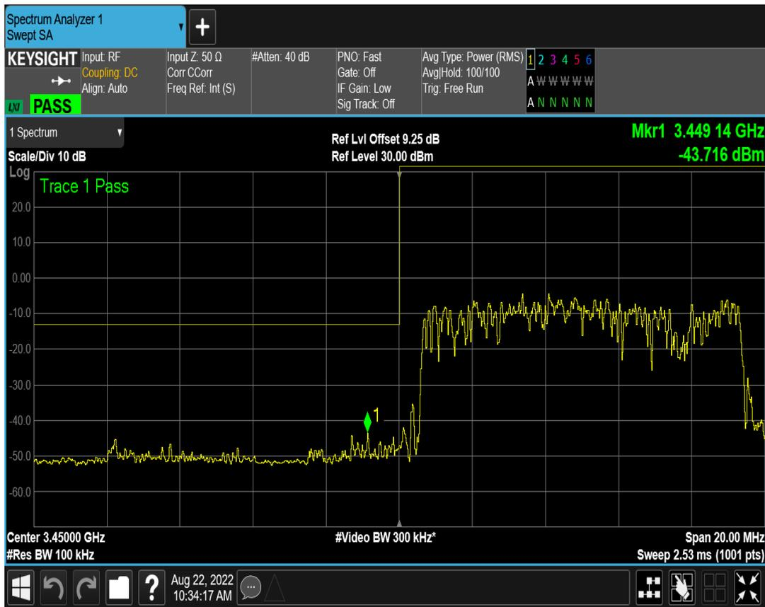
n77(3450-3550) SCS=30kHz DFT\_QPSK BW=10MHz Channel=630334 RB=1@0
