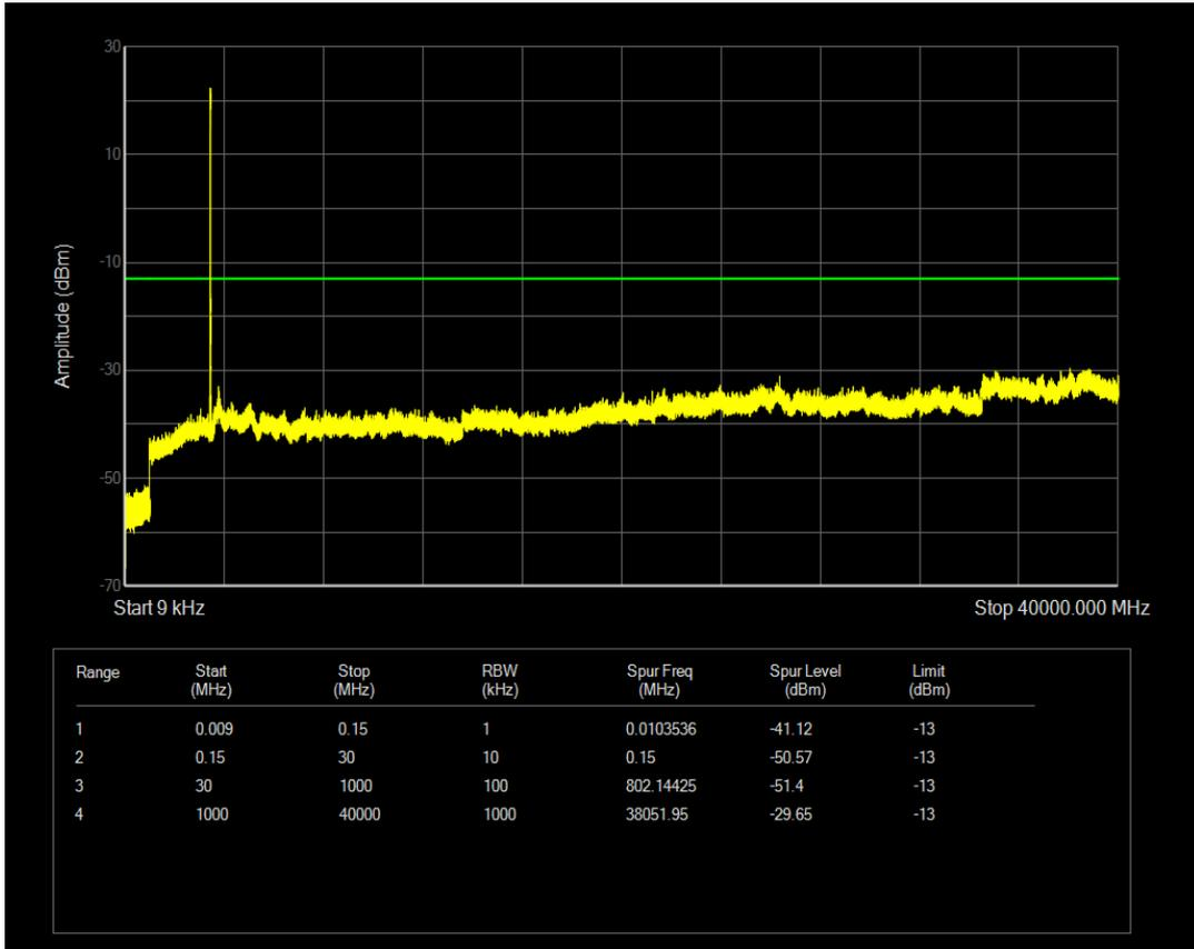
n77(3450-3550) SCS=30kHz DFT\_QPSK BW=10MHz Channel=630334 RB=1@0
