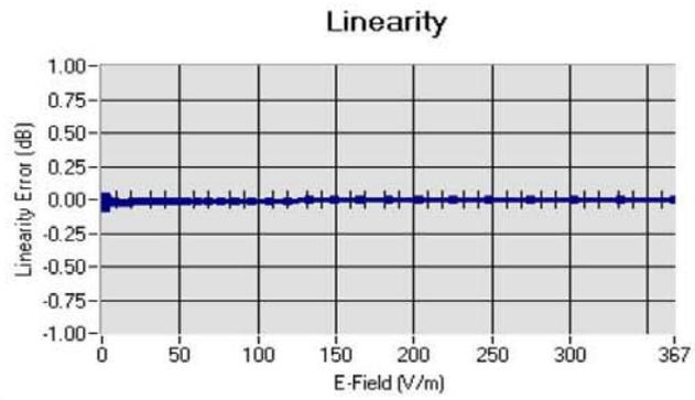
Linearity:  $\pm 1.50\%$  ( $\pm 0.07\text{dB}$ )5.3 SENSITIVITY IN LIQUID
