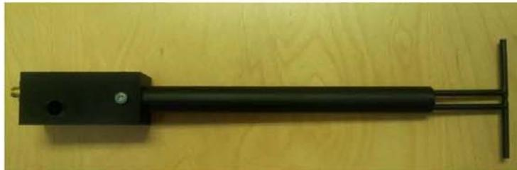
**Figure 1** – MVG COMOSAR Validation Dipole
