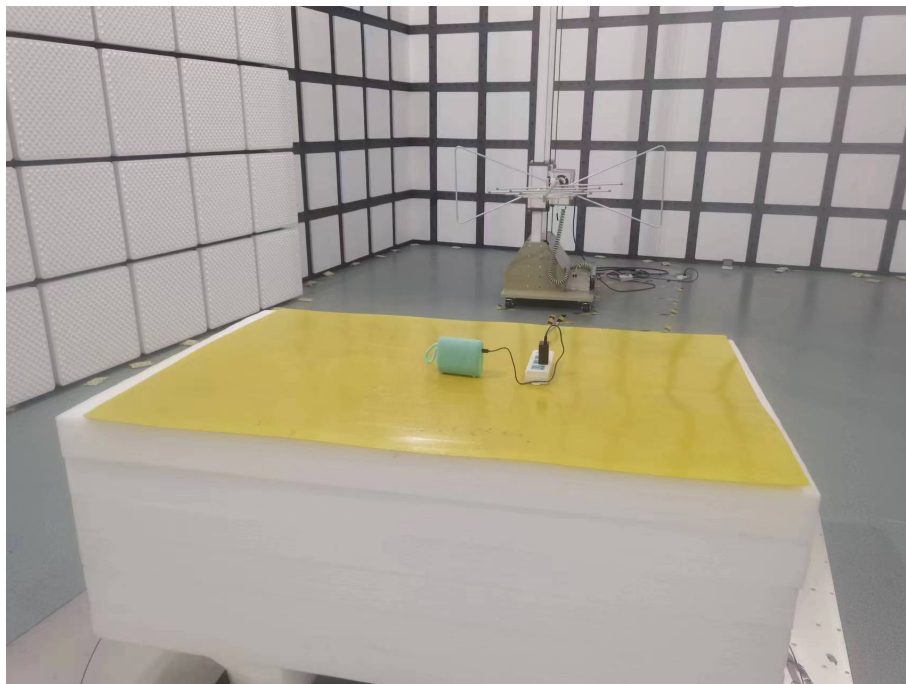
Photo of Radiated Emission Measurement (Above 1G)
