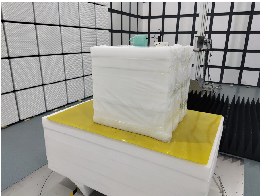
Photo of Radiated Emission Measurement (Above 1G)
