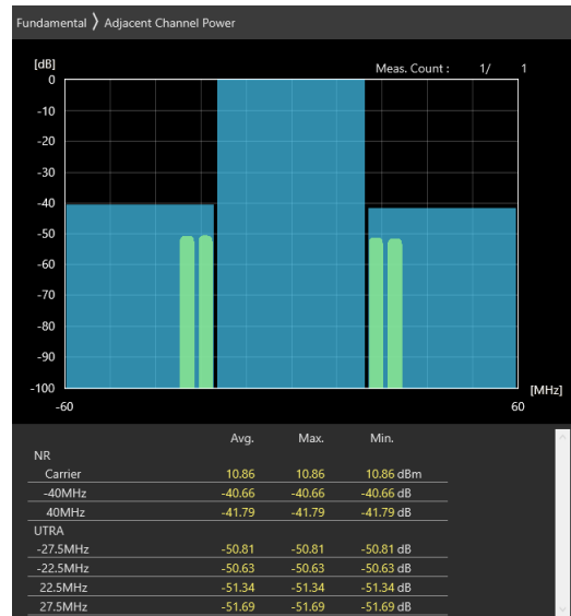
40MHz_15kHz_3570MHz_DFT-s-OFDM \pi/2 BPSK_RB108@54 -40.65 dB,-41.76 dB
