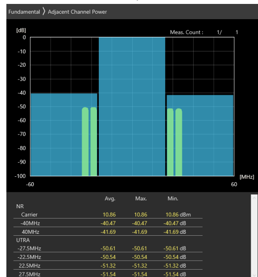
40MHz_15kHz_3680MHz_DFT-s-OFDM QPSK_RB108@54 -40.51 dB,-41.73 dB
