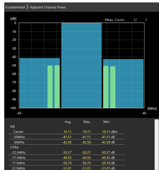
30MHz_30kHz_3685MHz_DFT-s-OFDM π/2 BPSK_RB75@0 -41.51 dB,-42.58 dB
