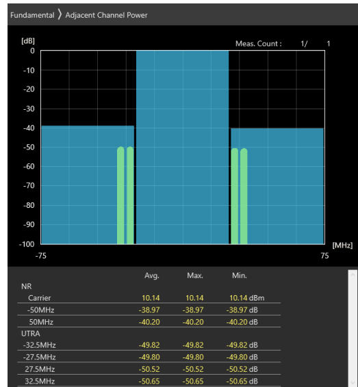
50MHz_15kHz_3575MHz_DFT-s-OFDM 16 QAM_RB135@67 -38.97 dB,-40.2 dB
