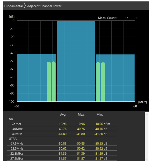
40MHz_30kHz_3570MHz_DFT-s-OFDM QPSK_RB50@25 -40.77 dB,-41.86 dB
