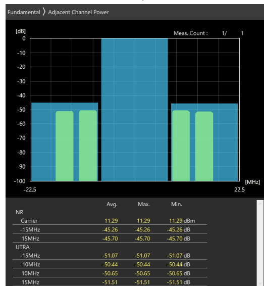
15MHz_15kHz_3557.5MHz_DFT-s-OFDM \pi/2 BPSK_RB36@18 -45.26 dB,-45.7 dB
