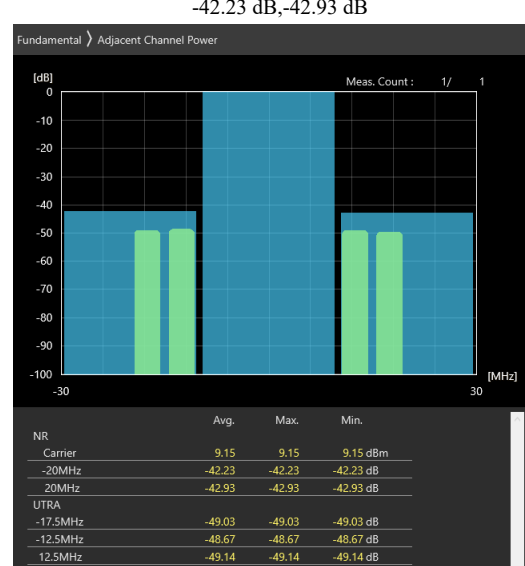
20MHz_15kHz_3690MHz_CP-OFDM 16 QAM_RB53@26 -42.23 dB,-42.93 dB
