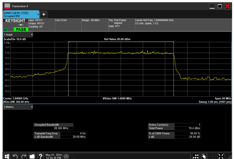
30MHz_15kHz_3840MHz_DFT-s-OFDM \pi/2 BPSK_RB160@0 28.585 MHz
