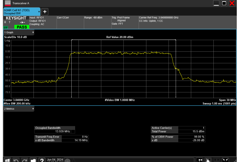
15MHz_15kHz_3840MHz_DFT-s-OFDM 64 QAM_RB75@0 13.939 MHz
