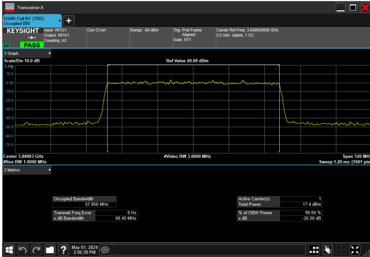
60MHz_30kHz_3840MHz_CP-OFDM 16 QAM_RB162@0 57.856 MHz
