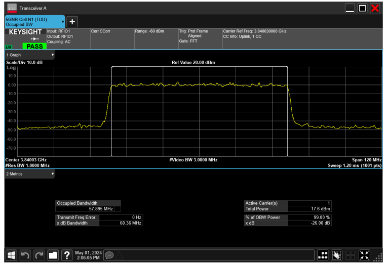
60MHz_30kHz_3840MHz_CP-OFDM QPSK_RB162@0 57.895 MHz
