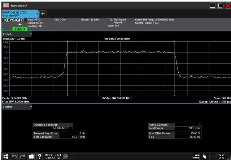
60MHz_30kHz_3840MHz_DFT-s-OFDM 16 QAM_RB162@0 57.684 MHz
