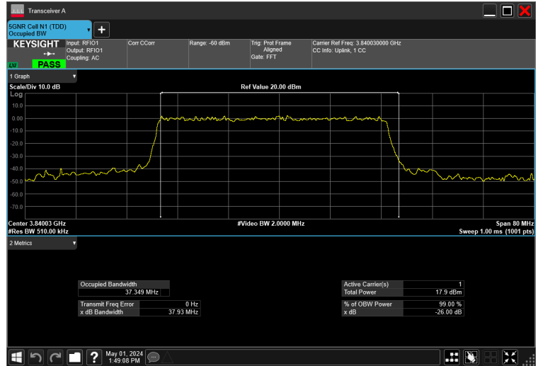
40MHz_30kHz_3840MHz_DFT-s-OFDM 16 QAM_RB100@0 37.349 MHz
