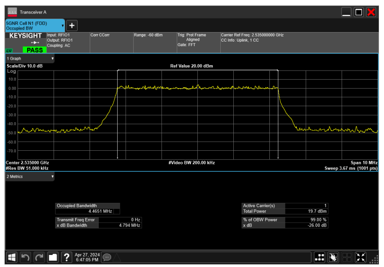
5MHz_15kHz_2535MHz_DFT-s-OFDM 16 QAM_RB25@0 4.465 MHz
