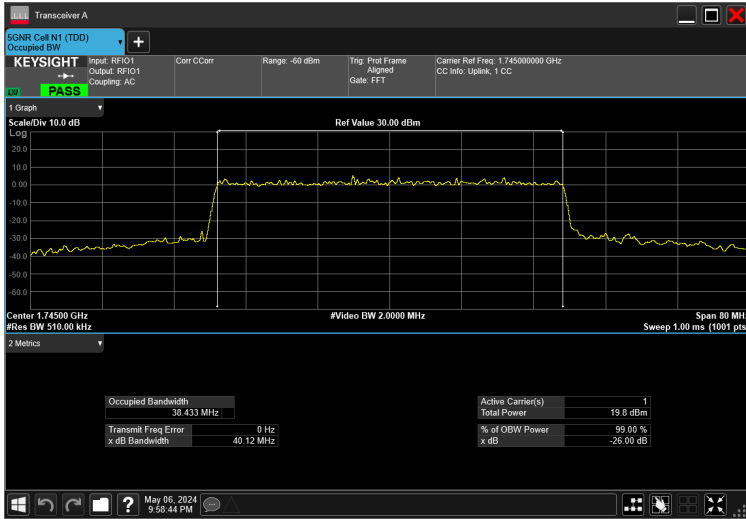
40MHz_15kHz_1745MHz_CP-OFDM 16 QAM_RB216@0 38.433 MHz
