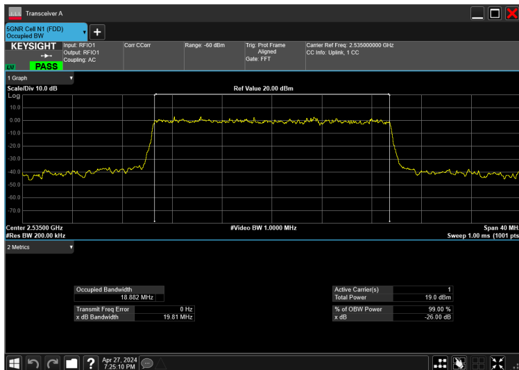
20MHz_15kHz_2535MHz_CP-OFDM 64 QAM_RB106@0 18.882 MHz
