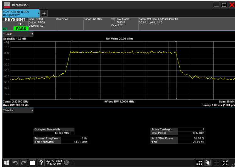
15MHz_15kHz_2535MHz_CP-OFDM QPSK_RB79@0 14.108 MHz
