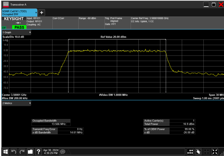
15MHz_30kHz_3500MHz_CP-OFDM 16 QAM_RB38@0 13.566 MHz
