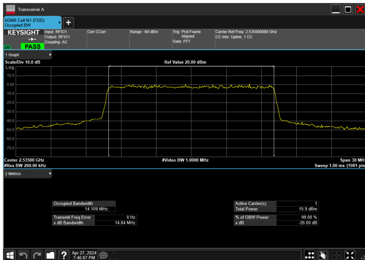
15MHz_15kHz_2535MHz_CP-OFDM 256 QAM_RB79@0 14.109 MHz
