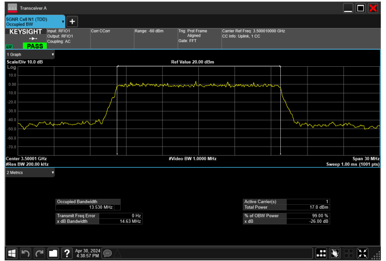
15MHz_30kHz_3500MHz_CP-OFDM QPSK_RB38@0 13.530 MHz
