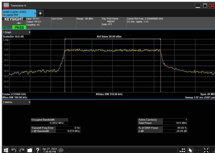
10MHz_15kHz_2535MHz_CP-OFDM 64 QAM_RB52@0 9.283 MHz
