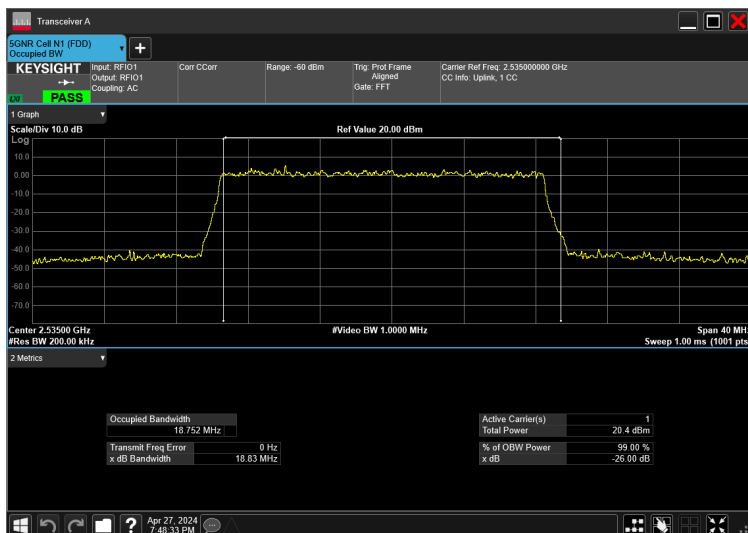
20MHz_15kHz_2535MHz_DFT-s-OFDM 16 QAM_RB100@0 18.752 MHz
