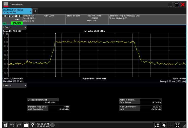
20MHz_15kHz_3500MHz_DFT-s-OFDM \pi/2 BPSK_RB100@0 18.805 MHz
