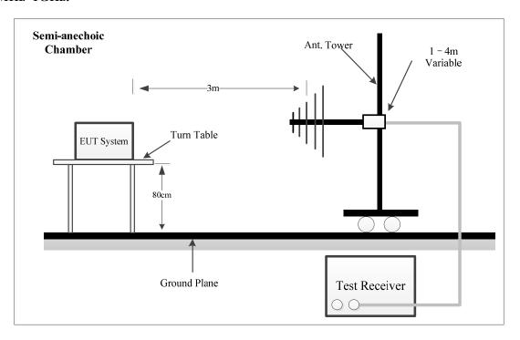
The radiated emission tests were performed in the 3-meter chamber test site, using the setup accordance with the ANSI C63.10-2013.
