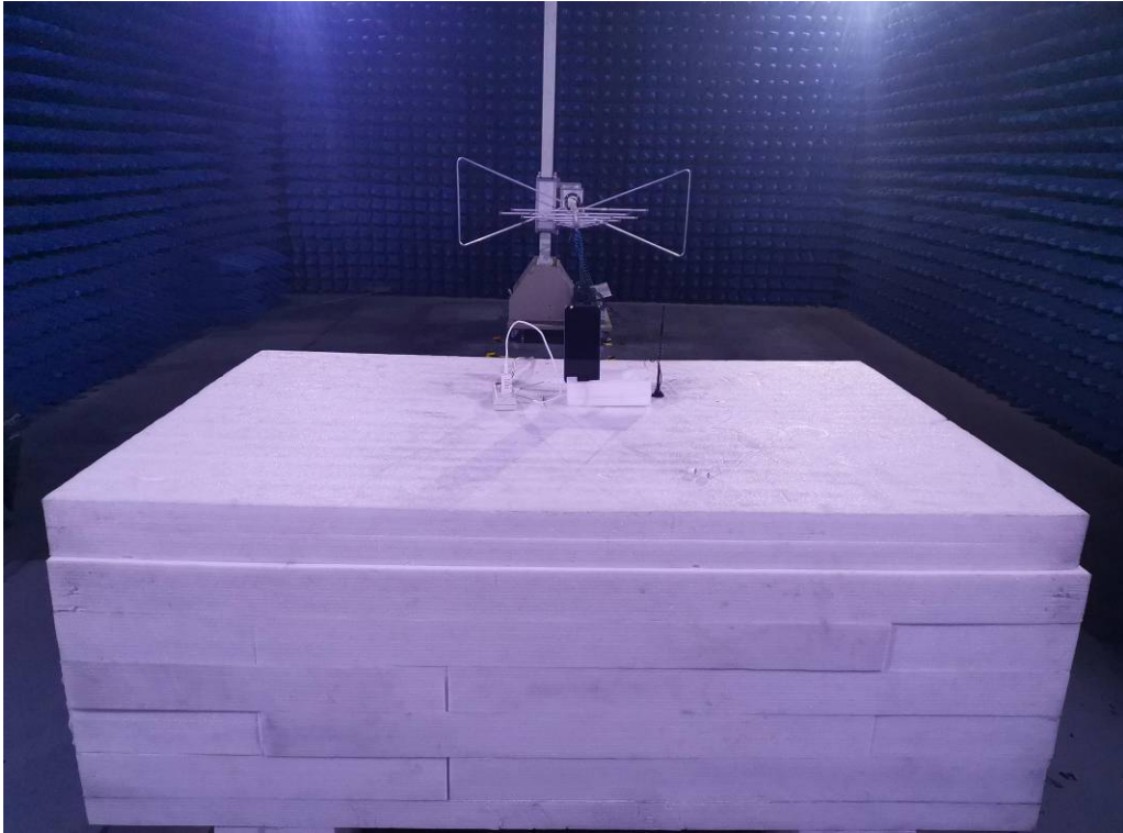
Photo of Radiated Emission Measurement (Above 1G)
