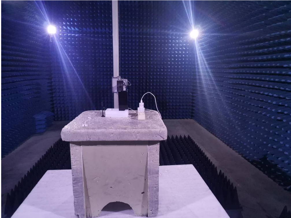
Photo of Radiated Emission Measurement (Above 1G)
