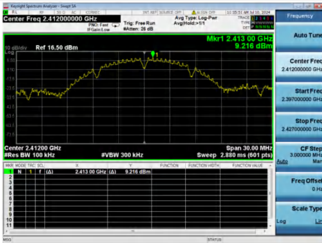
802.11b LOW CHANNEL, CARRIER LEVEL
