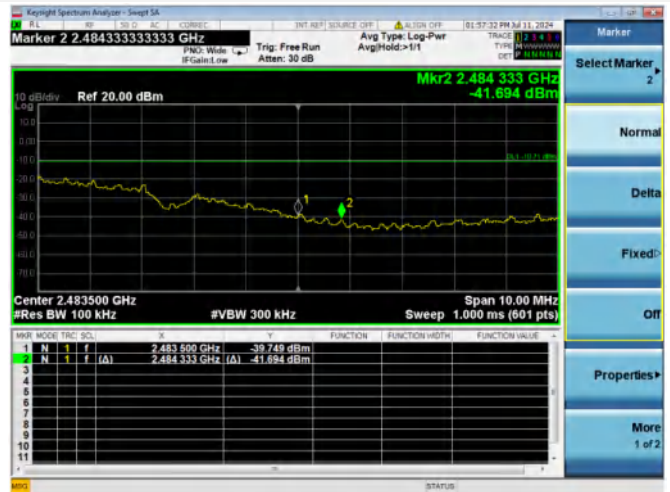
802.11b HIGH CHANNEL, BAND EDGE
