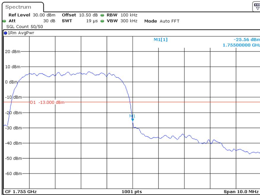
**AWS Band, Left Band Edge for HSUPA (QPSK) Mode**
