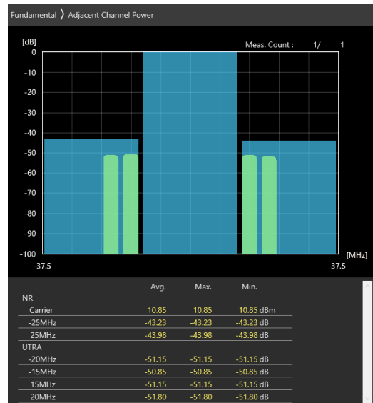
25MHz_30kHz_3562.5MHz_DFT-s-OFDM \pi/2 BPSK_RB32@16 -43.23 dB,-43.98 dB
