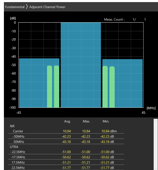
30MHz_15kHz_3565MHz_DFT-s-OFDM QPSK_RB80@40 -42.3 dB,-43.15 dB
