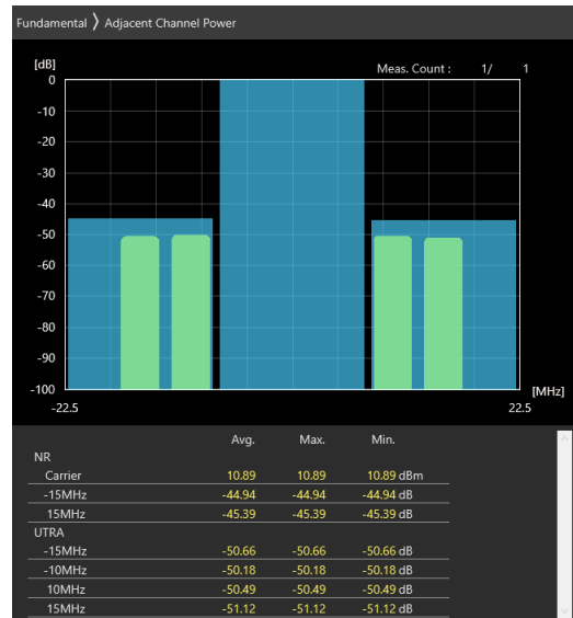
15MHz_15kHz_3557.5MHz_DFT-s-OFDM \pi/2 BPSK_RB36@18 -44.94 dB,-45.42 dB
