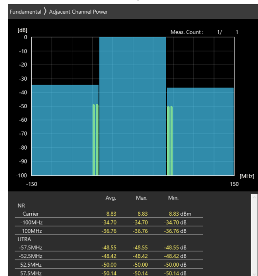
100MHz_30kHz_3650MHz_DFT-s-OFDM 16 QAM_RB270@0 -34.69 dB,-36.77 dB
