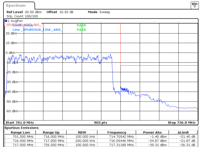
15MHz_15kHz_708.5MHz_DFT-s-OFDM QPSK_RB75@0 -34.87 dBm
