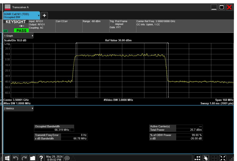
70MHz_30kHz_3500MHz_DFT-s-OFDM π/2 BPSK_RB180@0
