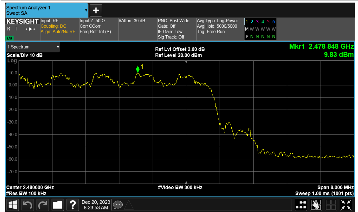
Band Edge(Hopping) NVNT 3-DH1 2480MHz Ant8 Hopping Emission
