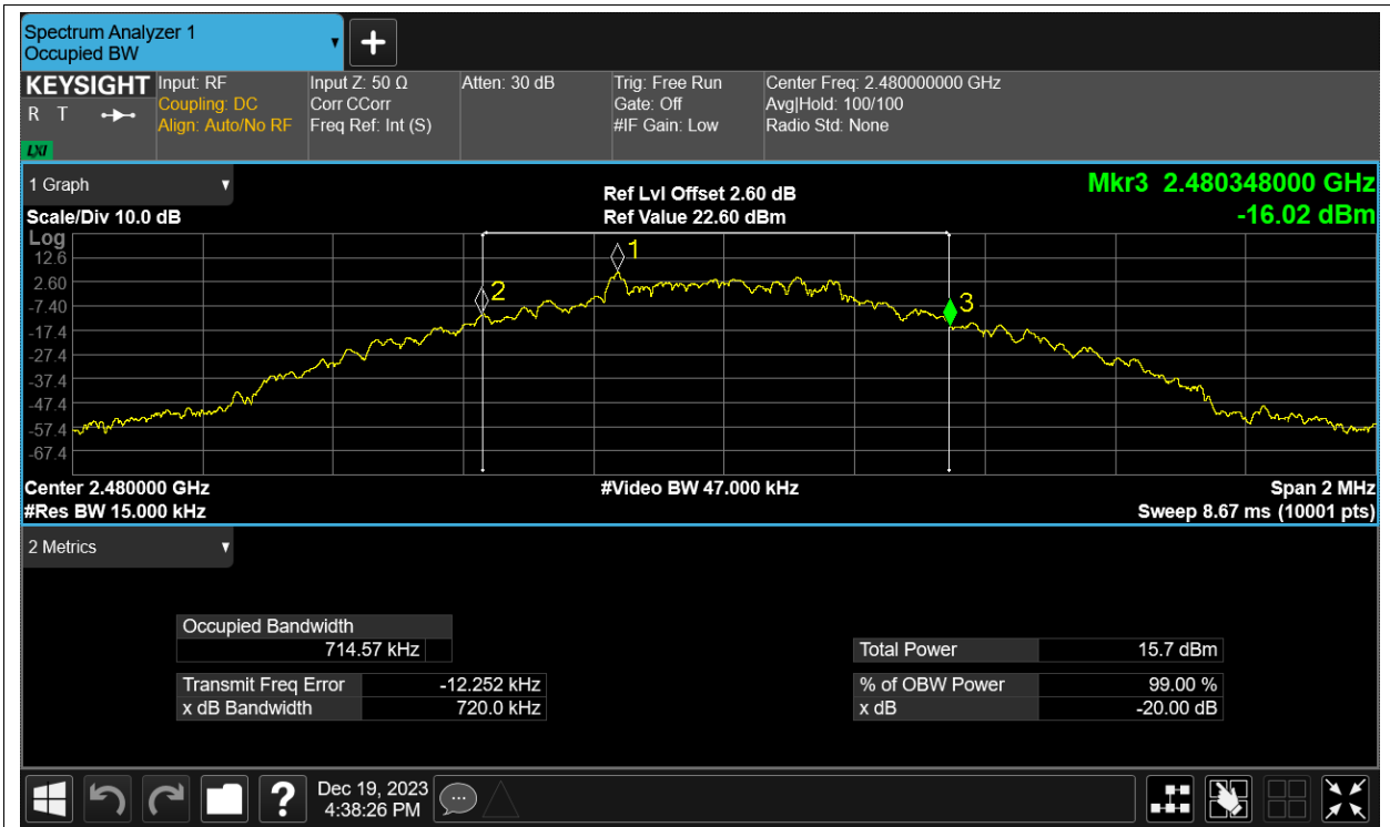
-20dB Bandwidth NVNT 2-DH1 2402MHz Ant8
