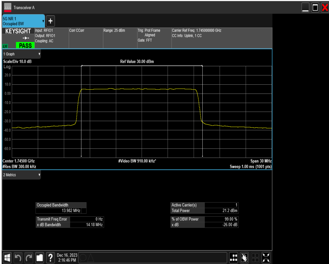
n66 SCS=15kHz DFT_QAM64 BW=15MHz Channel=349000 RB=75@0
