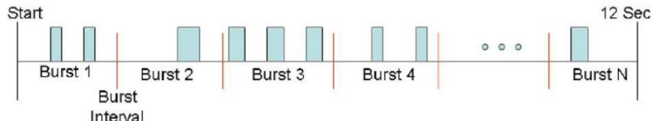
**Table D.7: Frequency Hopping Radar Test Waveform**
