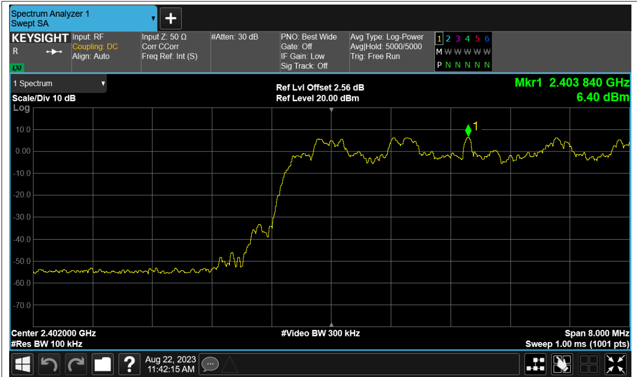
Band Edge(Hopping) NVNT 2-DH1 2402MHz Ant12 Hopping Emission
