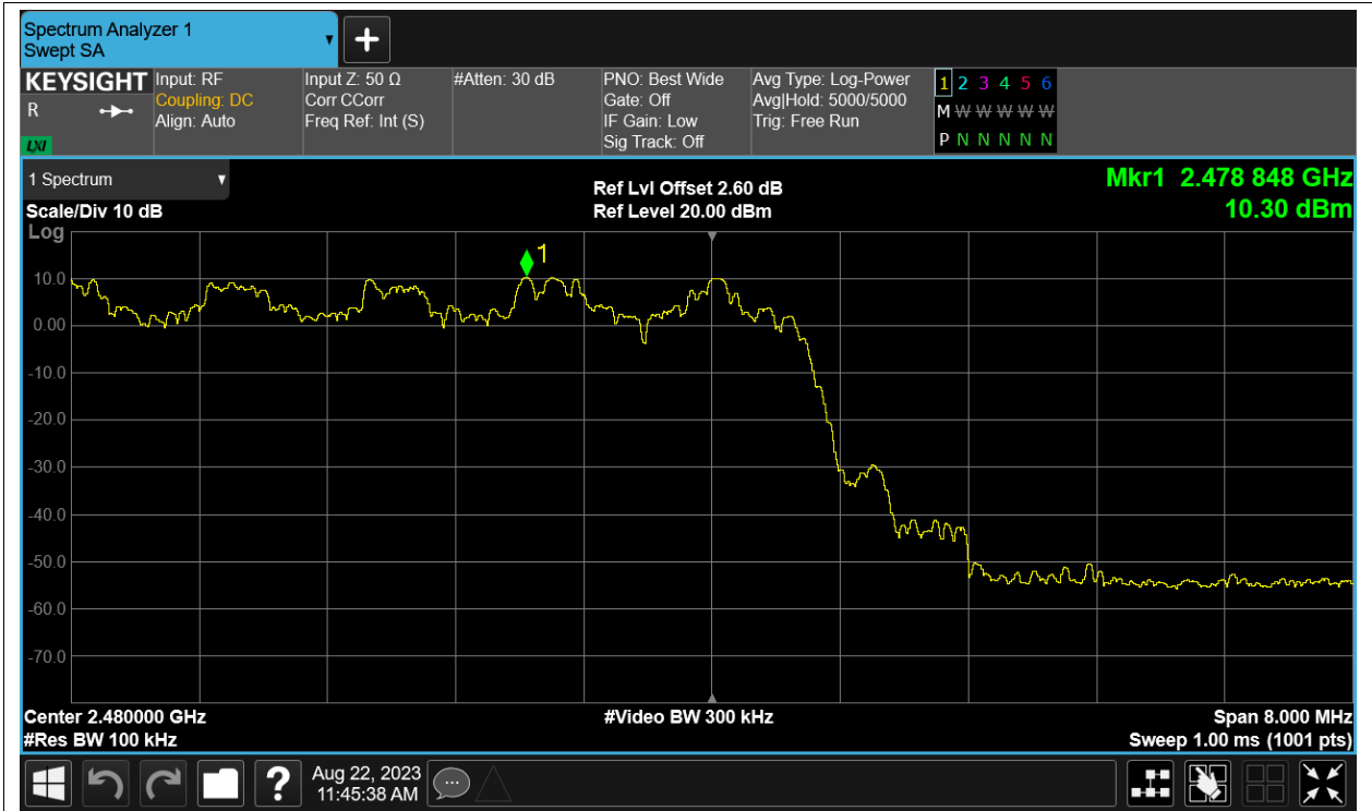
Band Edge(Hopping) NVNT 2-DH1 2480MHz Ant12 Hopping Emission
