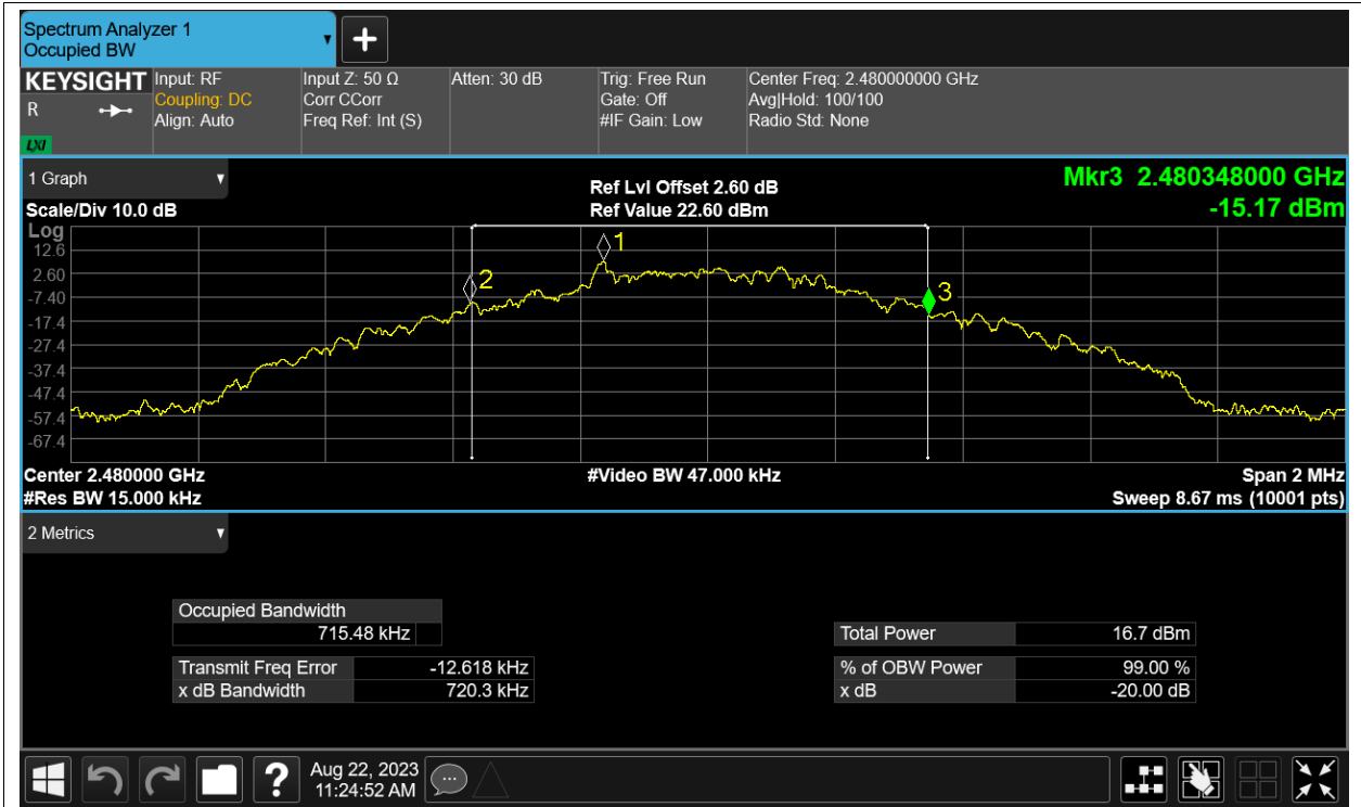
-20dB Bandwidth NVNT 2-DH1 2402MHz Ant12
