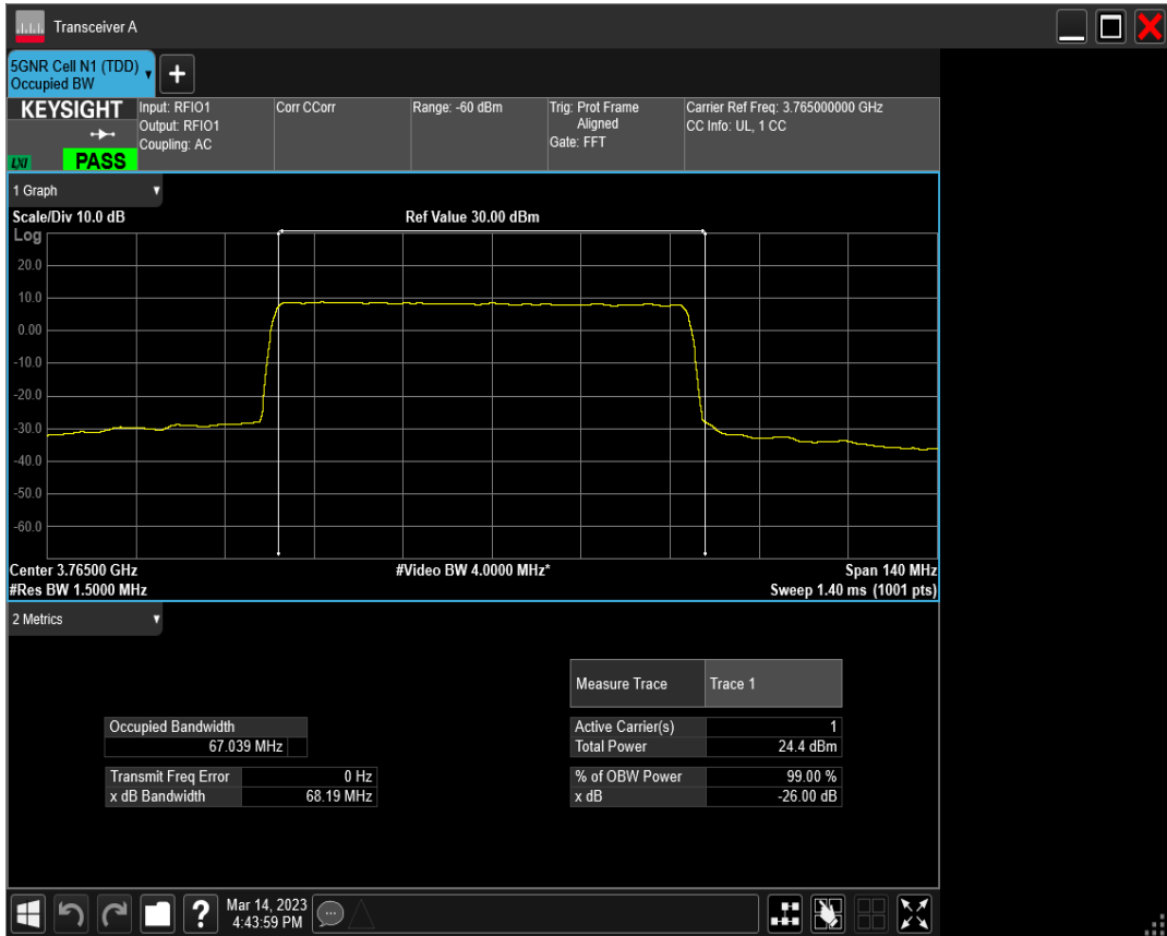
n78(3700-3800) SCS=30kHz CP_QPSK BW=70MHz Channel=651000 RB=189@0
