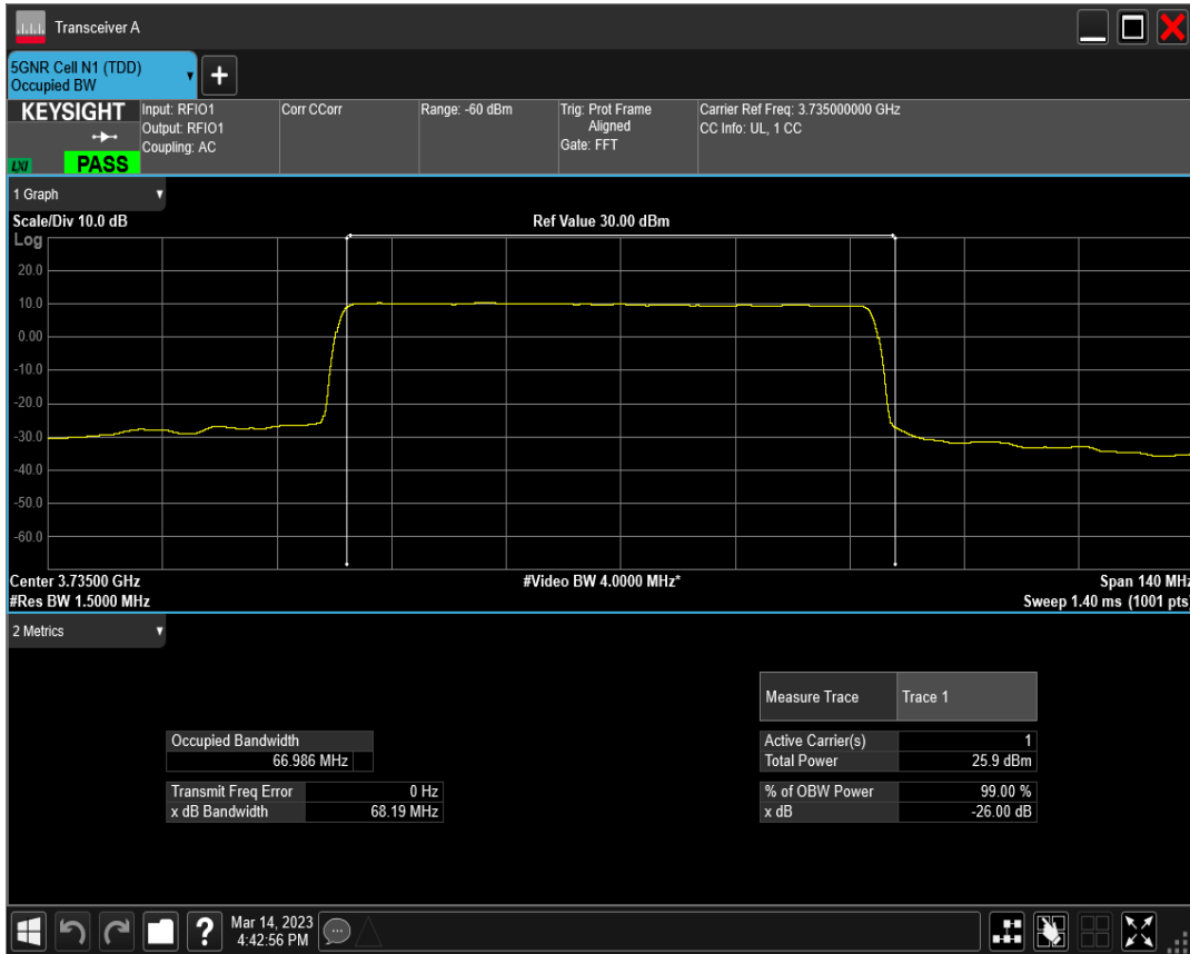
n78(3700-3800) SCS=30kHz DFT_QAM16 BW=70MHz Channel=649000 RB=180@0
