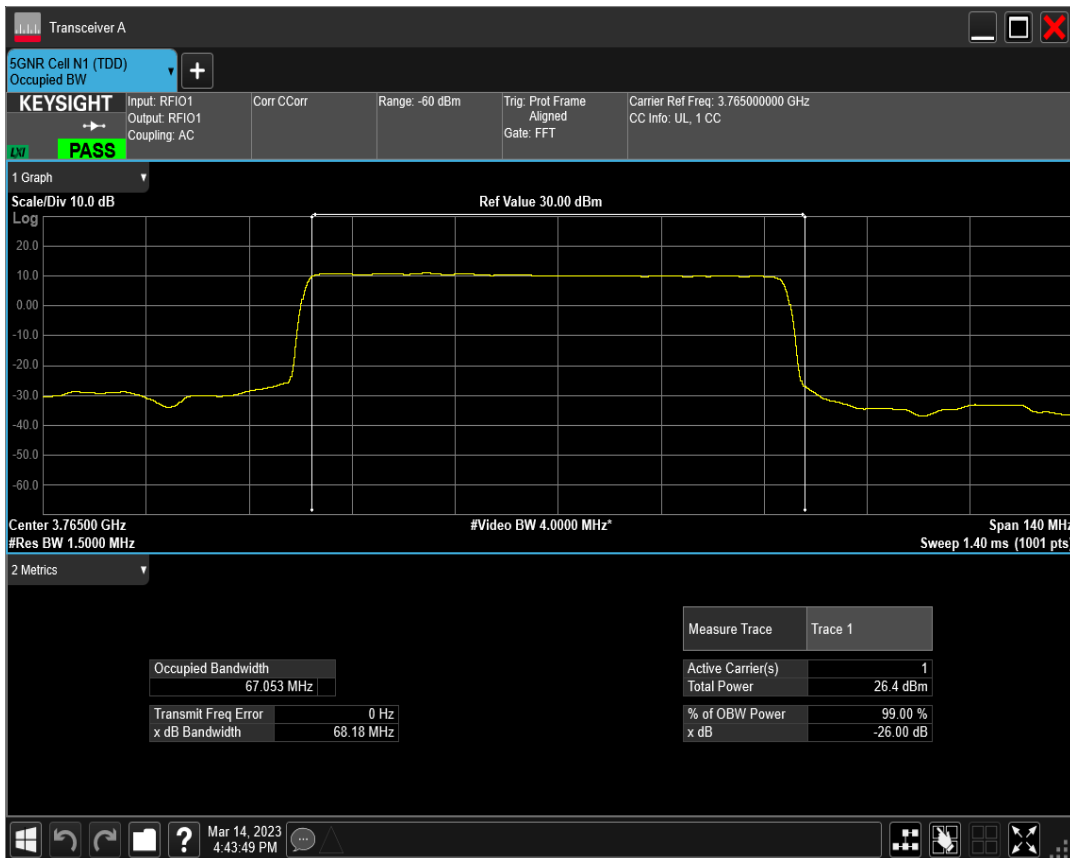
n78(3700-3800) SCS=30kHz DFT_QPSK BW=70MHz Channel=651000 RB=180@0
