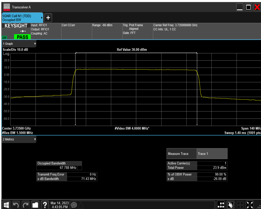
n78(3700-3800) SCS=30kHz DFT_BPSK BW=70MHz Channel=650000 RB=180@0
