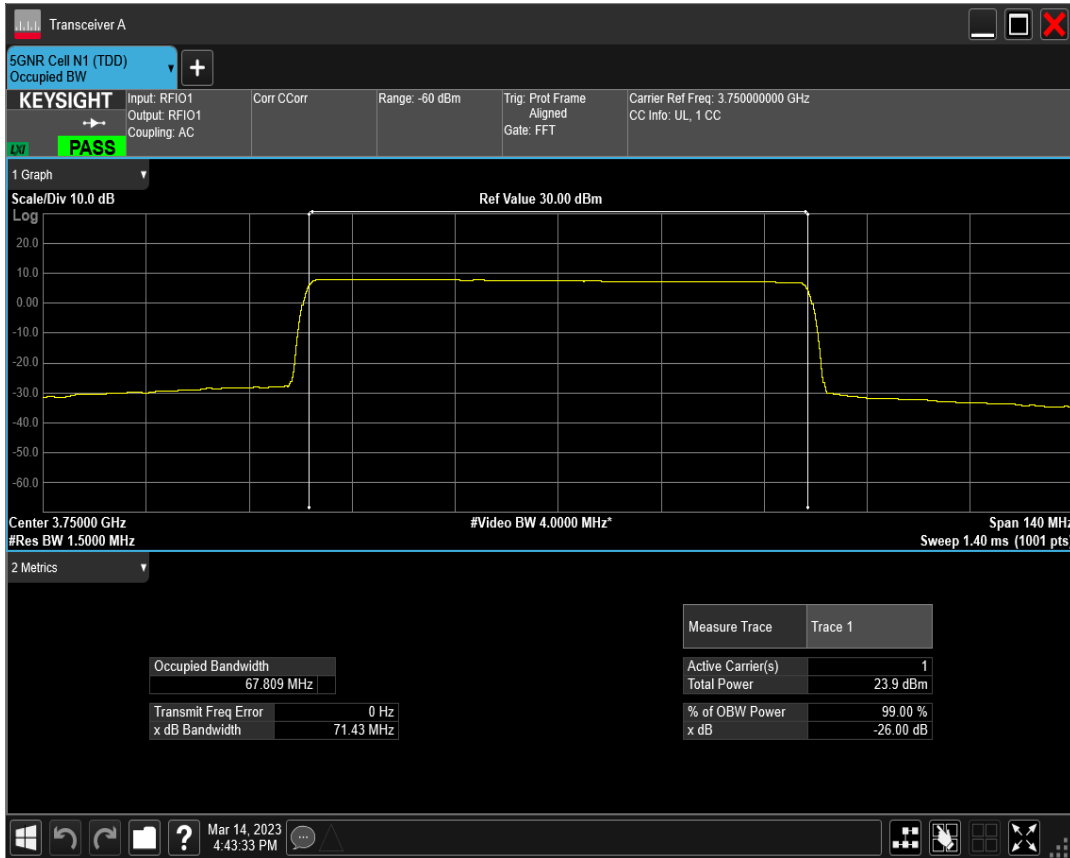
n78(3700-3800) SCS=30kHz DFT_BPSK BW=70MHz Channel=651000 RB=180@0
