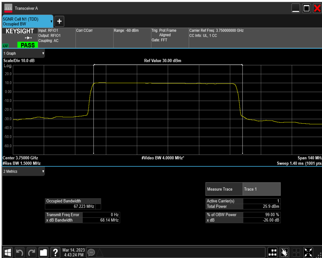
n78(3700-3800) SCS=30kHz DFT_QAM16 BW=70MHz Channel=650000 RB=180@0
