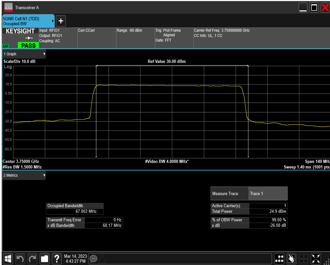
n78(3700-3800) SCS=30kHz DFT_QAM64 BW=70MHz Channel=650000 RB=180@0
