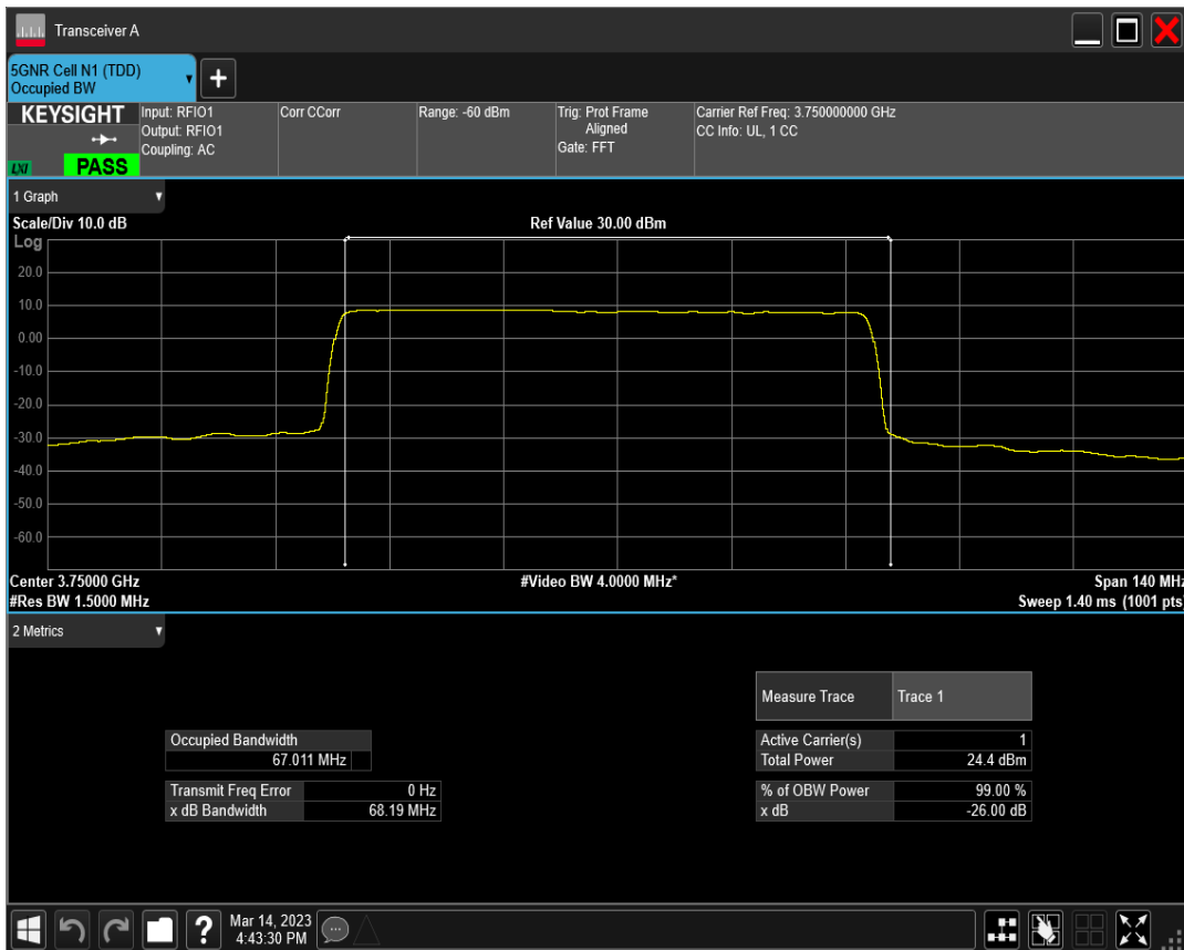
n78(3700-3800) SCS=30kHz CP_QPSK BW=70MHz Channel=650000 RB=189@0
