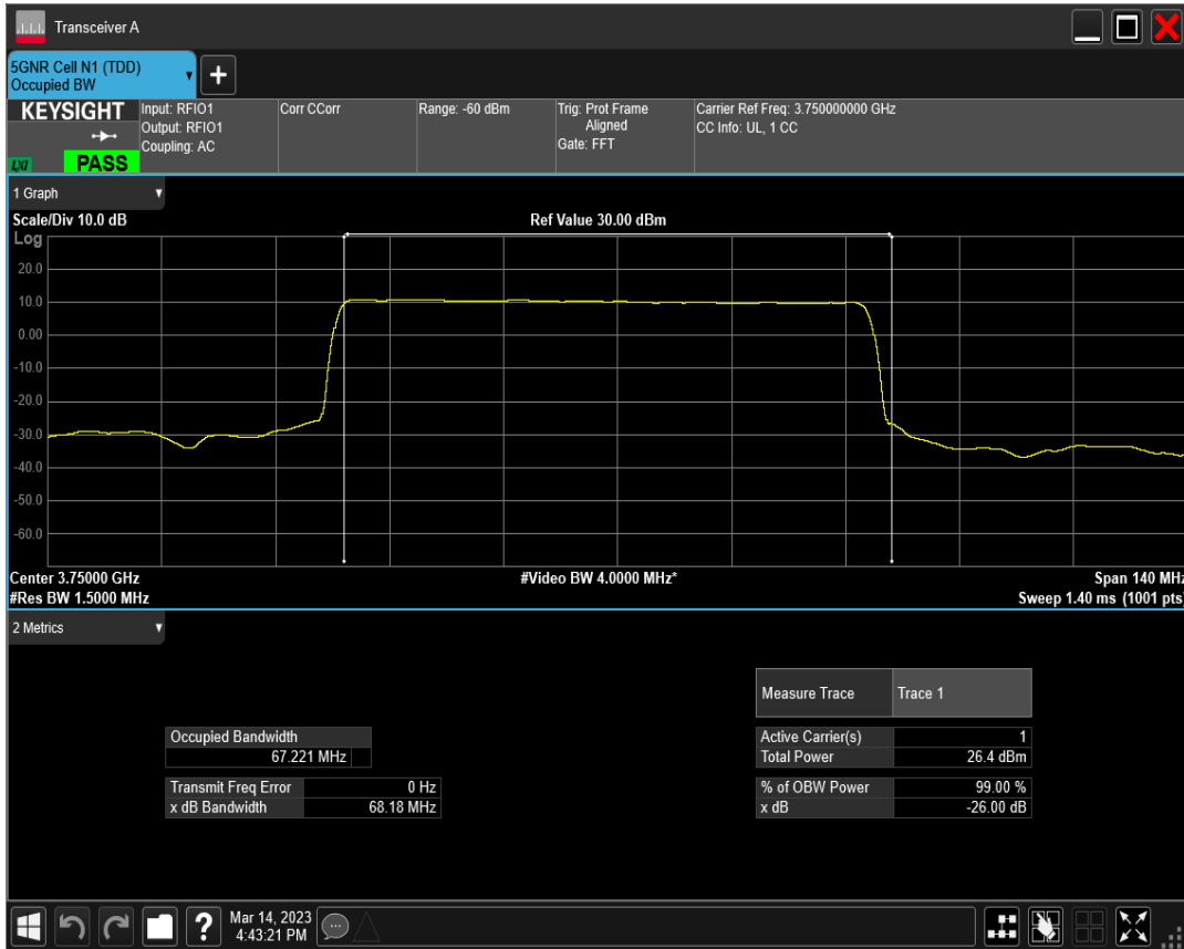
n78(3700-3800) SCS=30kHz DFT_QPSK BW=70MHz Channel=650000 RB=180@0
