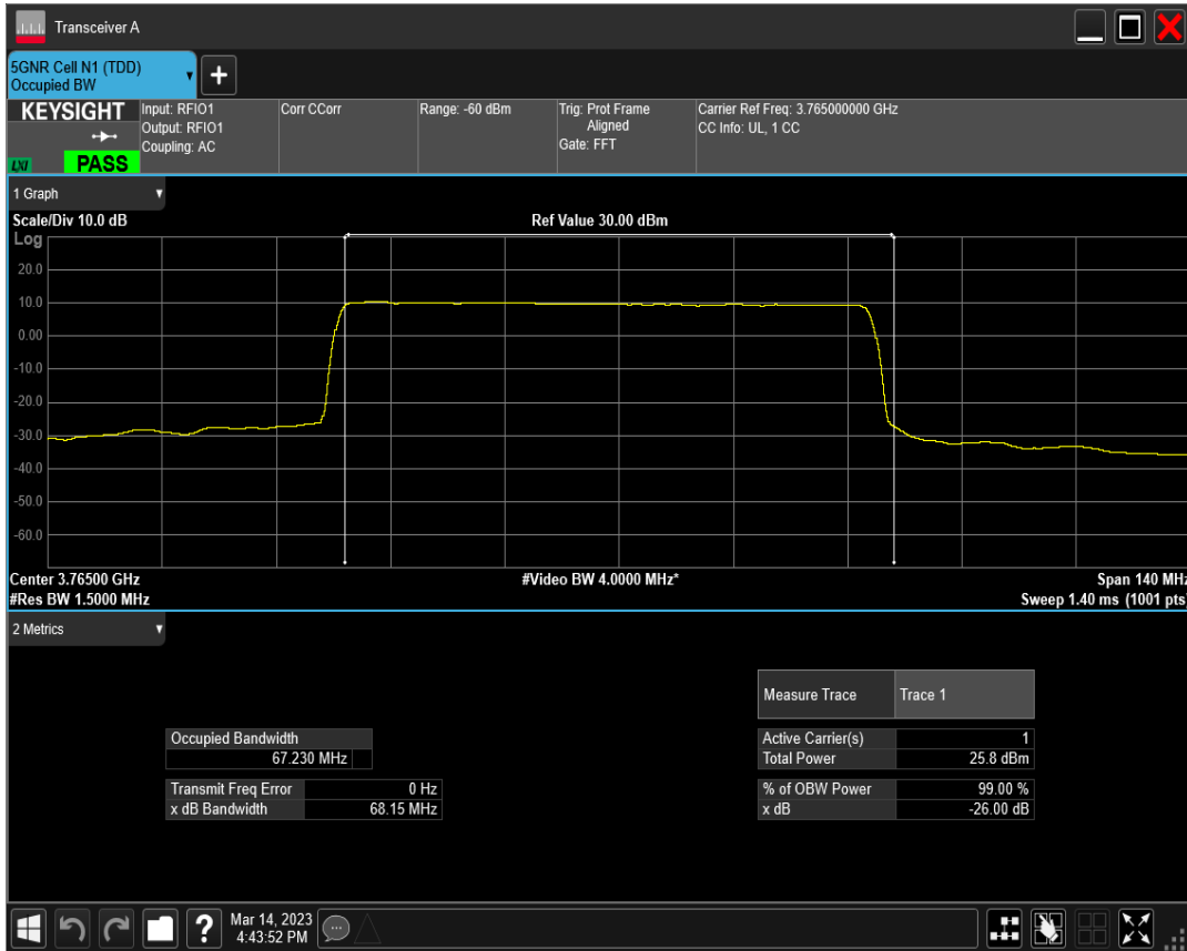
n78(3700-3800) SCS=30kHz DFT_QAM16 BW=70MHz Channel=651000 RB=180@0
