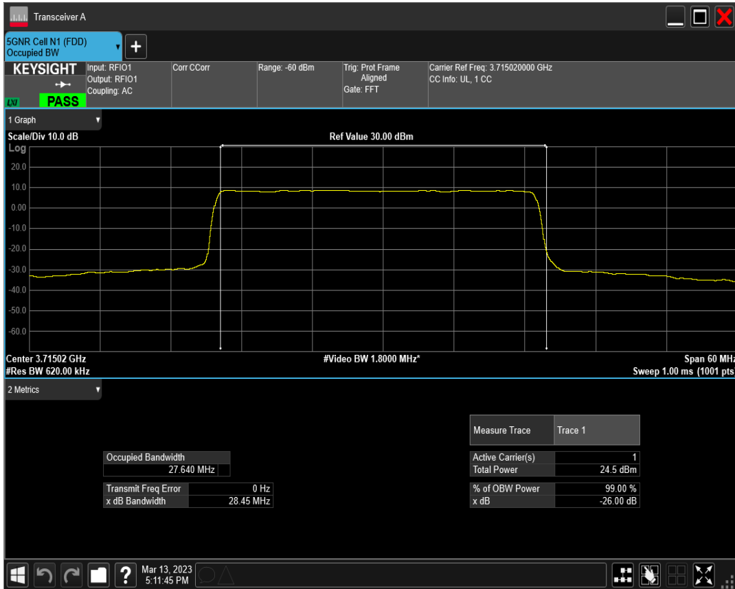
n77(3700-3980) SCS=30kHz DFT_QAM256 BW=30MHz Channel=647668 RB=75@0
