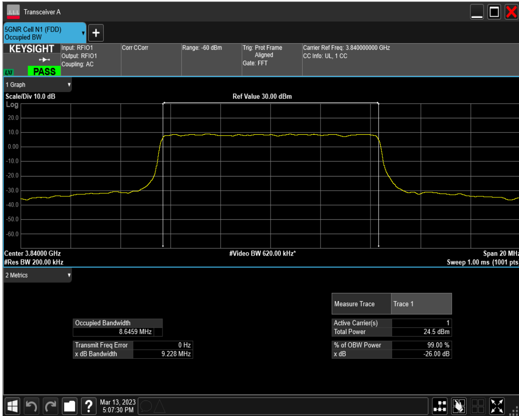
n77(3700-3980) SCS=30kHz DFT_QAM256 BW=10MHz Channel=656000 RB=24@0
