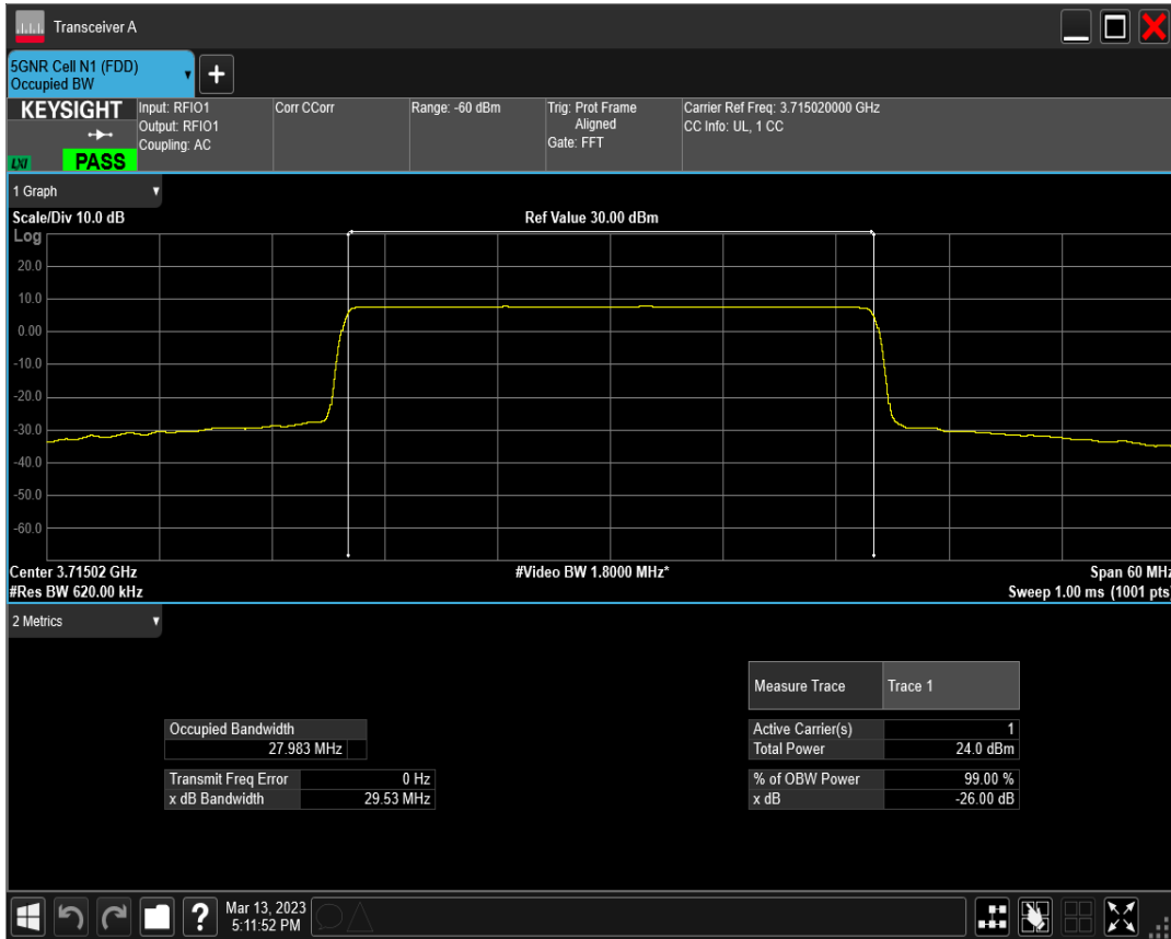
n77(3700-3980) SCS=30kHz DFT_BPSK BW=30MHz Channel=656000 RB=75@0
