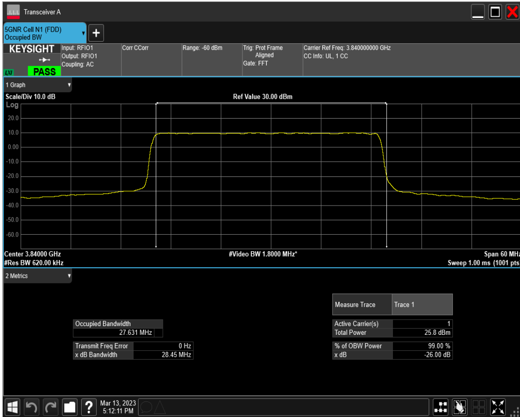
n77(3700-3980) SCS=30kHz DFT_QAM16 BW=30MHz Channel=656000 RB=75@0
