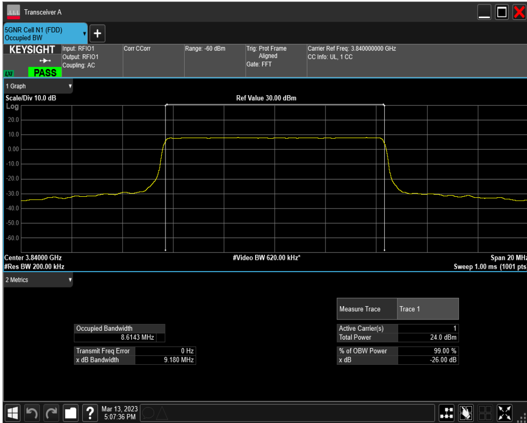
n77(3700-3980) SCS=30kHz DFT_BPSK BW=10MHz Channel=665000 RB=24@0
