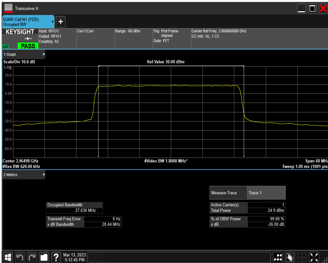
n77(3700-3980) SCS=30kHz DFT_QAM64 BW=30MHz Channel=664332 RB=75@0
