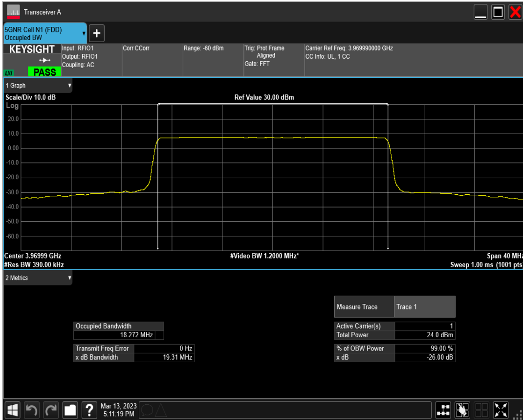
n77(3700-3980) SCS=30kHz DFT_BPSK BW=30MHz Channel=647668 RB=75@0
