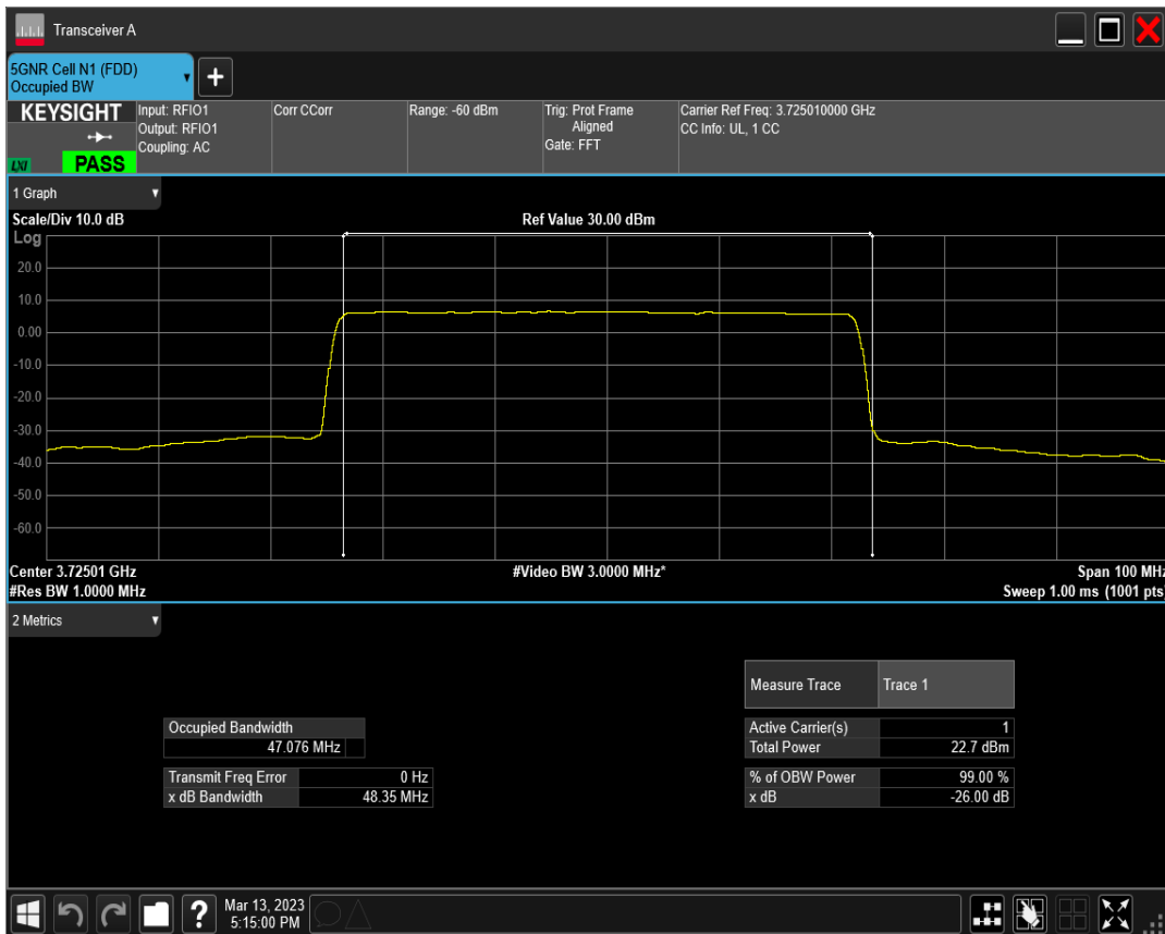
n77(3700-3980) SCS=30kHz CP_QPSK BW=50MHz Channel=648334 RB=133@0
