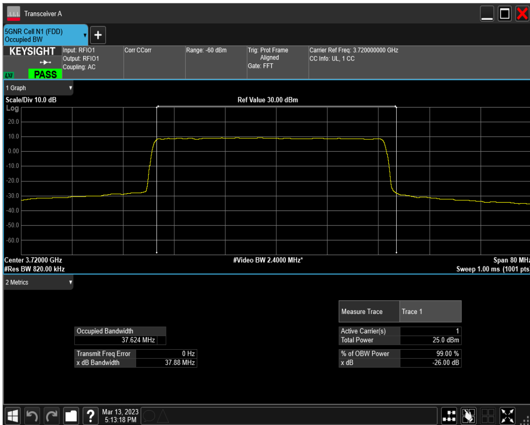
n77(3700-3980) SCS=30kHz DFT_QAM64 BW=40MHz Channel=648000 RB=100@0
