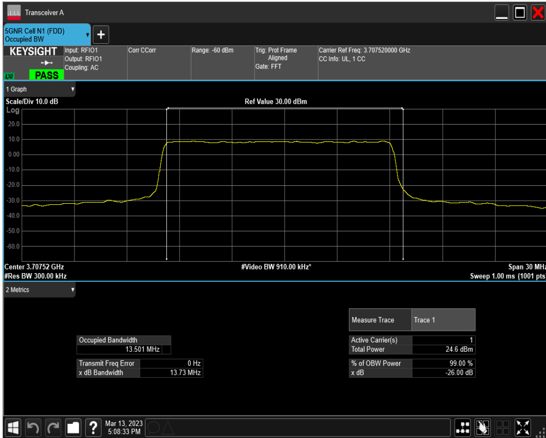
n77(3700-3980) SCS=30kHz DFT_QAM256 BW=15MHz Channel=647168 RB=36@0
