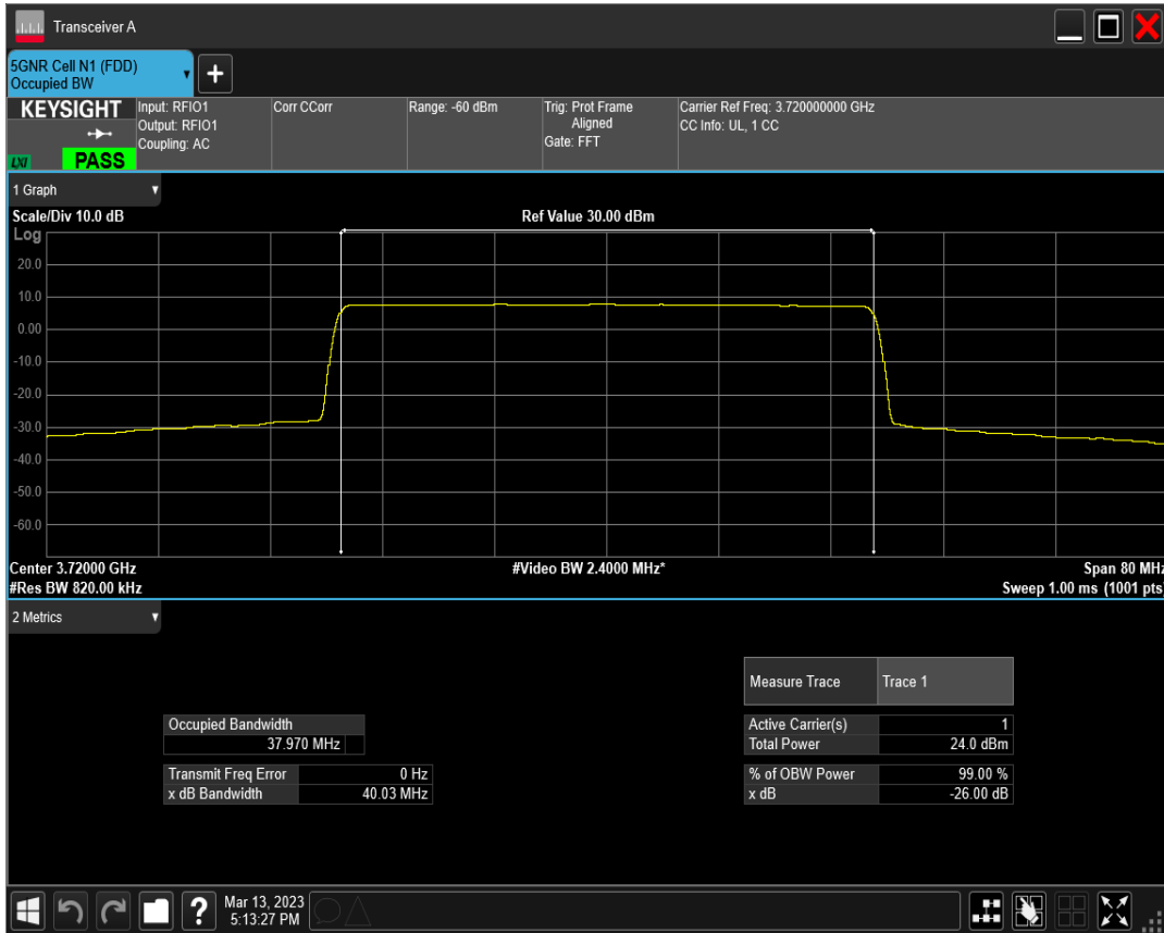
n77(3700-3980) SCS=30kHz DFT_BPSK BW=40MHz Channel=656000 RB=100@0
