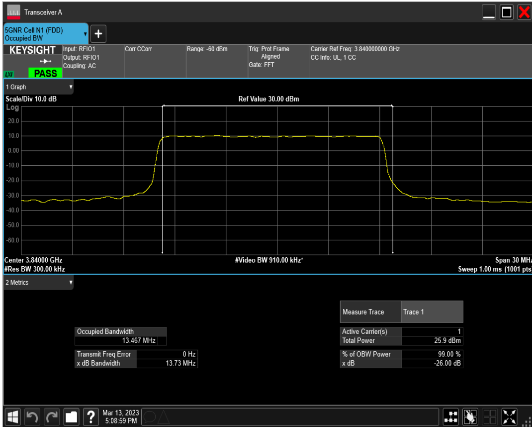
n77(3700-3980) SCS=30kHz DFT_QAM16 BW=15MHz Channel=656000 RB=36@0
