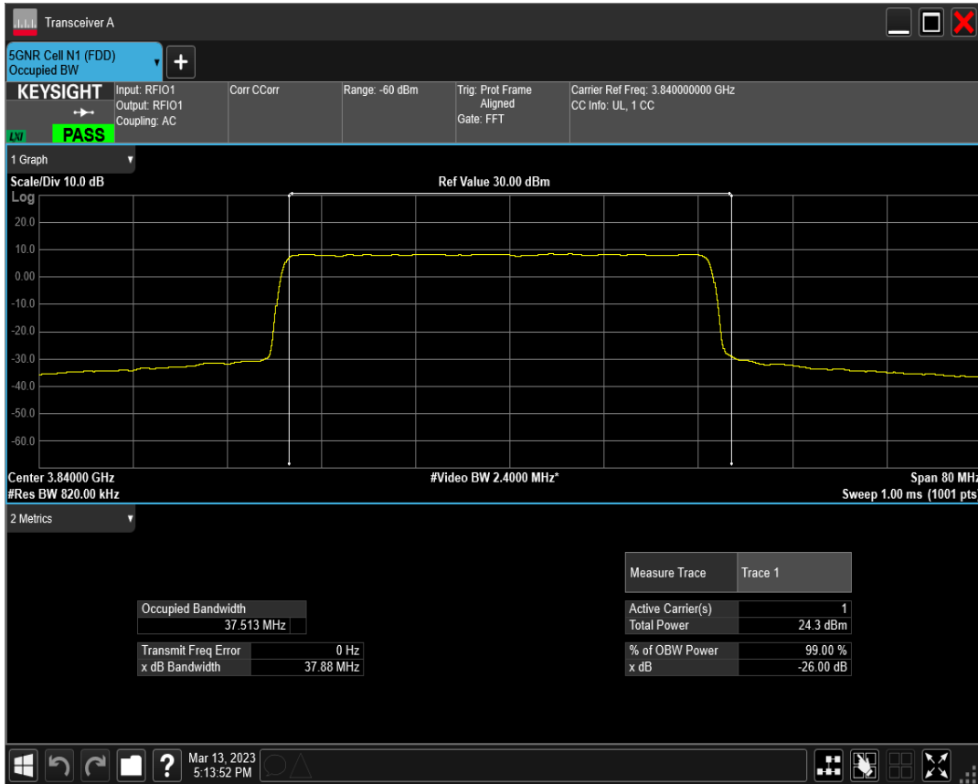
n77(3700-3980) SCS=30kHz DFT_QAM256 BW=40MHz Channel=656000 RB=100@0
