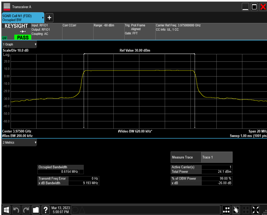
n77(3700-3980) SCS=30kHz DFT_BPSK BW=15MHz Channel=647168 RB=36@0
