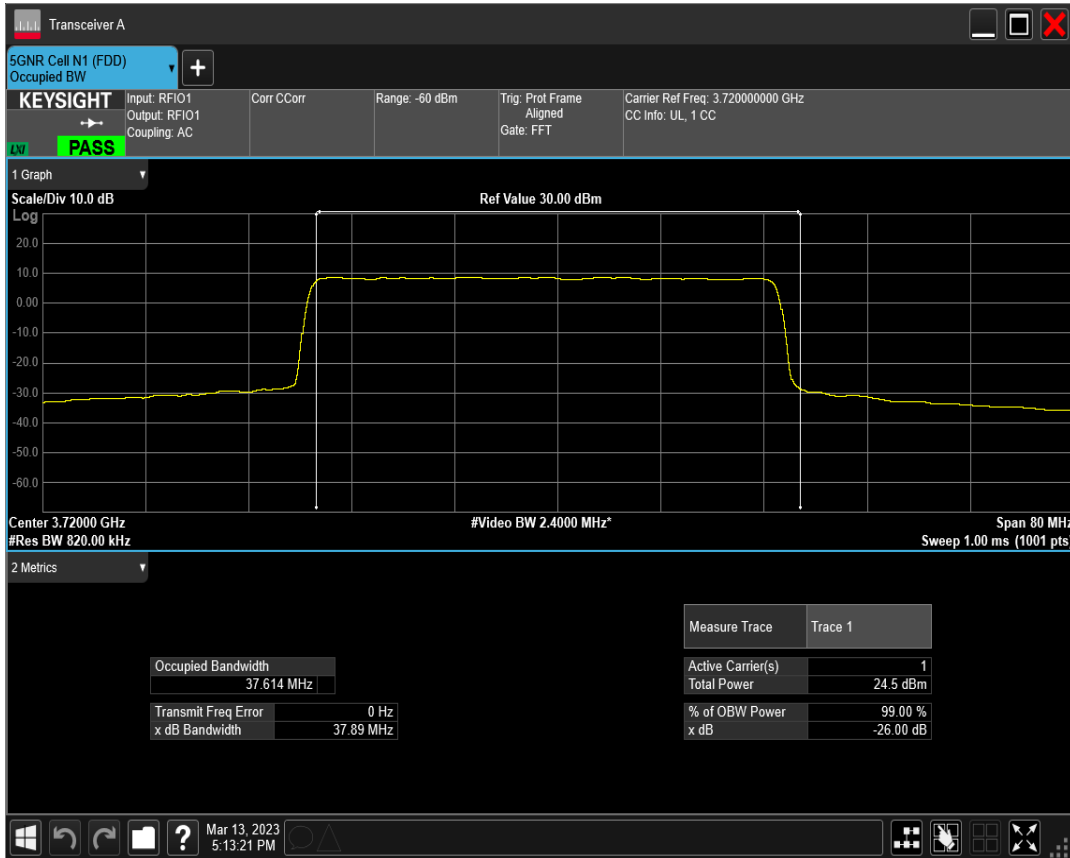
n77(3700-3980) SCS=30kHz DFT_QAM256 BW=40MHz Channel=648000 RB=100@0
