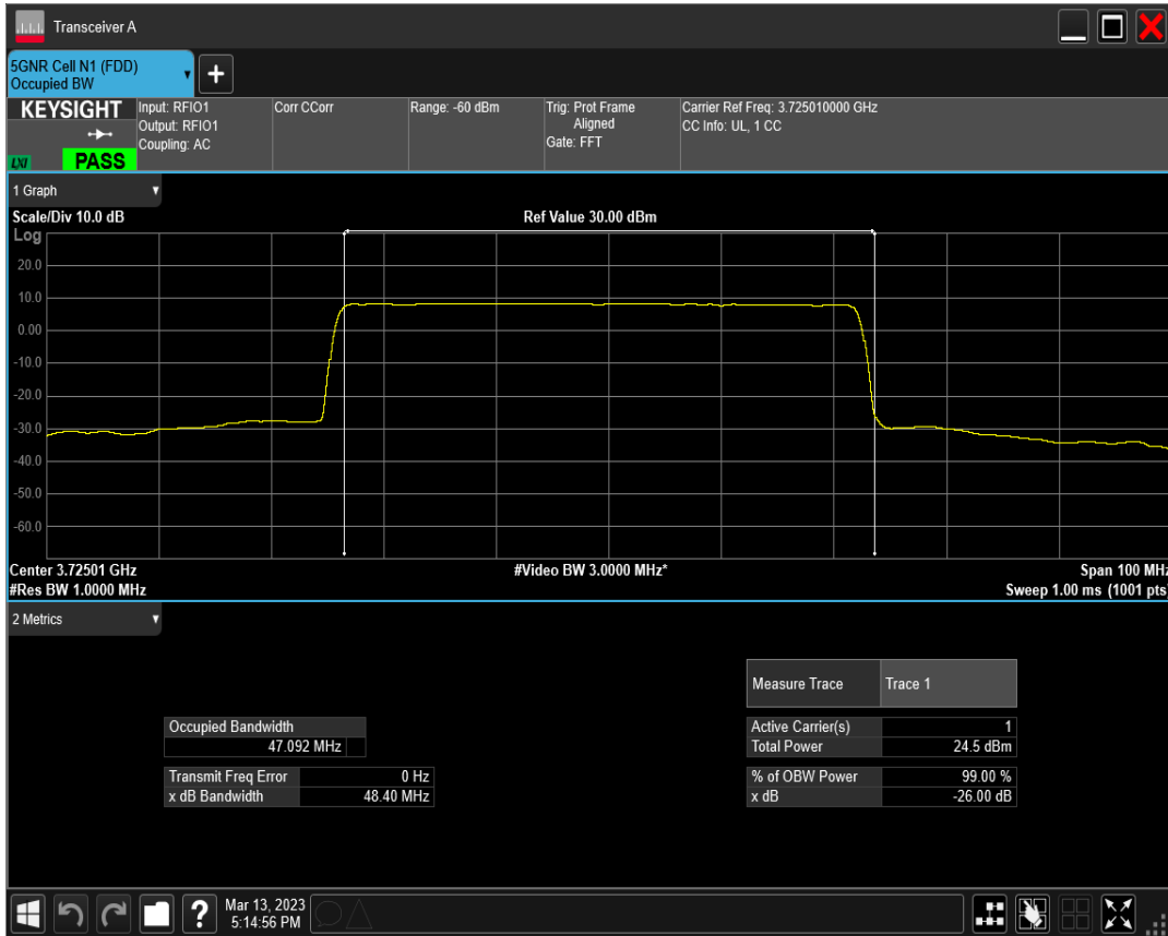
n77(3700-3980) SCS=30kHz DFT_QAM256 BW=50MHz Channel=648334 RB=128@0
