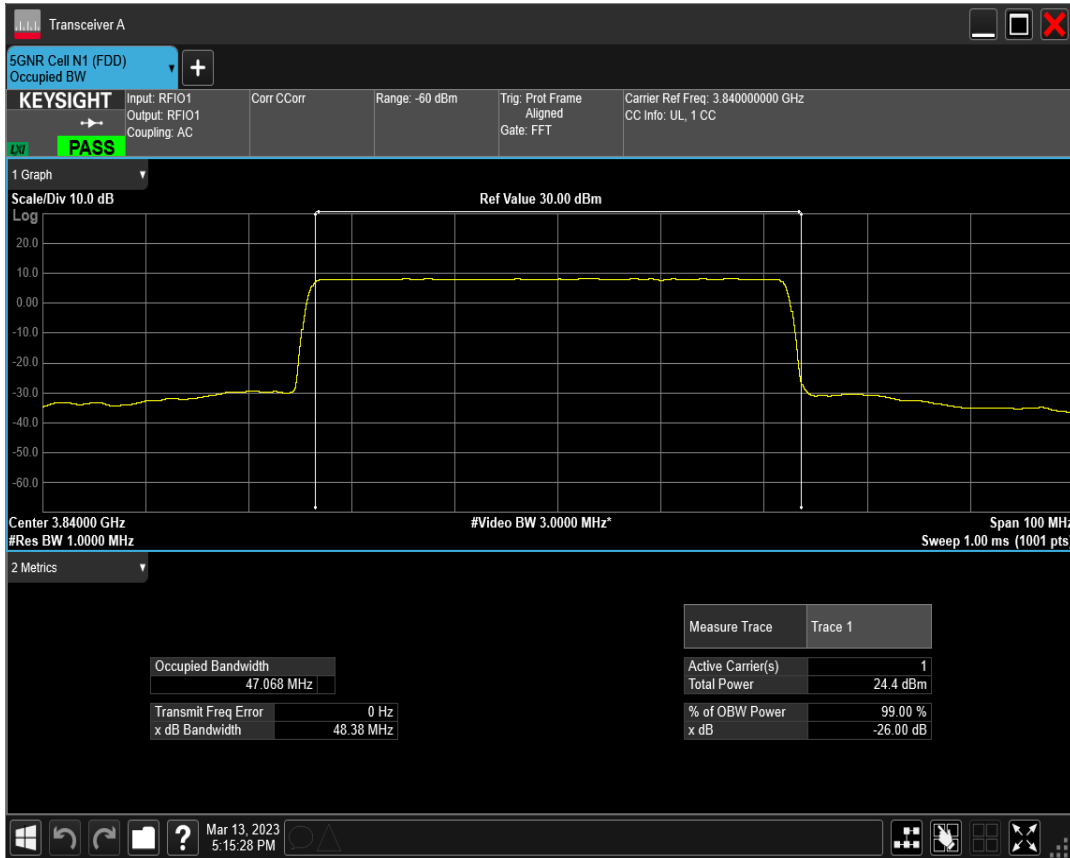
n77(3700-3980) SCS=30kHz DFT_QAM256 BW=50MHz Channel=656000 RB=128@0
