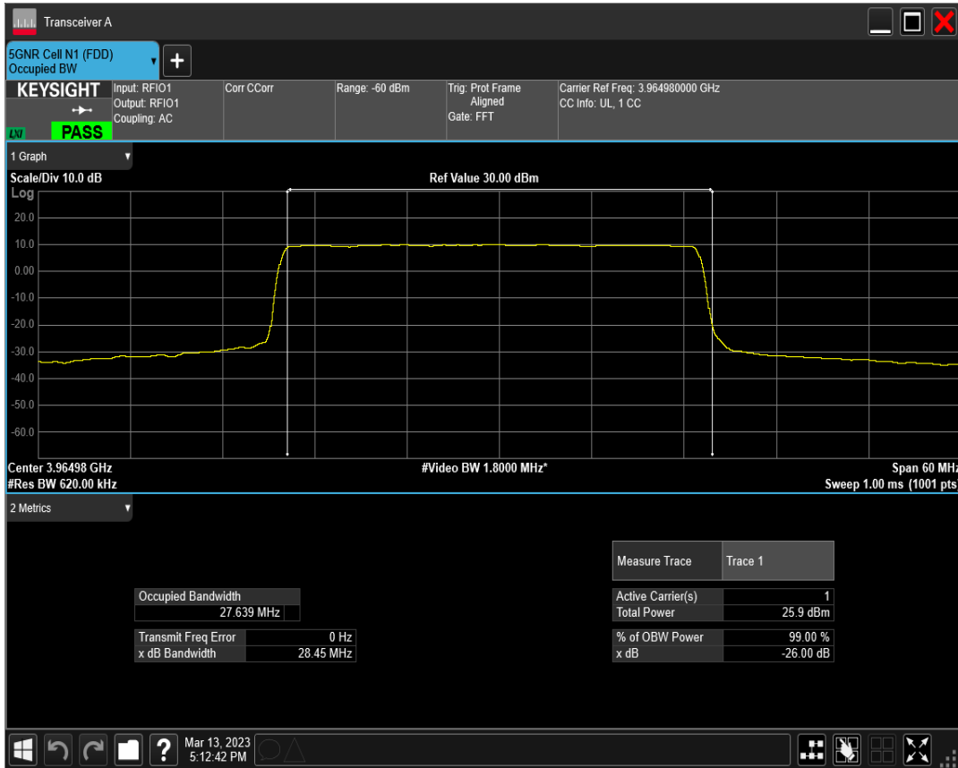
n77(3700-3980) SCS=30kHz DFT_QAM16 BW=30MHz Channel=664332 RB=75@0
