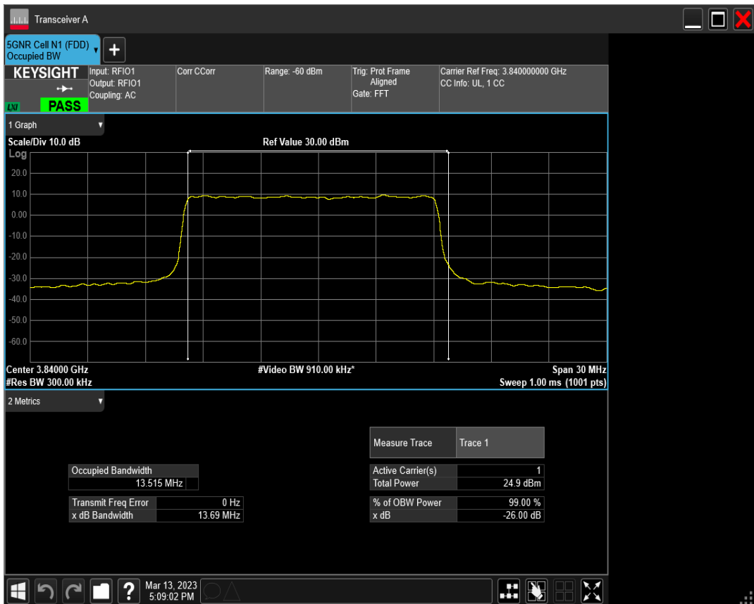
n77(3700-3980) SCS=30kHz DFT_QAM64 BW=15MHz Channel=656000 RB=36@0
