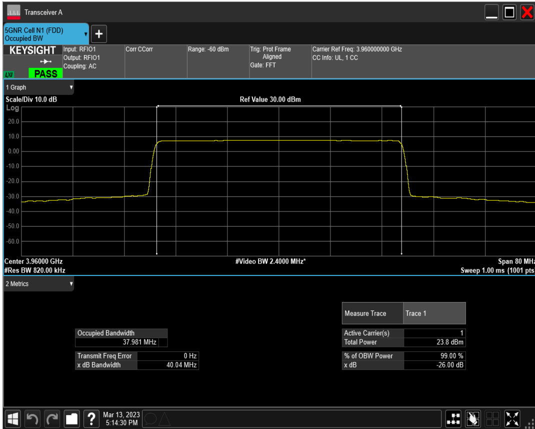
n77(3700-3980) SCS=30kHz DFT_BPSK BW=50MHz Channel=648334 RB=128@0
