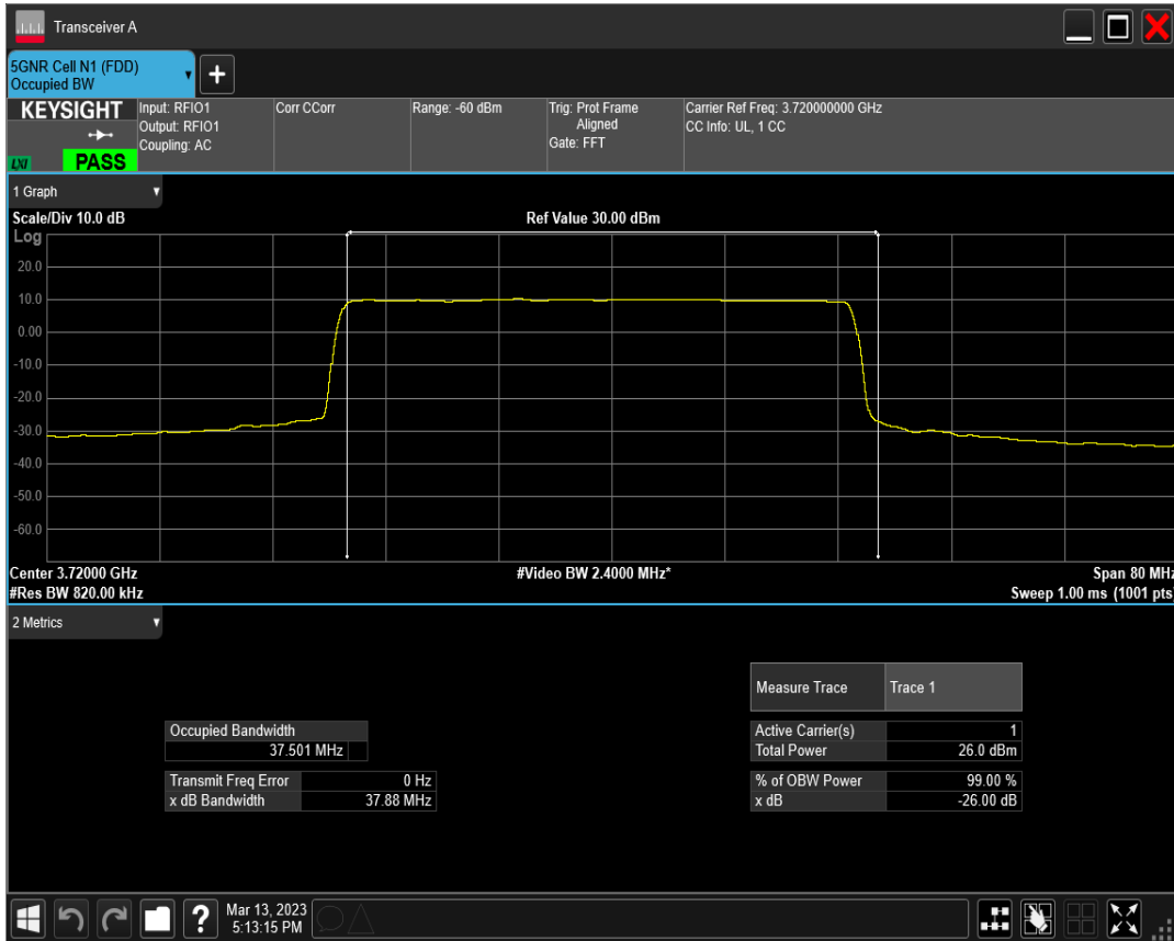
n77(3700-3980) SCS=30kHz DFT_QAM16 BW=40MHz Channel=648000 RB=100@0
