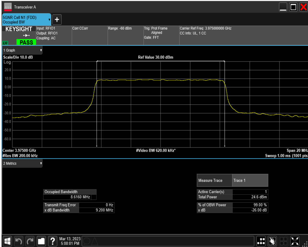
n77(3700-3980) SCS=30kHz DFT_QAM256 BW=10MHz Channel=665000 RB=24@0
