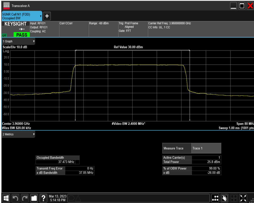
n77(3700-3980) SCS=30kHz DFT_QAM16 BW=40MHz Channel=664000 RB=100@0
