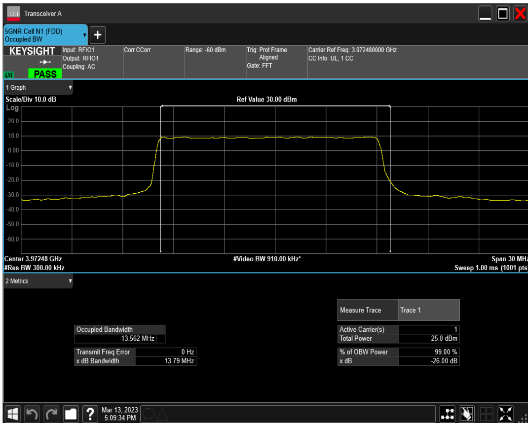
n77(3700-3980) SCS=30kHz DFT_QAM64 BW=15MHz Channel=664832 RB=36@0
