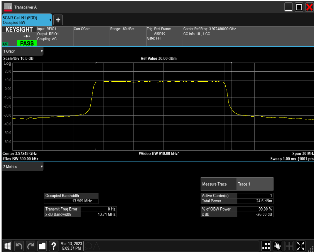
n77(3700-3980) SCS=30kHz DFT_QAM256 BW=15MHz Channel=664832 RB=36@0
