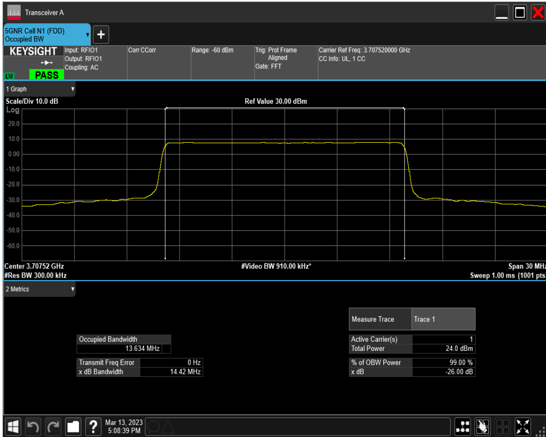
n77(3700-3980) SCS=30kHz DFT_BPSK BW=15MHz Channel=656000 RB=36@0
