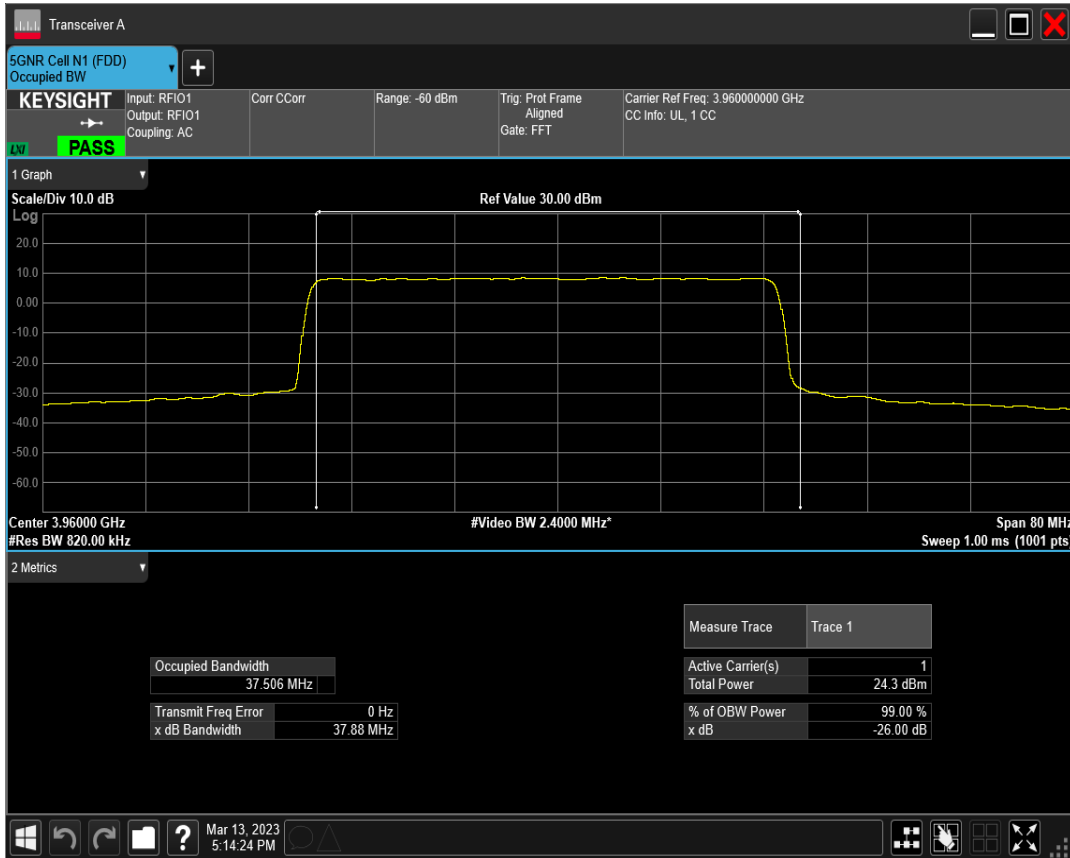
n77(3700-3980) SCS=30kHz DFT_QAM256 BW=40MHz Channel=664000 RB=100@0
