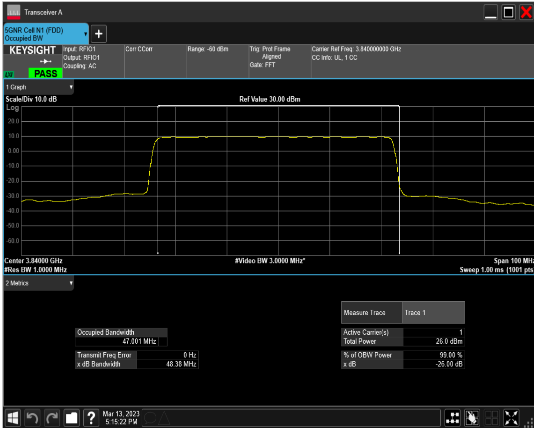
n77(3700-3980) SCS=30kHz DFT_QAM16 BW=50MHz Channel=656000 RB=128@0
