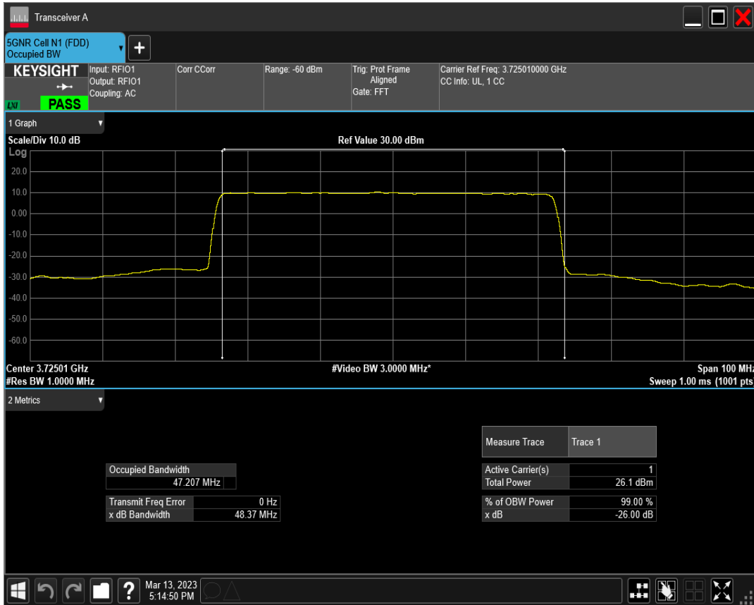
n77(3700-3980) SCS=30kHz DFT_QAM16 BW=50MHz Channel=648334 RB=128@0
