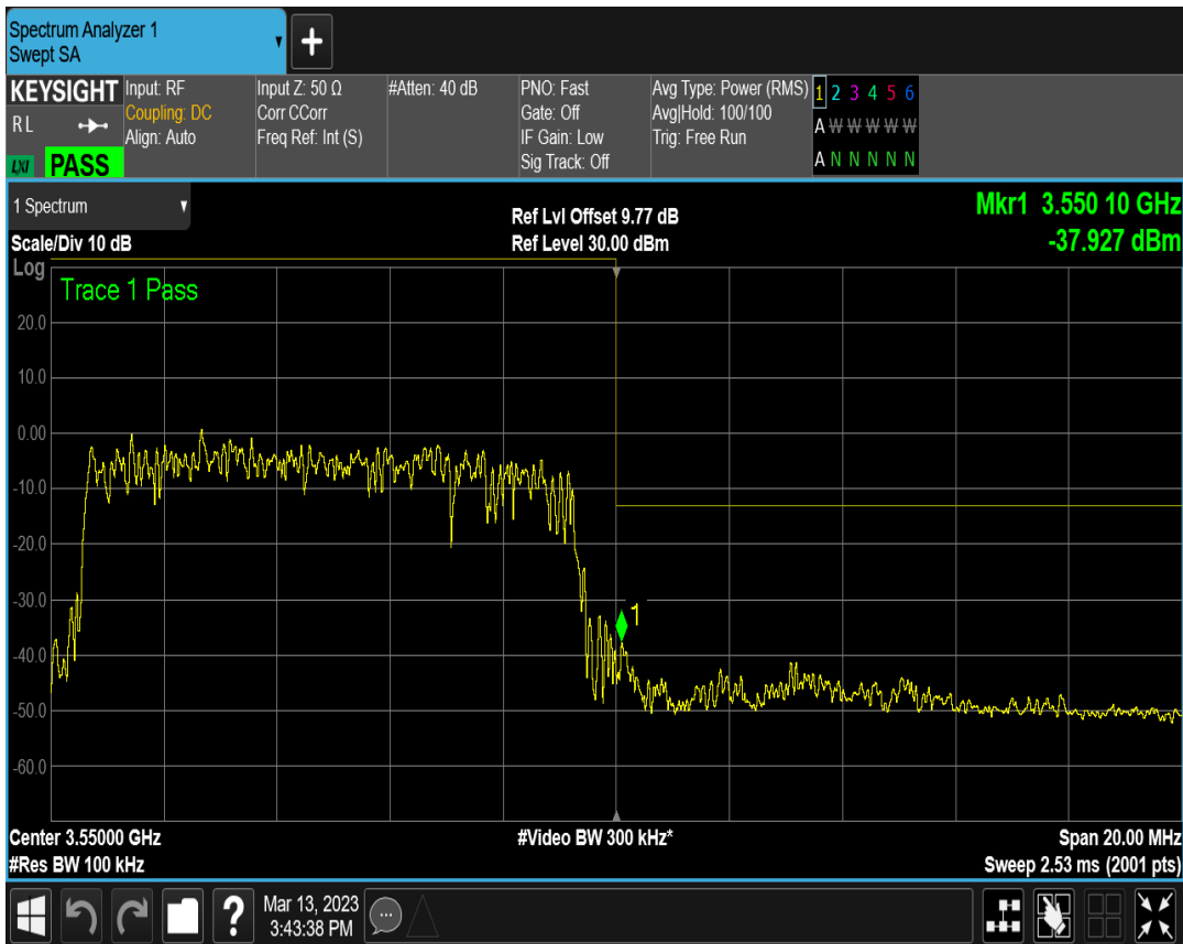
n77(3450-3550) SCS=30kHz DFT_QPSK BW=10MHz Channel=636332 RB=1@23
