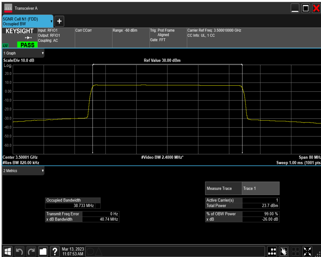
n77(3450-3550) SCS=15kHz DFT_BPSK BW=40MHz Channel=635332 RB=216@0
