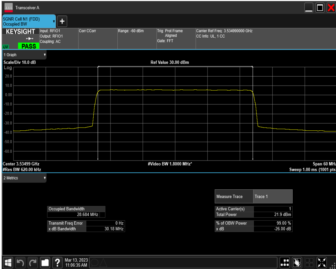
n77(3450-3550) SCS=15kHz CP_QPSK BW=30MHz Channel=635666 RB=160@0
