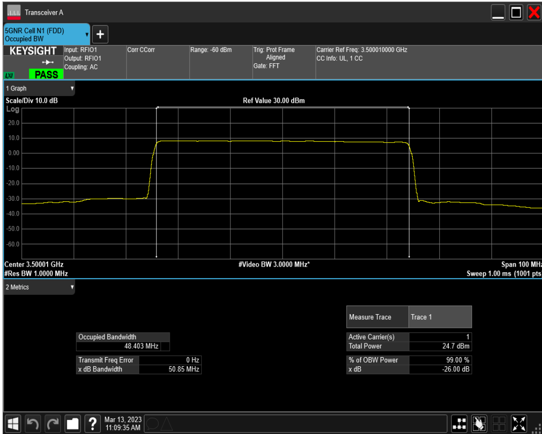
n77(3450-3550) SCS=15kHz DFT_QAM64 BW=50MHz Channel=633334 RB=270@0
