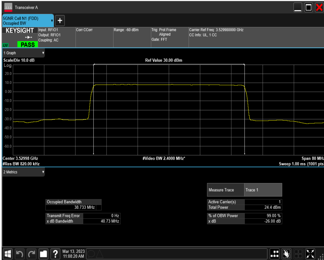
n77(3450-3550) SCS=15kHz DFT_QAM64 BW=40MHz Channel=635332 RB=216@0
