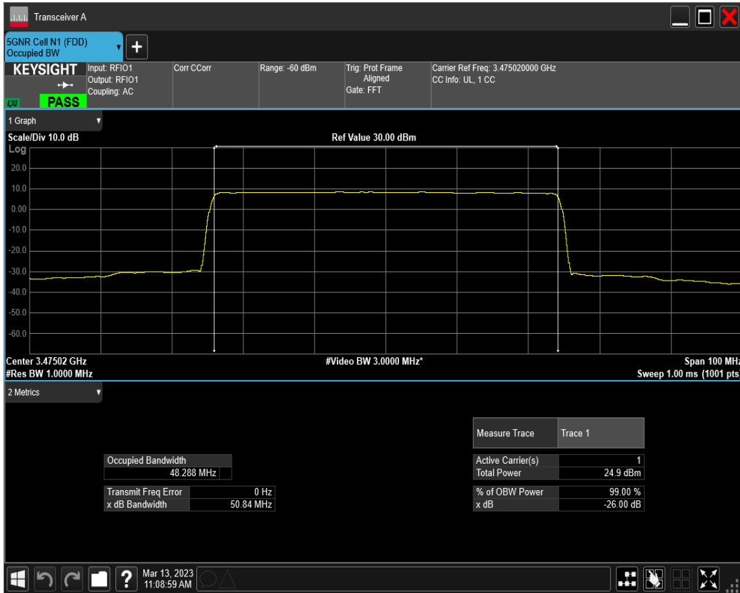
n77(3450-3550) SCS=15kHz DFT_QAM64 BW=50MHz Channel=631668 RB=270@0
