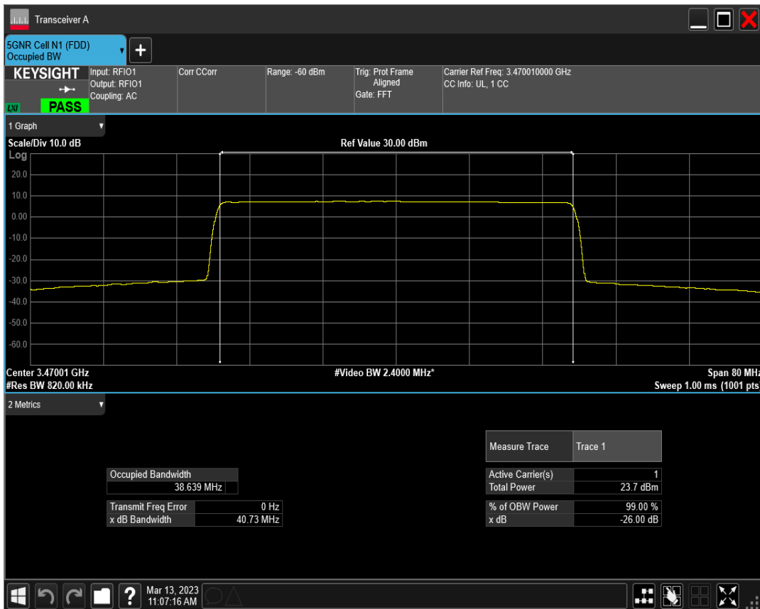
n77(3450-3550) SCS=15kHz DFT_BPSK BW=40MHz Channel=633334 RB=216@0
