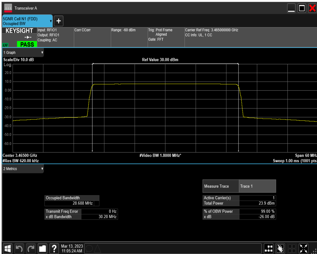
n77(3450-3550) SCS=15kHz DFT_BPSK BW=30MHz Channel=633334 RB=160@0
