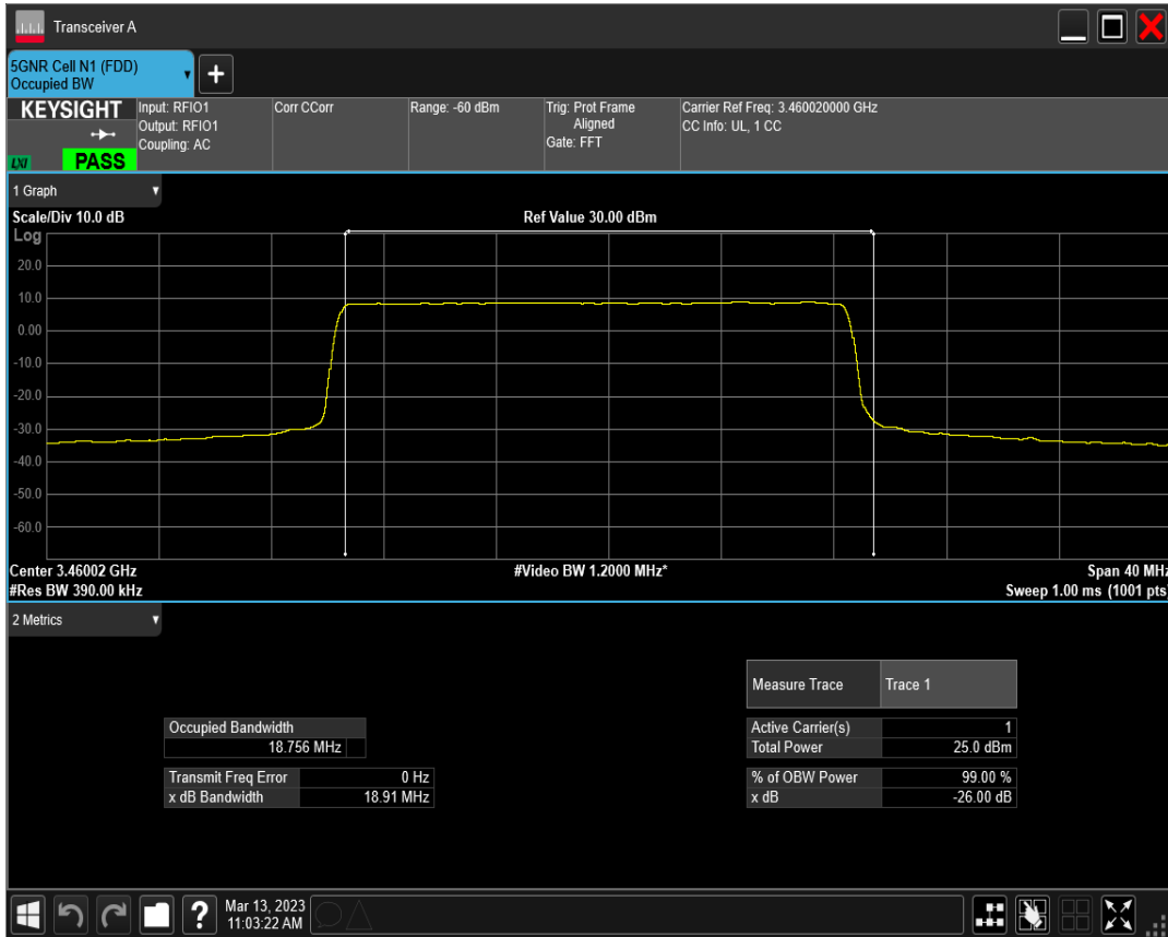
n77(3450-3550) SCS=15kHz DFT_QAM64 BW=20MHz Channel=630668 RB=100@0
