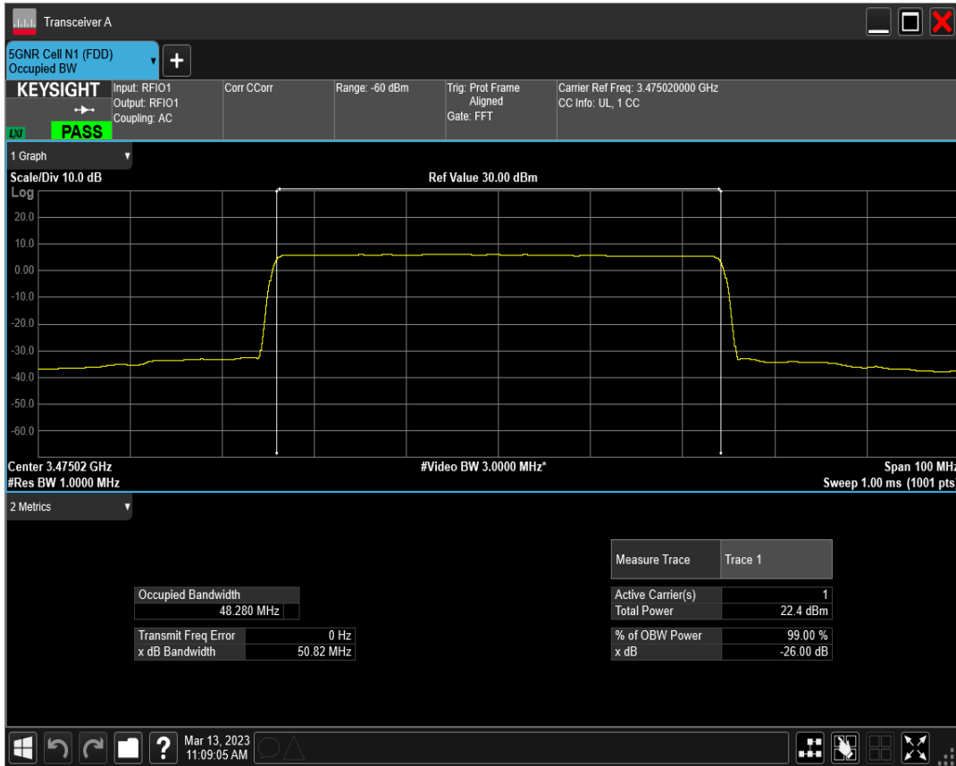
n77(3450-3550) SCS=15kHz CP_QPSK BW=50MHz Channel=631668 RB=270@0
