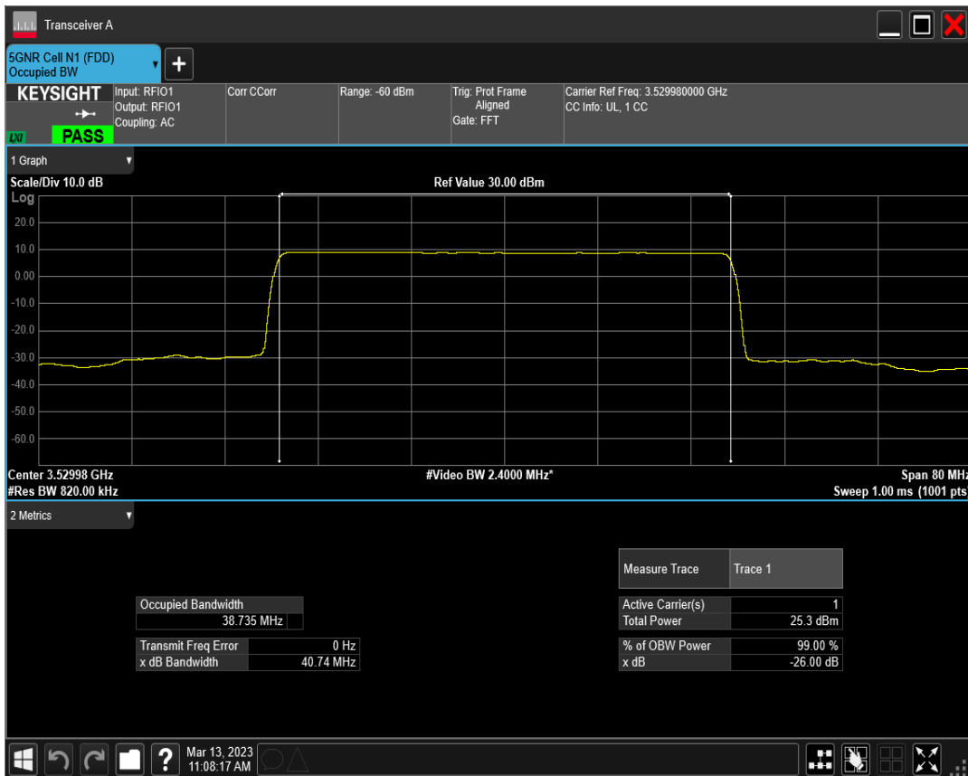
n77(3450-3550) SCS=15kHz DFT_QAM16 BW=40MHz Channel=635332 RB=216@0
