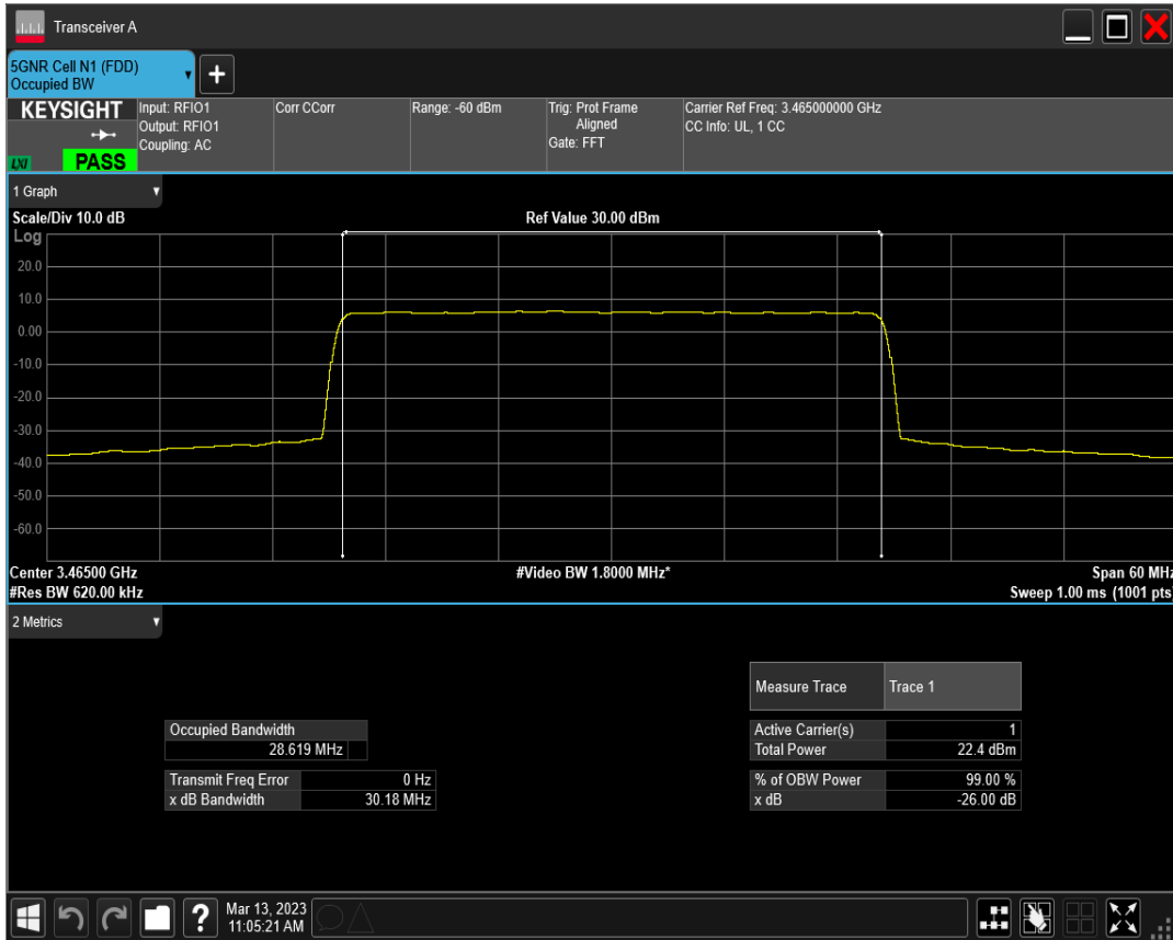
n77(3450-3550) SCS=15kHz CP_QPSK BW=30MHz Channel=631000 RB=160@0
