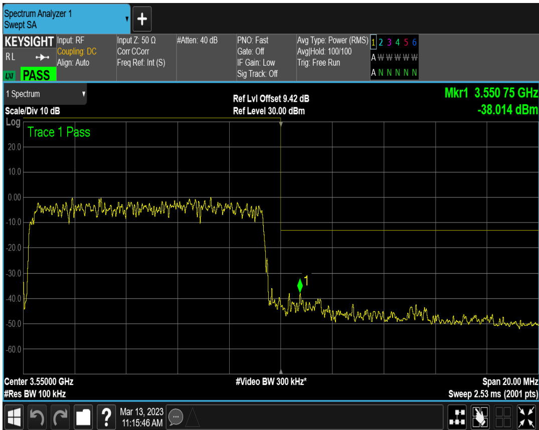
n77(3450-3550) SCS=15kHz DFT_QPSK BW=10MHz Channel=636332 RB=1@51
