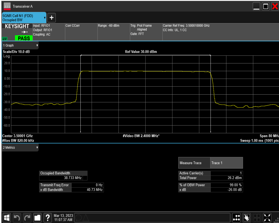
n77(3450-3550) SCS=15kHz DFT_QPSK BW=40MHz Channel=633334 RB=216@0
