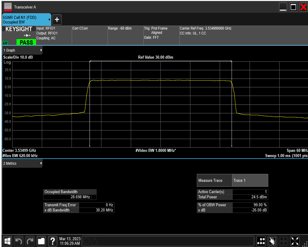
n77(3450-3550) SCS=15kHz DFT_QAM64 BW=30MHz Channel=635666 RB=160@0
