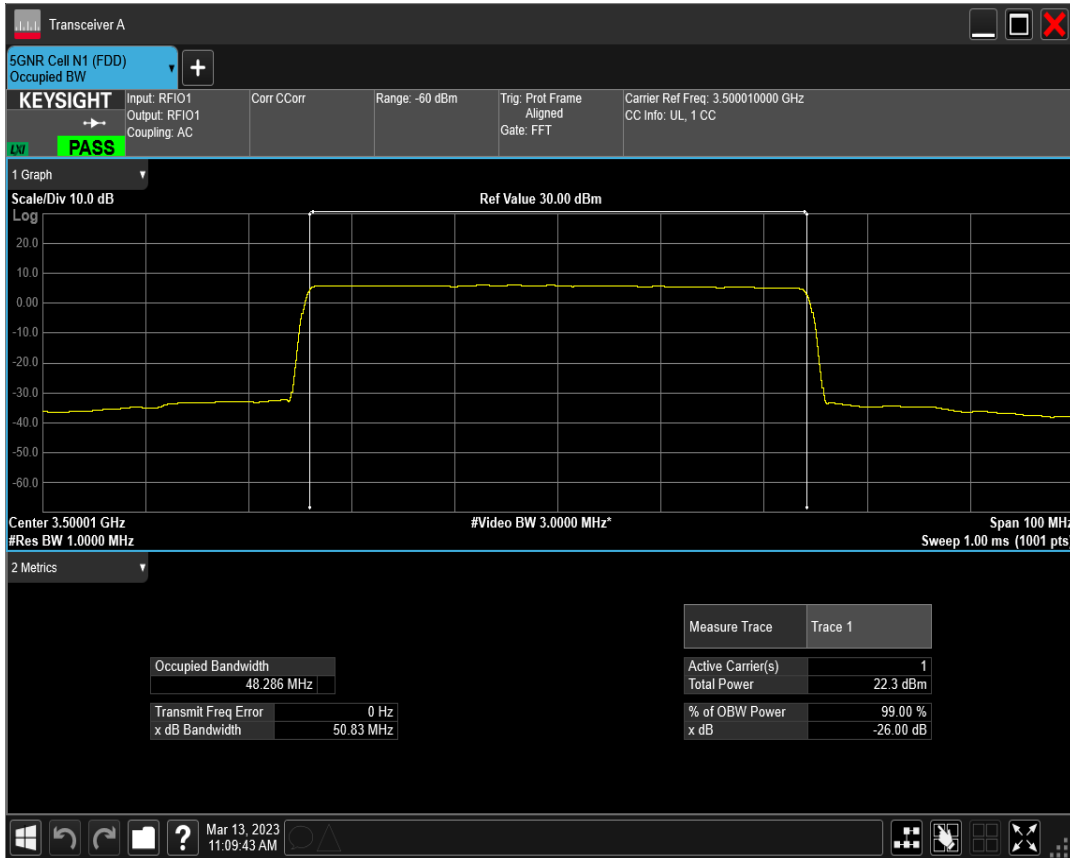
n77(3450-3550) SCS=15kHz CP_QPSK BW=50MHz Channel=633334 RB=270@0
