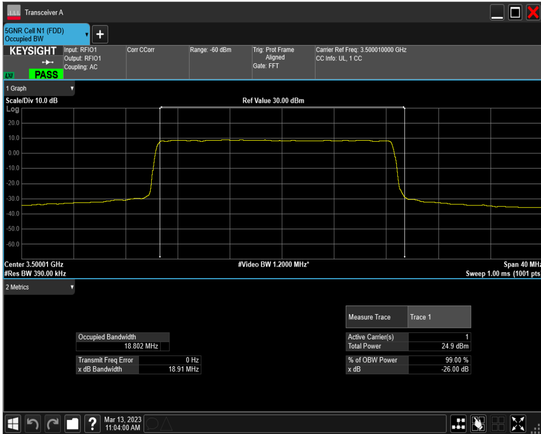
n77(3450-3550) SCS=15kHz DFT_QAM64 BW=20MHz Channel=633334 RB=100@0
