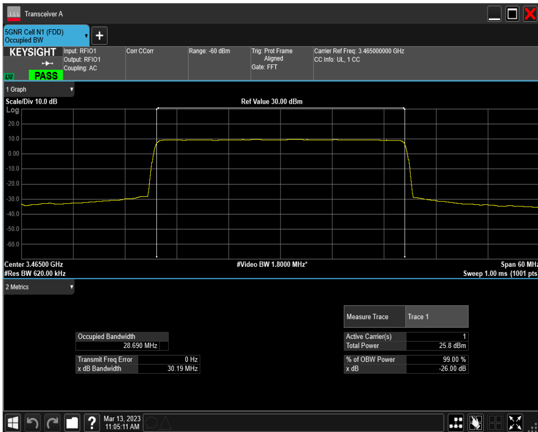
n77(3450-3550) SCS=15kHz DFT_QAM16 BW=30MHz Channel=631000 RB=160@0
