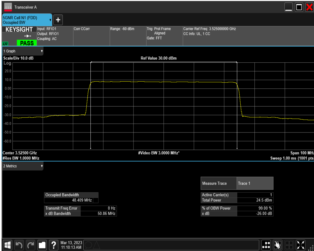
n77(3450-3550) SCS=15kHz DFT_QAM64 BW=50MHz Channel=635000 RB=270@0
