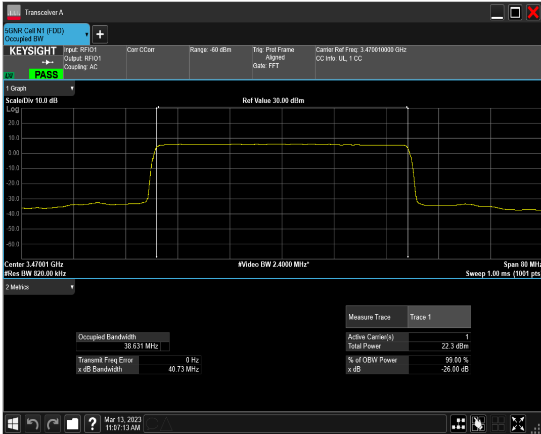
n77(3450-3550) SCS=15kHz CP_QPSK BW=40MHz Channel=631334 RB=216@0
