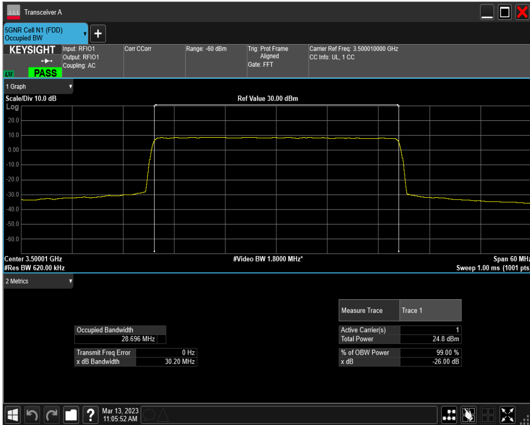
n77(3450-3550) SCS=15kHz DFT_QAM64 BW=30MHz Channel=633334 RB=160@0
