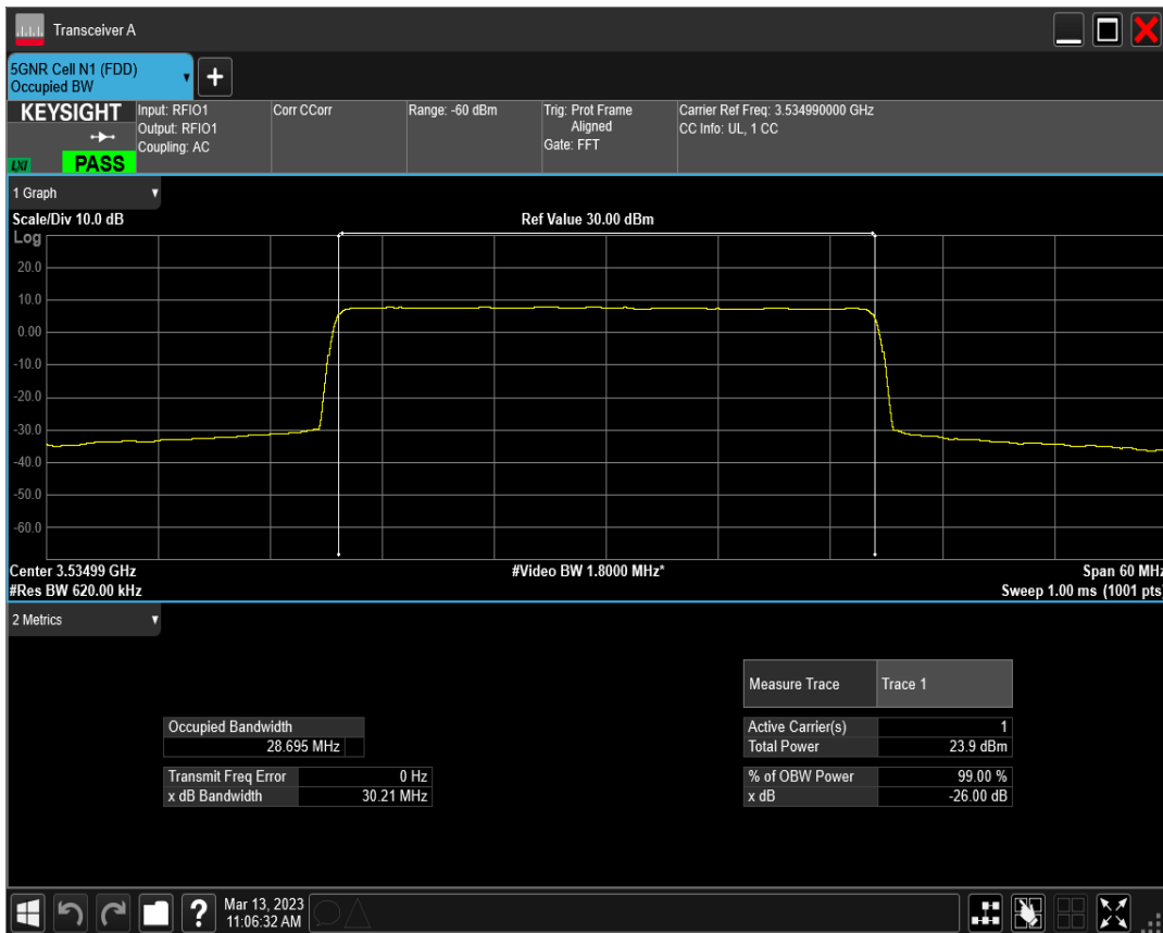
n77(3450-3550) SCS=15kHz DFT_QAM256 BW=30MHz Channel=635666 RB=160@0
