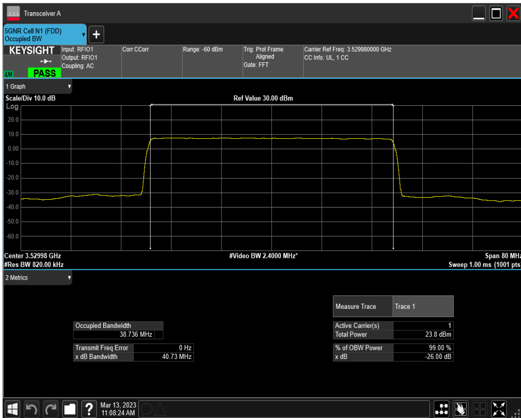
n77(3450-3550) SCS=15kHz DFT_QAM256 BW=40MHz Channel=635332 RB=216@0
