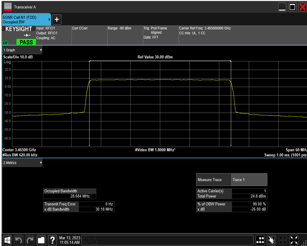
n77(3450-3550) SCS=15kHz DFT_QAM64 BW=30MHz Channel=631000 RB=160@0
