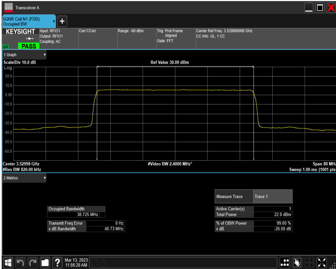
n77(3450-3550) SCS=15kHz CP_QPSK BW=40MHz Channel=635332 RB=216@0
