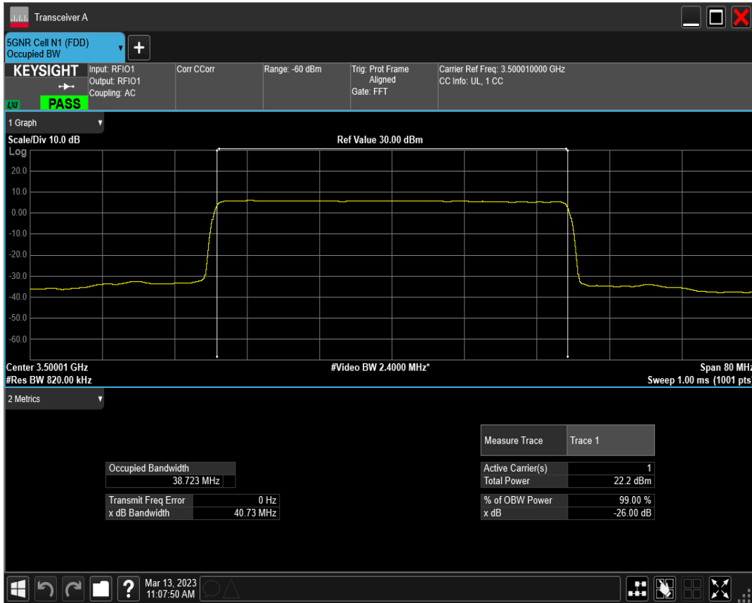
n77(3450-3550) SCS=15kHz CP_QPSK BW=40MHz Channel=633334 RB=216@0
