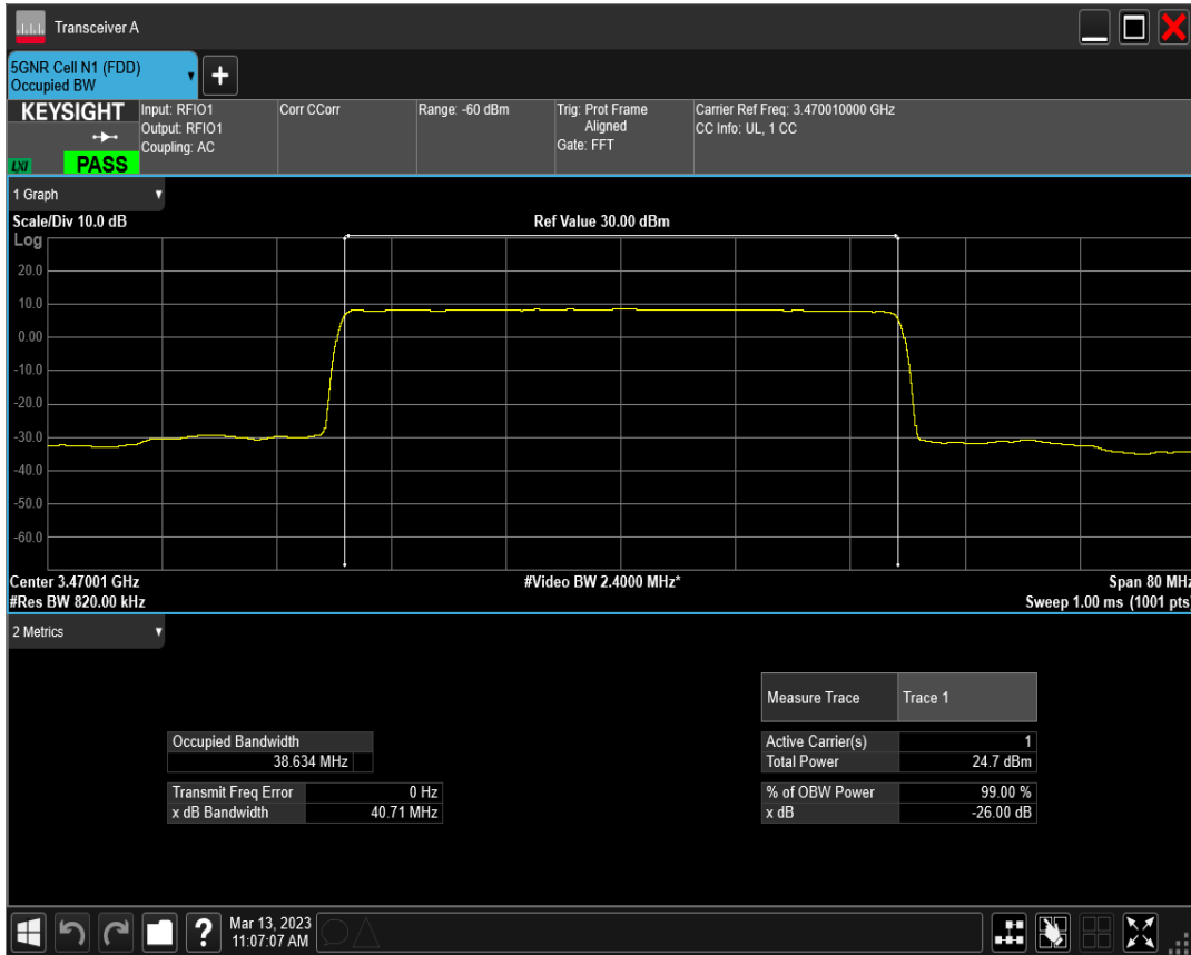
n77(3450-3550) SCS=15kHz DFT_QAM64 BW=40MHz Channel=631334 RB=216@0
