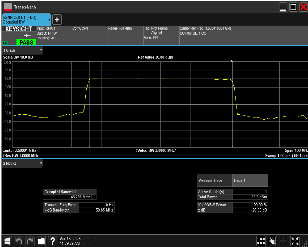
n77(3450-3550) SCS=15kHz DFT_QPSK BW=50MHz Channel=633334 RB=270@0
