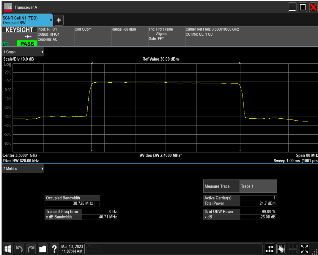
n77(3450-3550) SCS=15kHz DFT_QAM64 BW=40MHz Channel=633334 RB=216@0
