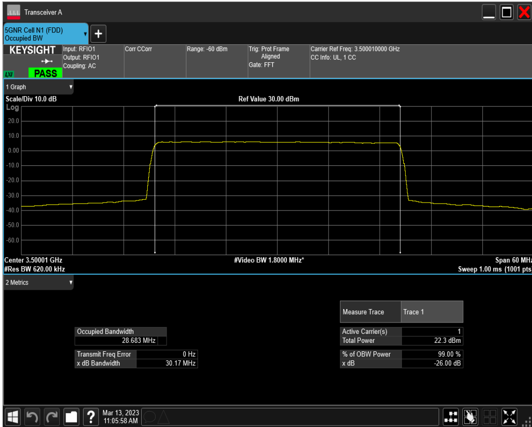
n77(3450-3550) SCS=15kHz CP_QPSK BW=30MHz Channel=633334 RB=160@0
