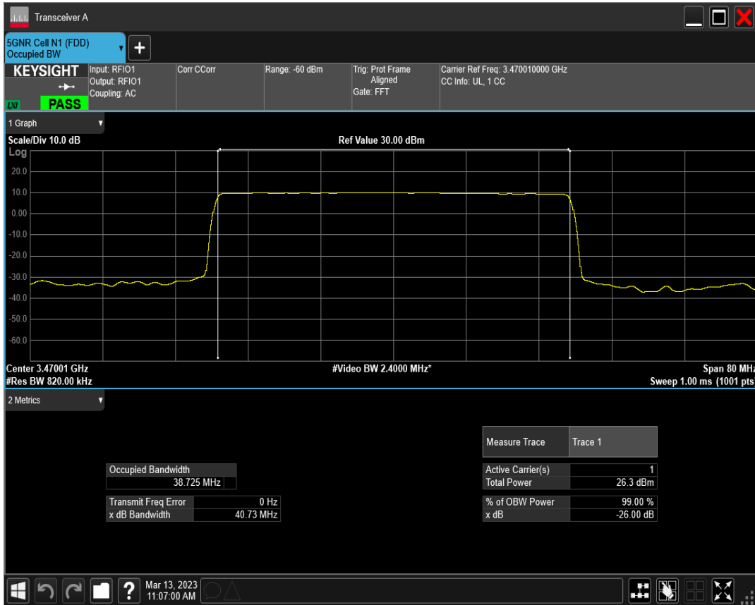
n77(3450-3550) SCS=15kHz DFT_QPSK BW=40MHz Channel=631334 RB=216@0
