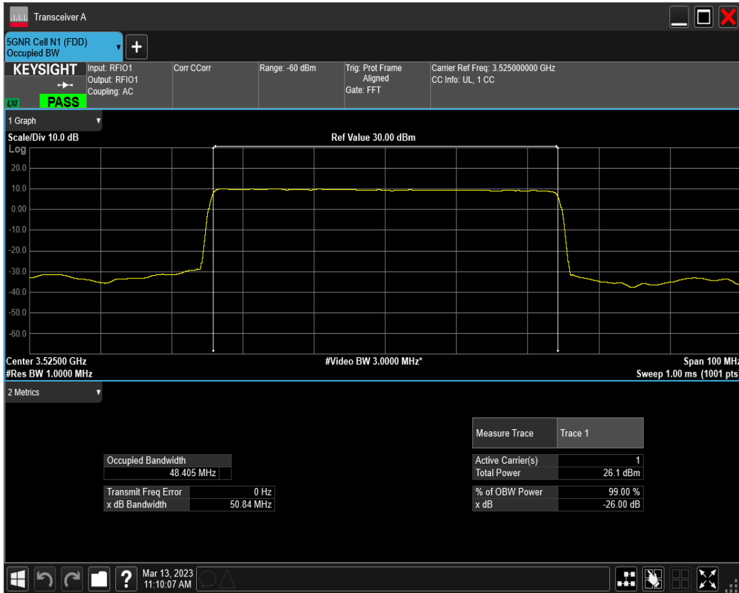
n77(3450-3550) SCS=15kHz DFT_QPSK BW=50MHz Channel=635000 RB=270@0
