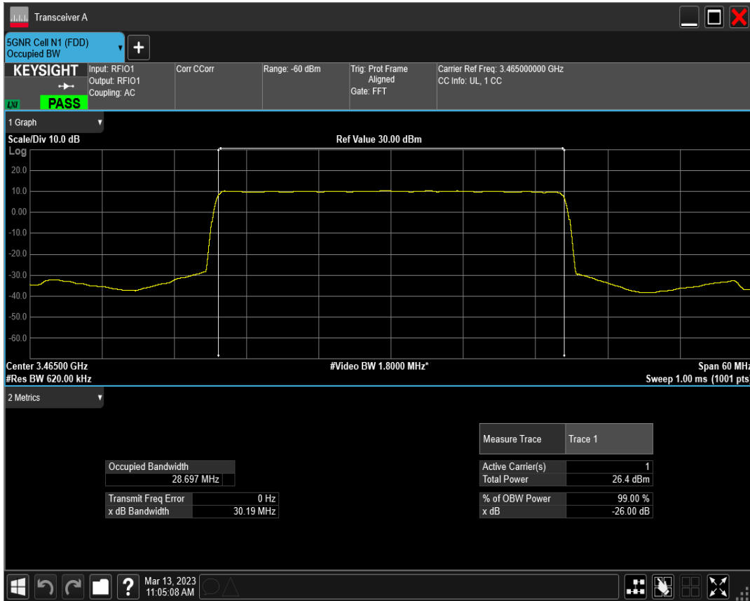
n77(3450-3550) SCS=15kHz DFT_QPSK BW=30MHz Channel=631000 RB=160@0
