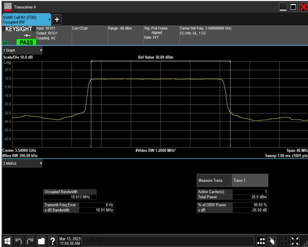
n77(3450-3550) SCS=15kHz DFT_QPSK BW=20MHz Channel=636000 RB=100@0
