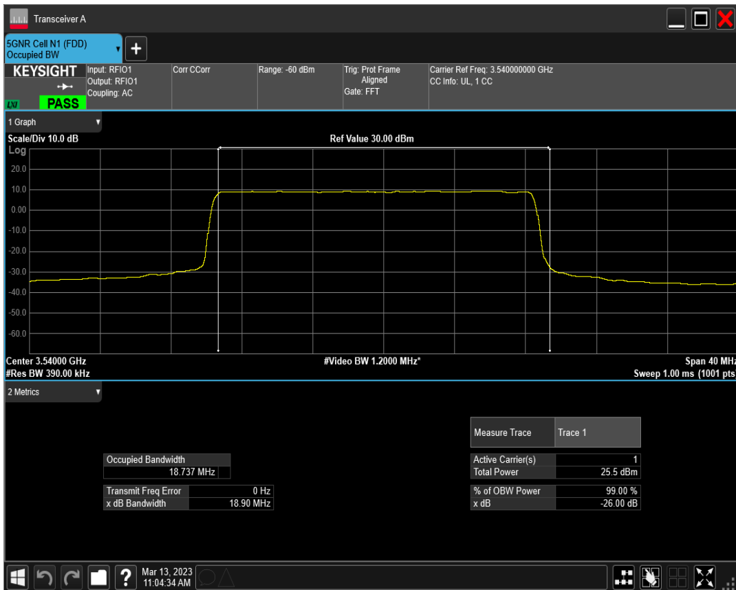
n77(3450-3550) SCS=15kHz DFT_QAM16 BW=20MHz Channel=636000 RB=100@0
