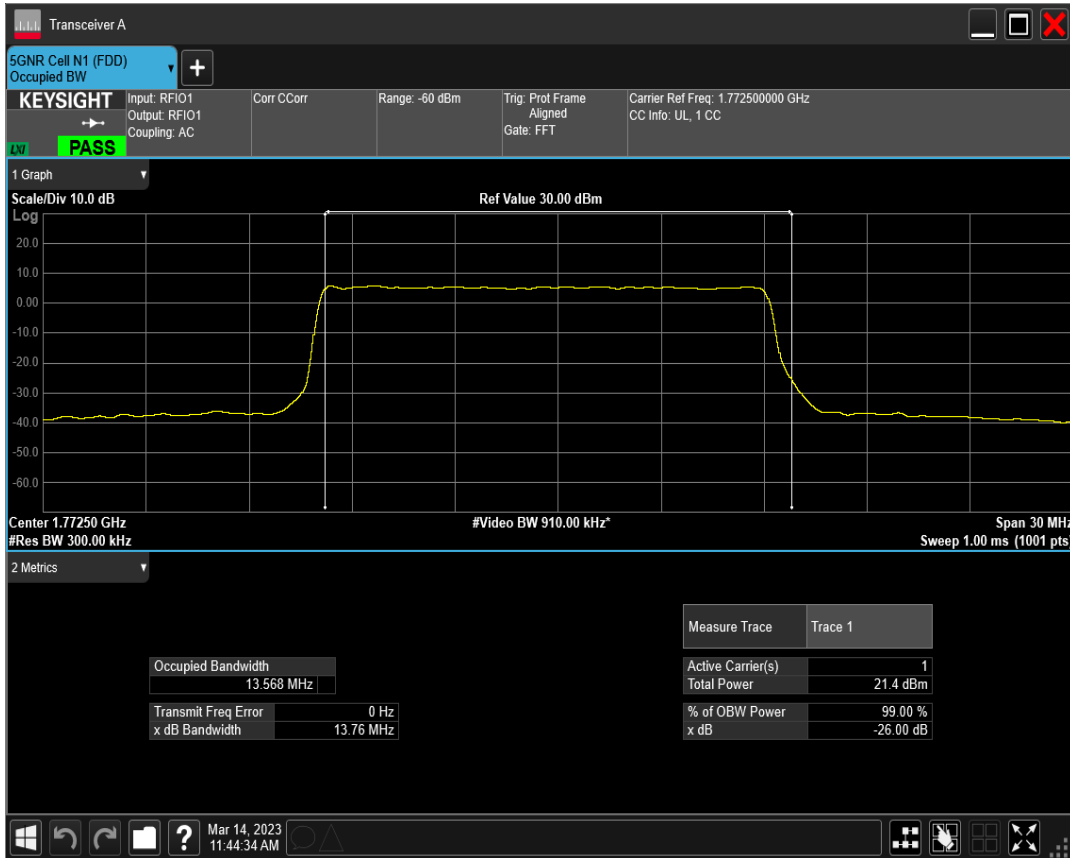
n66 SCS=30kHz DFT_QAM64 BW=15MHz Channel=354500 RB=36@0
