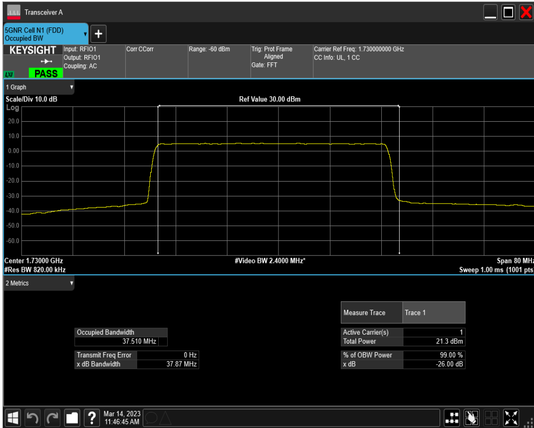
n66 SCS=30kHz DFT_QAM64 BW=40MHz Channel=346000 RB=100@0
