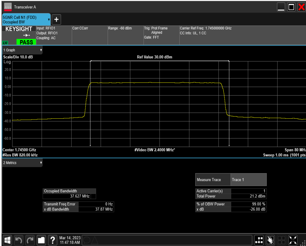
n66 SCS=30kHz DFT_QAM64 BW=40MHz Channel=349000 RB=100@0
