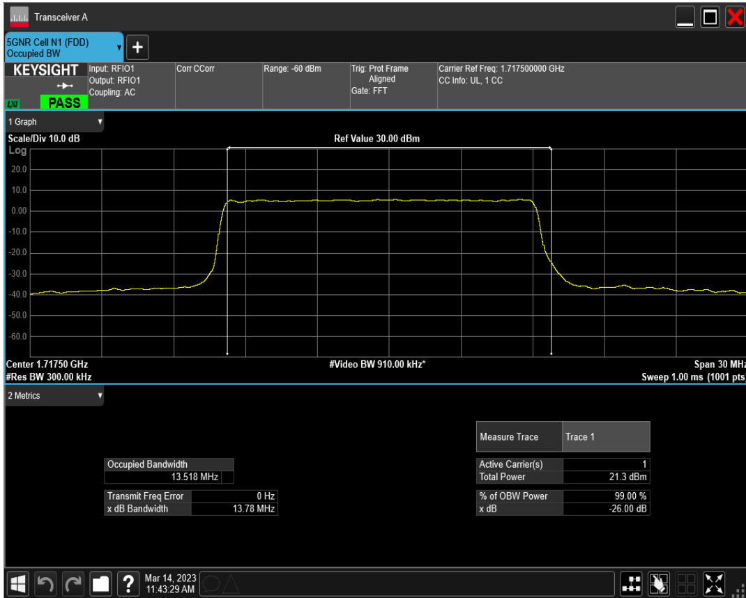
n66 SCS=30kHz DFT_QAM64 BW=15MHz Channel=343500 RB=36@0
