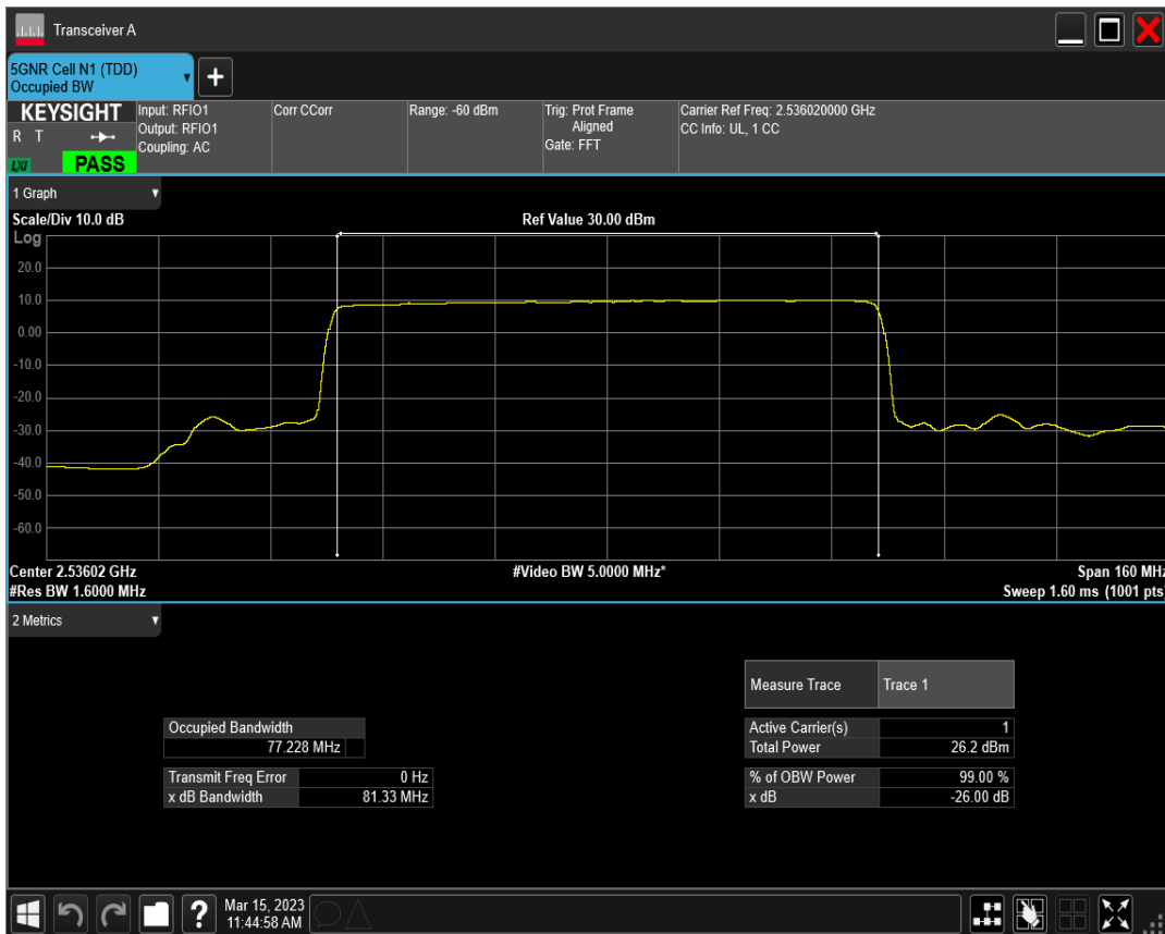
n41 SCS=30kHz DFT_QPSK BW=80MHz Channel=507204 RB=216@0
