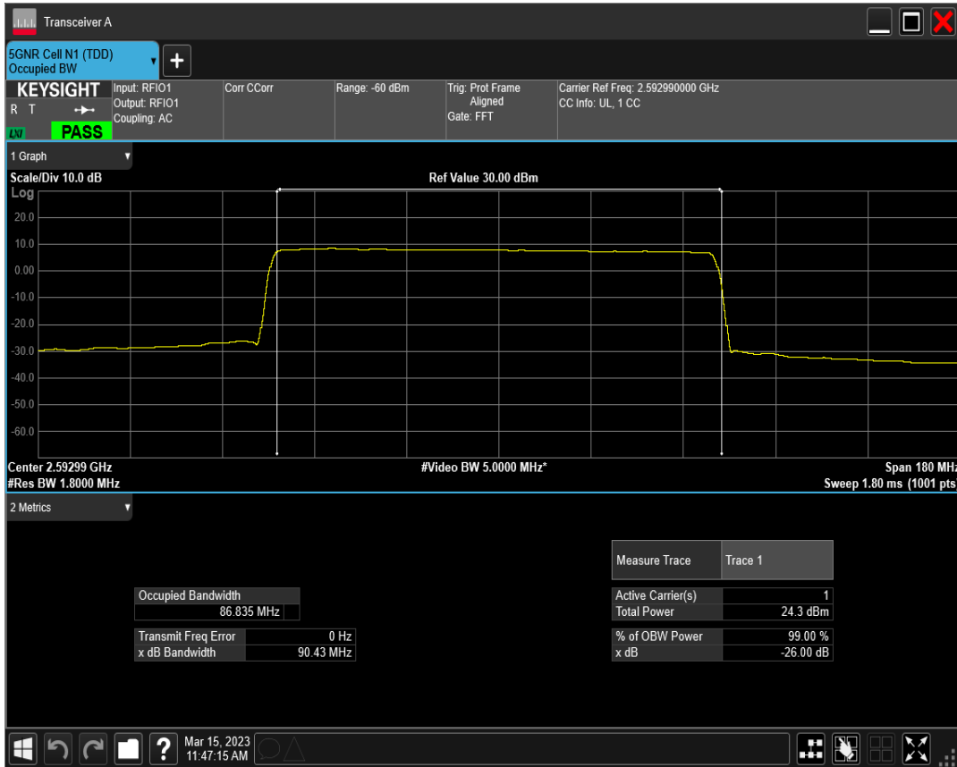
n41 SCS=30kHz DFT_QAM256 BW=90MHz Channel=518598 RB=240@0
