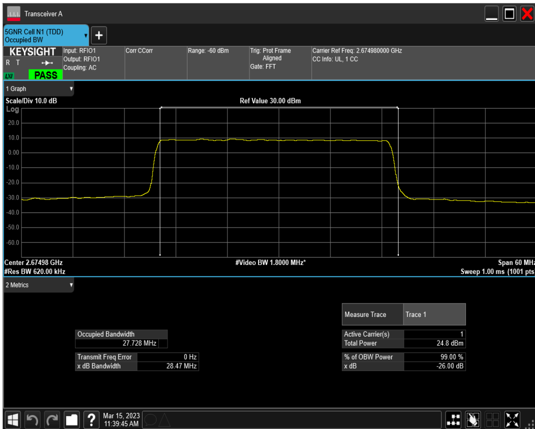
n41 SCS=30kHz DFT_QAM64 BW=30MHz Channel=534996 RB=75@0
