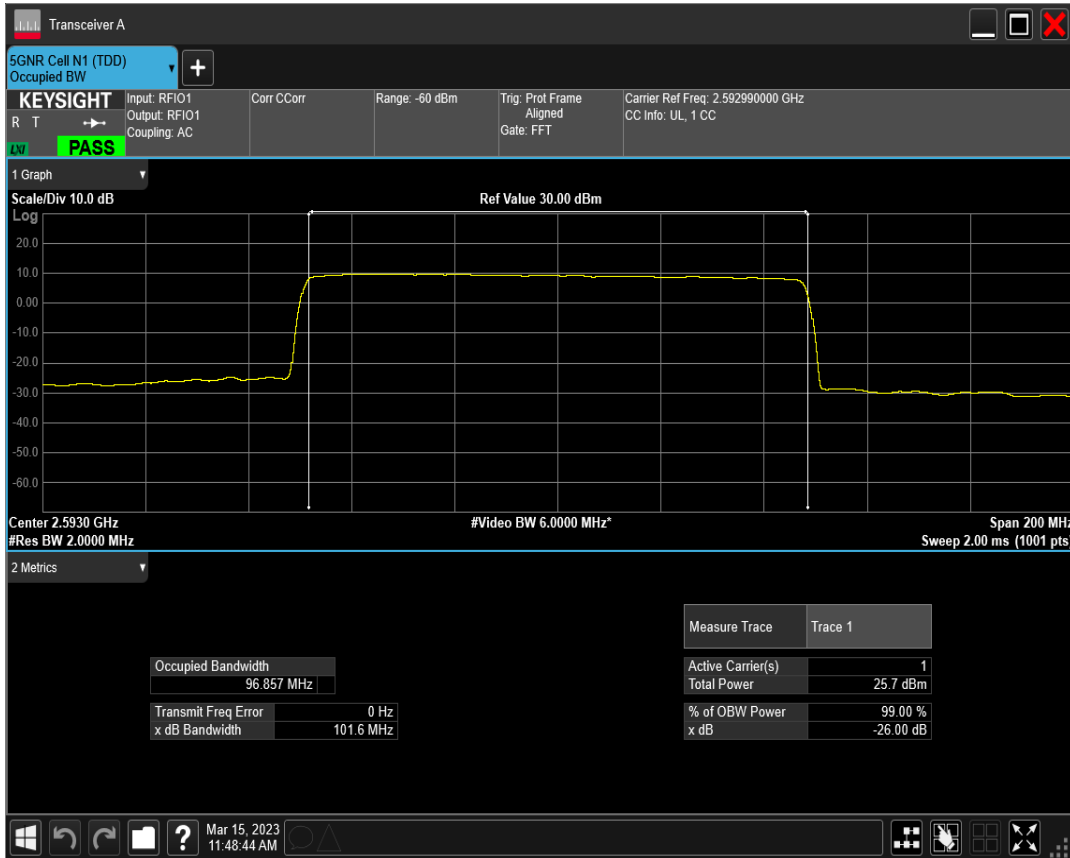
n41 SCS=30kHz DFT_QAM16 BW=100MHz Channel=518598 RB=270@0
