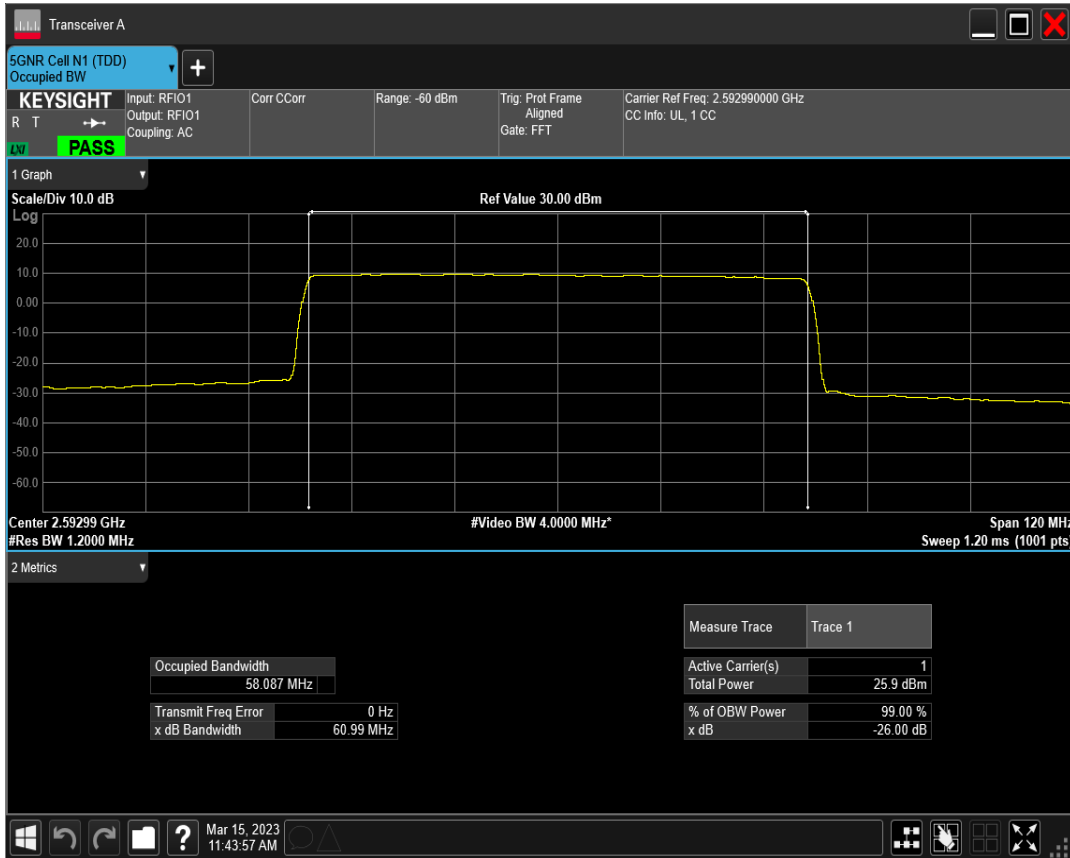
n41 SCS=30kHz DFT_QAM16 BW=60MHz Channel=518598 RB=162@0
