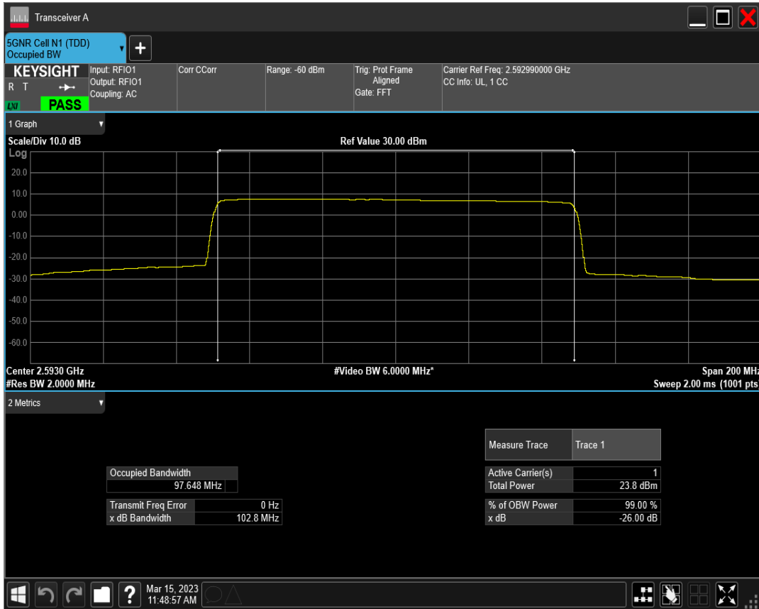
n41 SCS=30kHz DFT_BPSK BW=100MHz Channel=528000 RB=270@0
