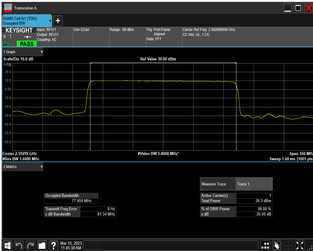
n41 SCS=30kHz DFT_QPSK BW=80MHz Channel=518598 RB=216@0
