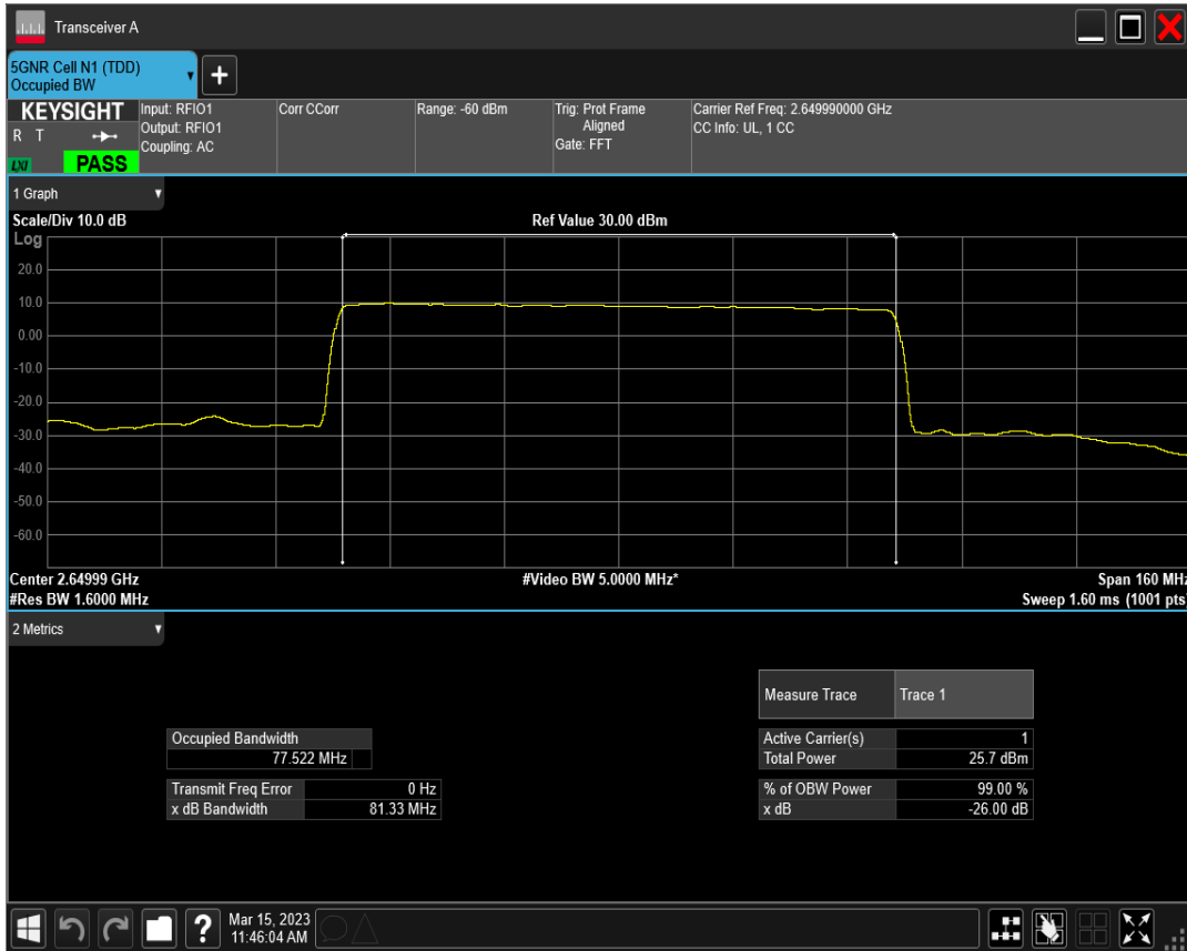
n41 SCS=30kHz DFT_QAM16 BW=80MHz Channel=529998 RB=216@0
