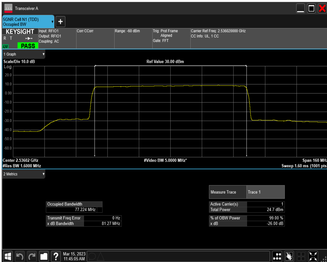
n41 SCS=30kHz DFT_QAM64 BW=80MHz Channel=507204 RB=216@0
