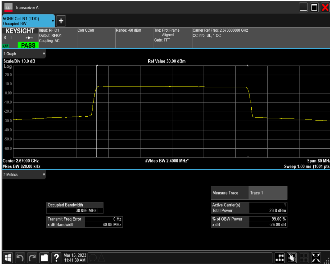
n41 SCS=30kHz DFT_BPSK BW=50MHz Channel=504204 RB=128@0
