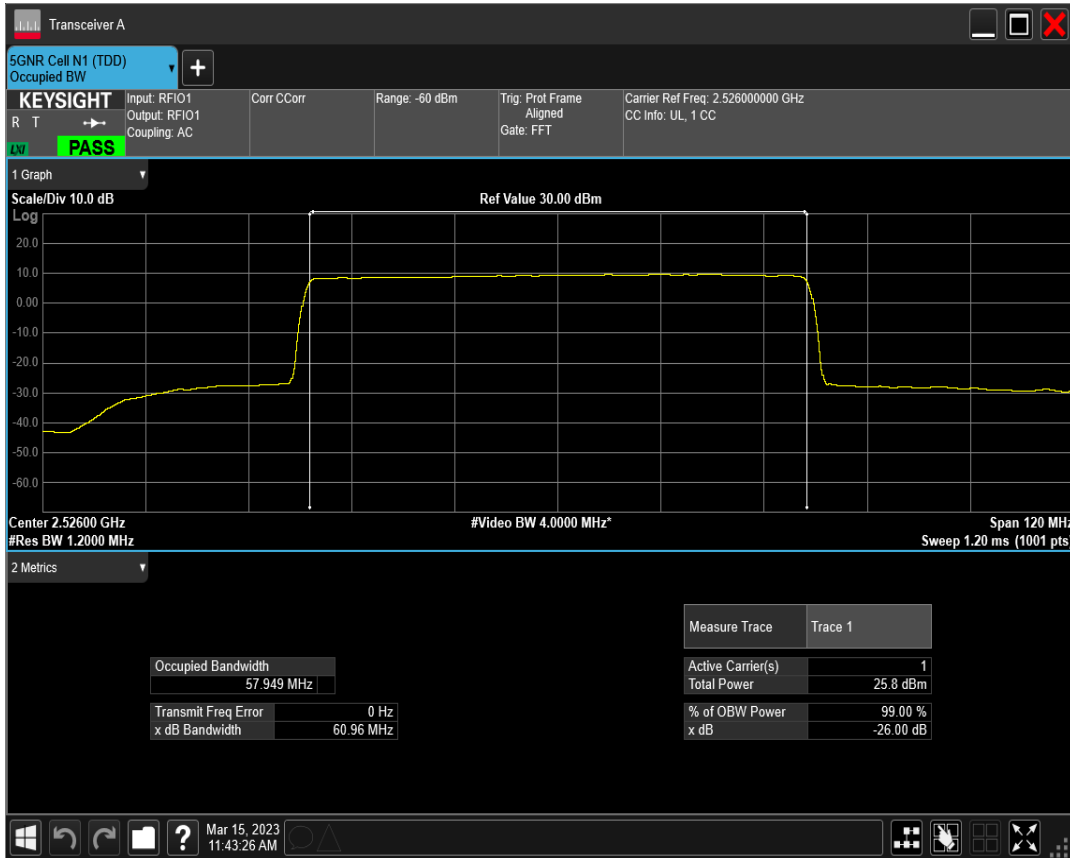
n41 SCS=30kHz DFT_QAM16 BW=60MHz Channel=505200 RB=162@0
