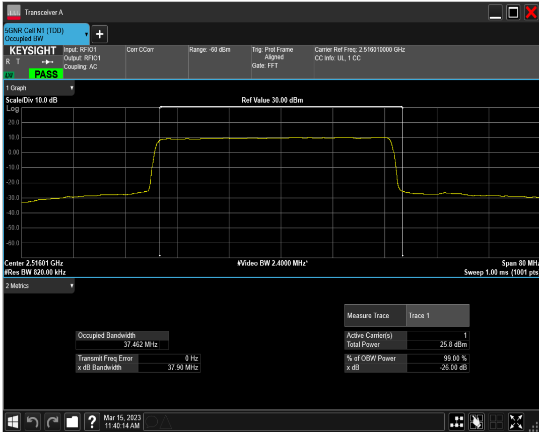
n41 SCS=30kHz DFT_QAM16 BW=40MHz Channel=503202 RB=100@0
