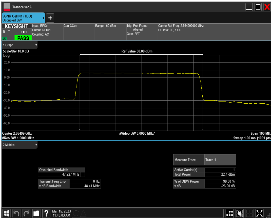
n41 SCS=30kHz CP_QPSK BW=50MHz Channel=532998 RB=133@0
