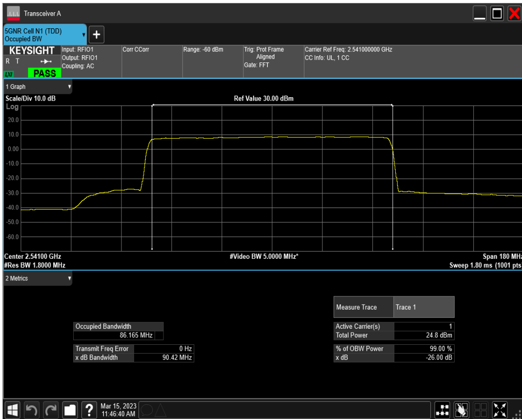
n41 SCS=30kHz DFT_QAM64 BW=90MHz Channel=508200 RB=240@0
