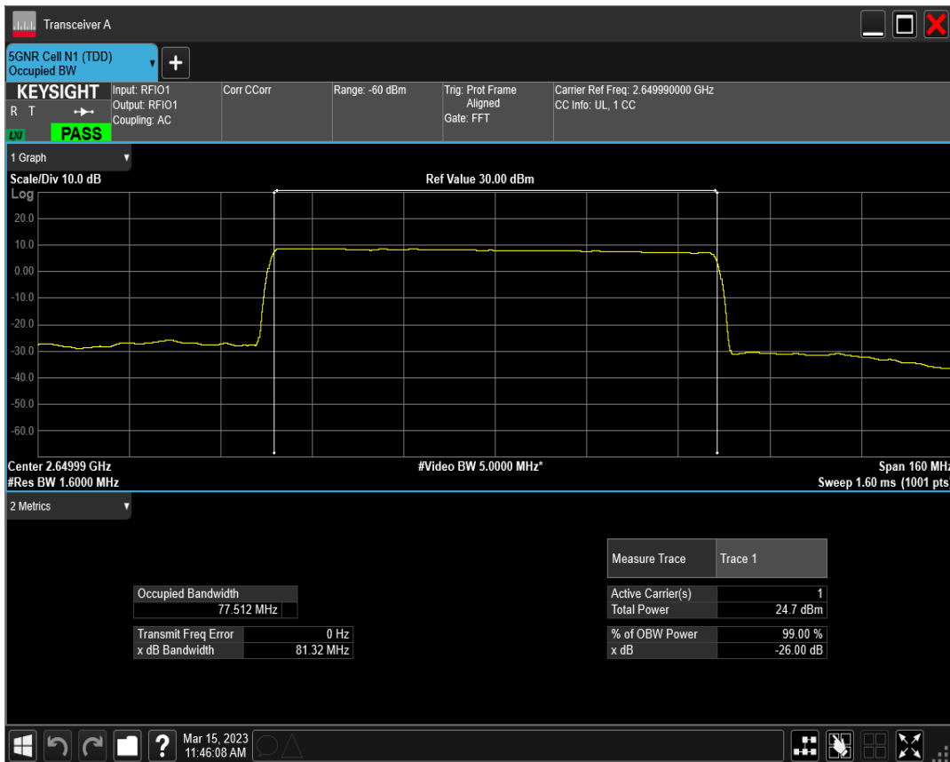
n41 SCS=30kHz DFT_QAM64 BW=80MHz Channel=529998 RB=216@0
