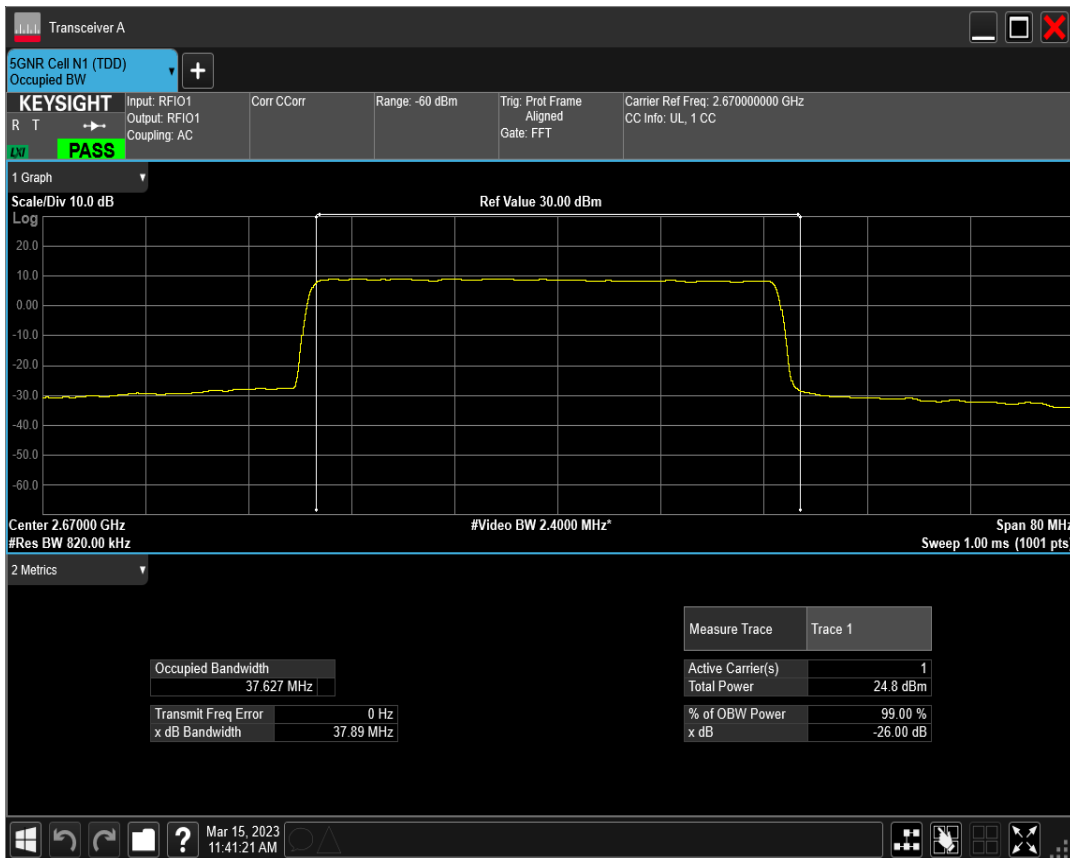
n41 SCS=30kHz DFT_QAM64 BW=40MHz Channel=534000 RB=100@0
