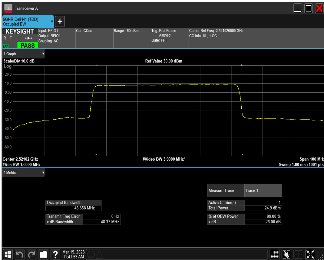
n41 SCS=30kHz DFT_QAM64 BW=50MHz Channel=504204 RB=128@0
