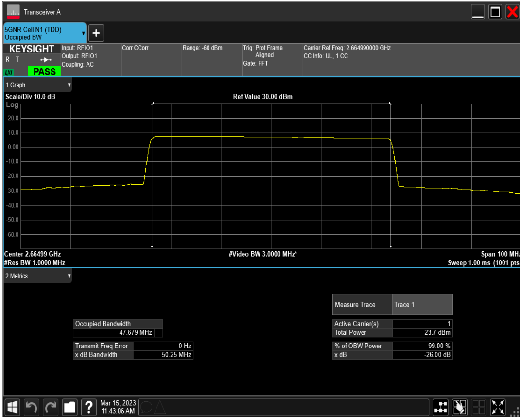
n41 SCS=30kHz DFT_BPSK BW=60MHz Channel=505200 RB=162@0
