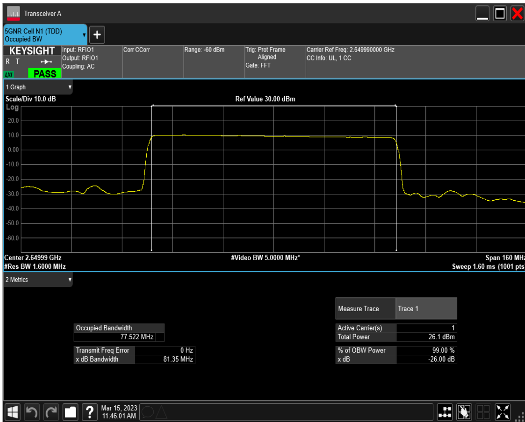
n41 SCS=30kHz DFT_QPSK BW=80MHz Channel=529998 RB=216@0
