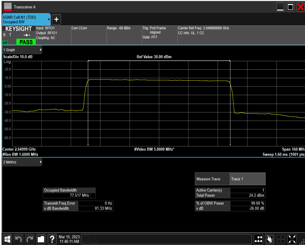
n41 SCS=30kHz DFT_QAM256 BW=80MHz Channel=529998 RB=216@0
