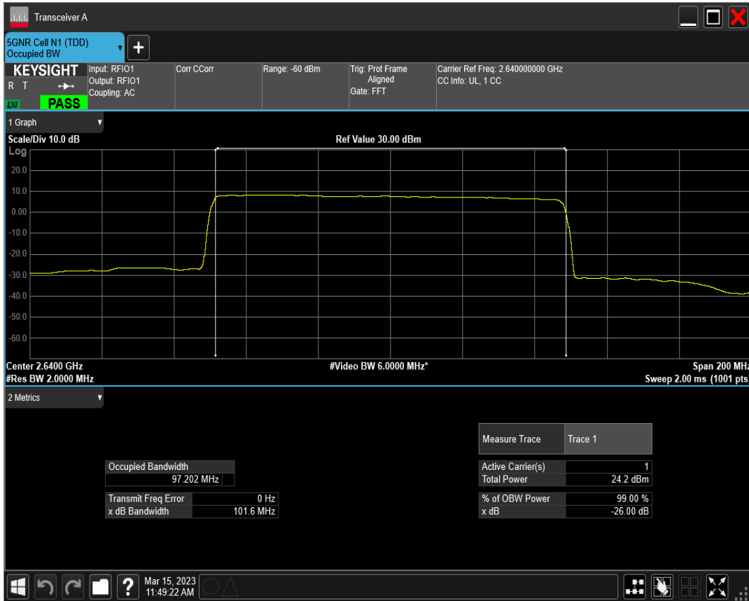
n41 SCS=30kHz DFT_QAM256 BW=100MHz Channel=528000 RB=270@0
