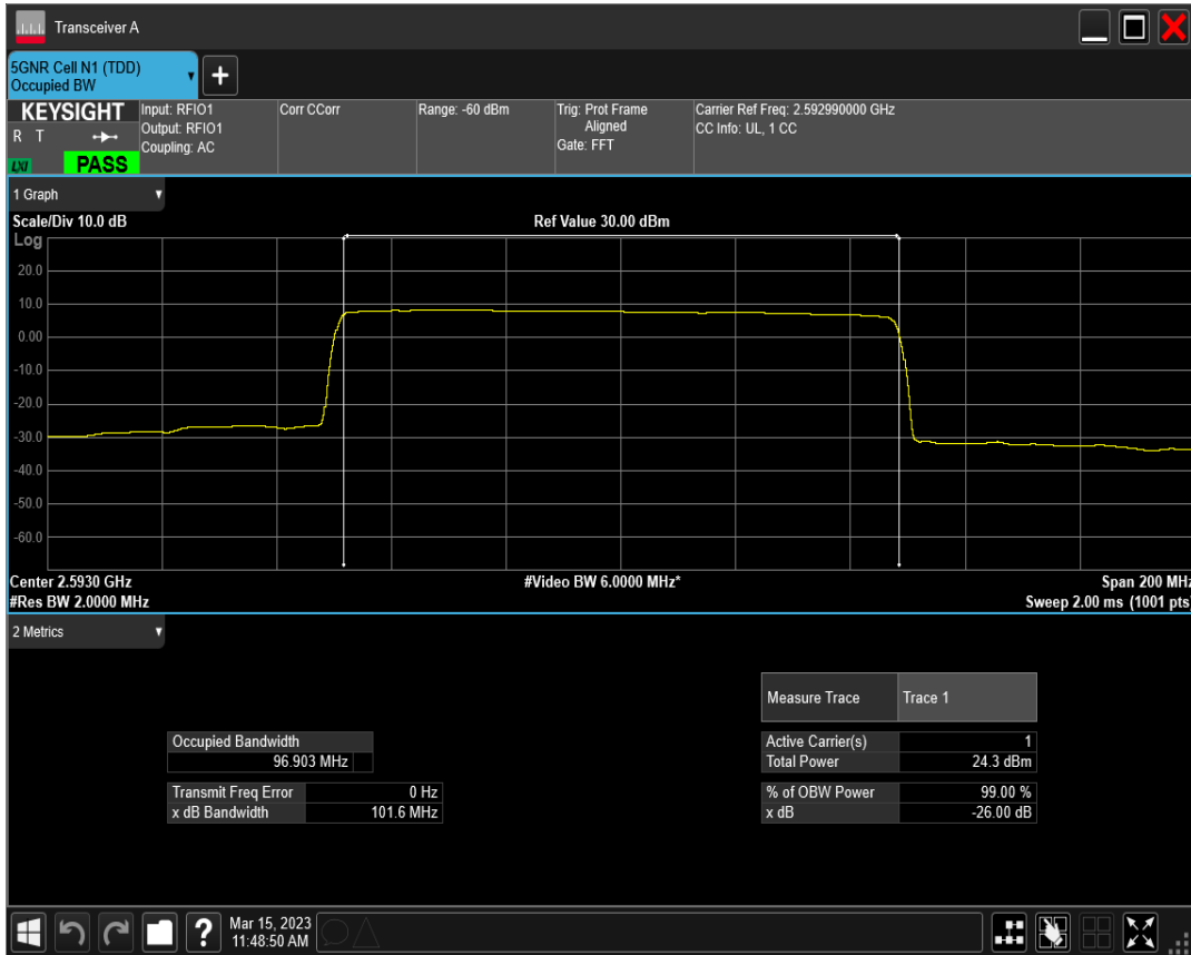
n41 SCS=30kHz DFT_QAM256 BW=100MHz Channel=518598 RB=270@0
