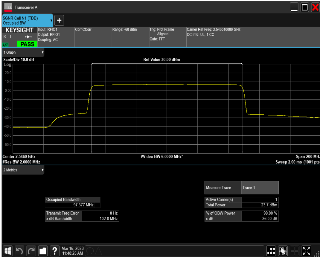
n41 SCS=30kHz DFT_BPSK BW=100MHz Channel=518598 RB=270@0
