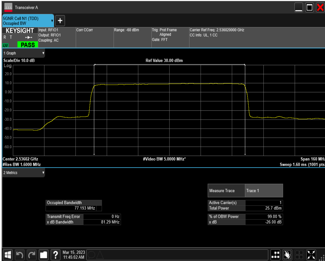
n41 SCS=30kHz DFT_QAM16 BW=80MHz Channel=507204 RB=216@0
