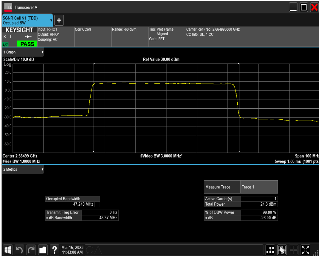
n41 SCS=30kHz DFT_QAM256 BW=50MHz Channel=532998 RB=128@0
