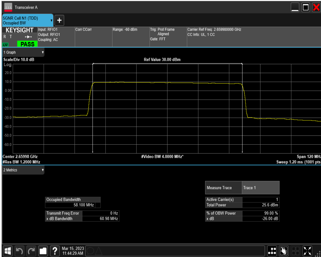
n41 SCS=30kHz DFT_QAM16 BW=60MHz Channel=531996 RB=162@0
