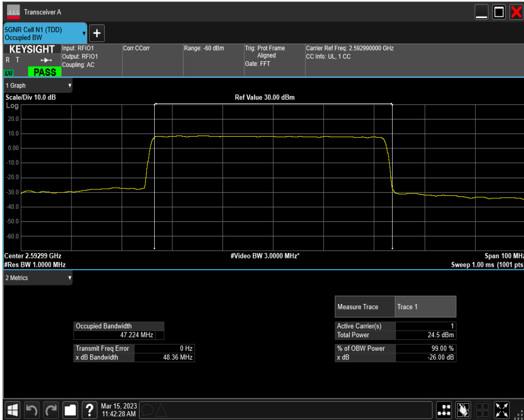
n41 SCS=30kHz DFT_QAM256 BW=50MHz Channel=518598 RB=128@0
