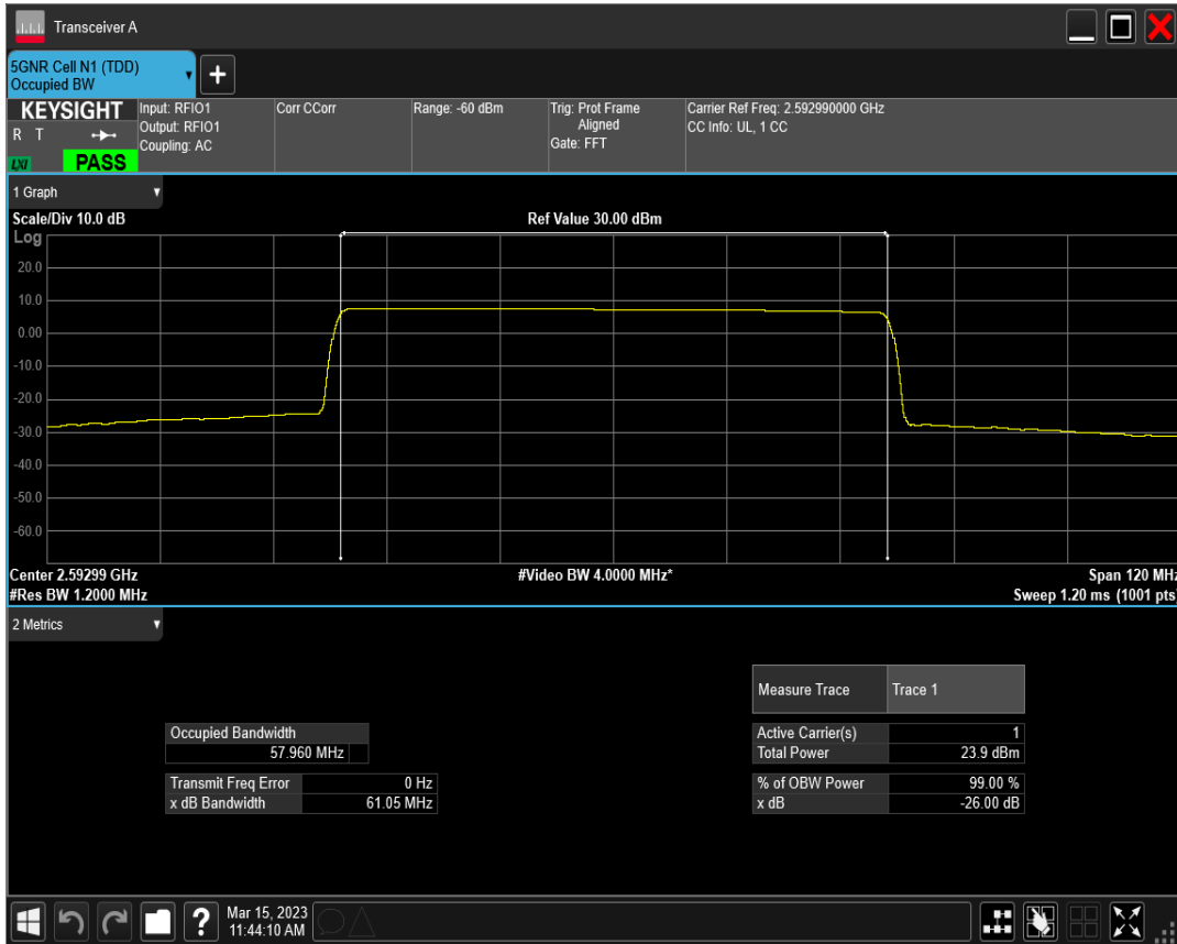
n41 SCS=30kHz DFT_BPSK BW=60MHz Channel=531996 RB=162@0
