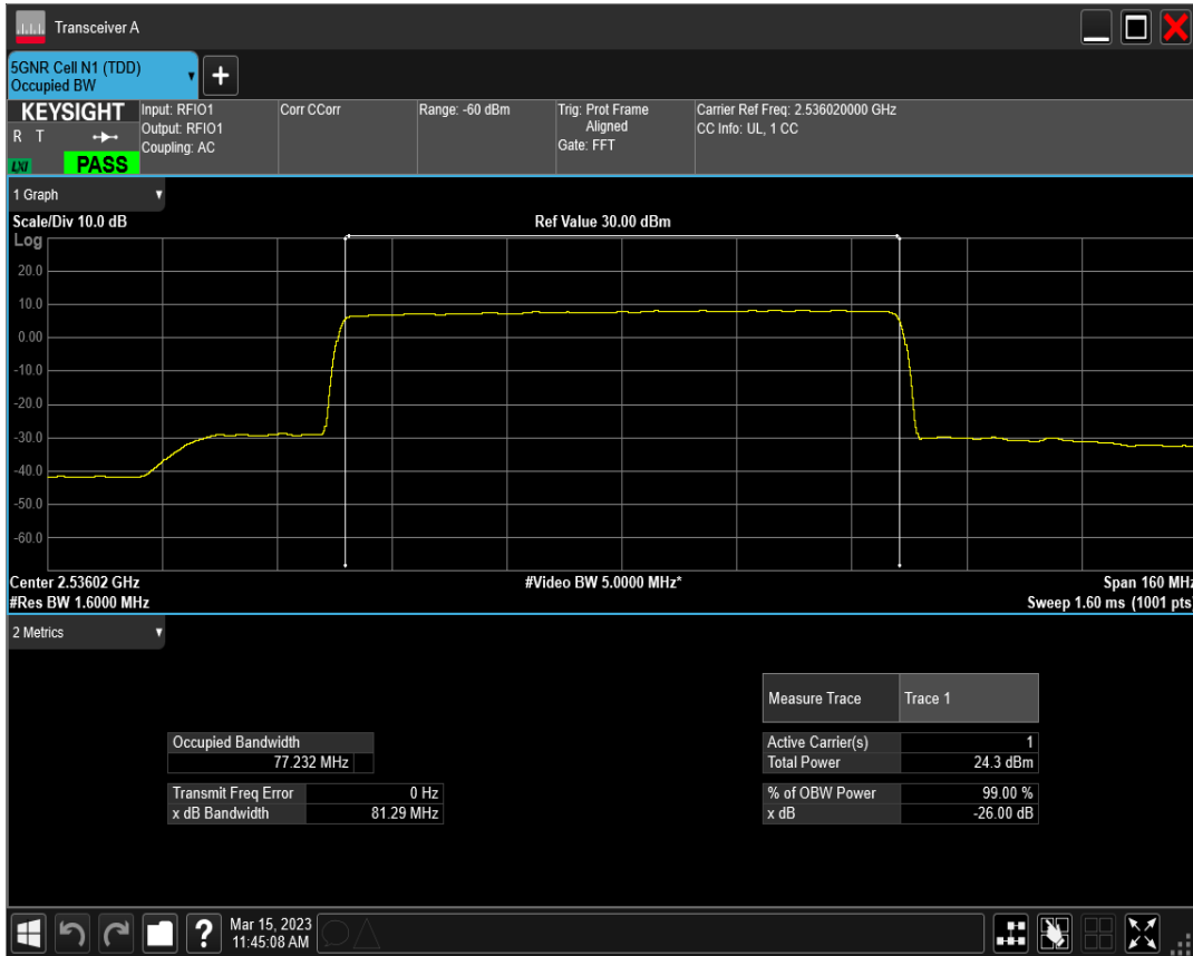
n41 SCS=30kHz DFT_QAM256 BW=80MHz Channel=507204 RB=216@0
