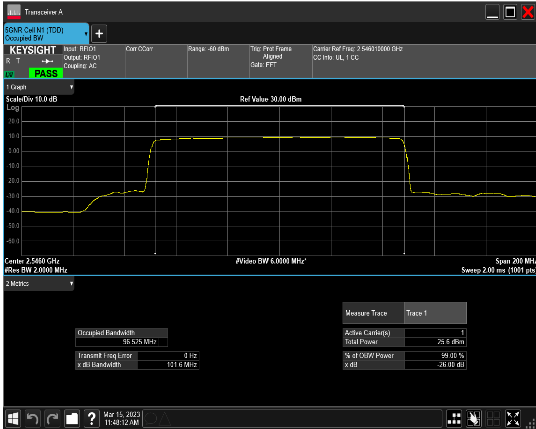
n41 SCS=30kHz DFT_QAM16 BW=100MHz Channel=509202 RB=270@0
