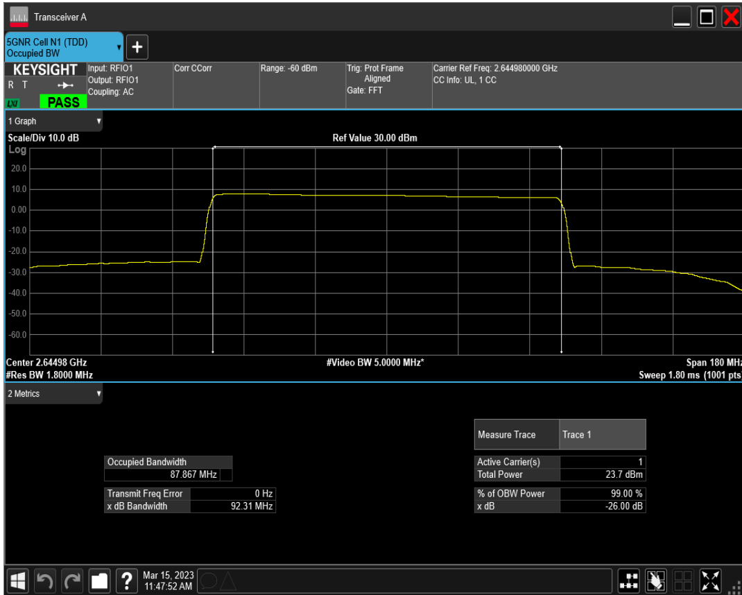
n41 SCS=30kHz DFT_BPSK BW=100MHz Channel=509202 RB=270@0
