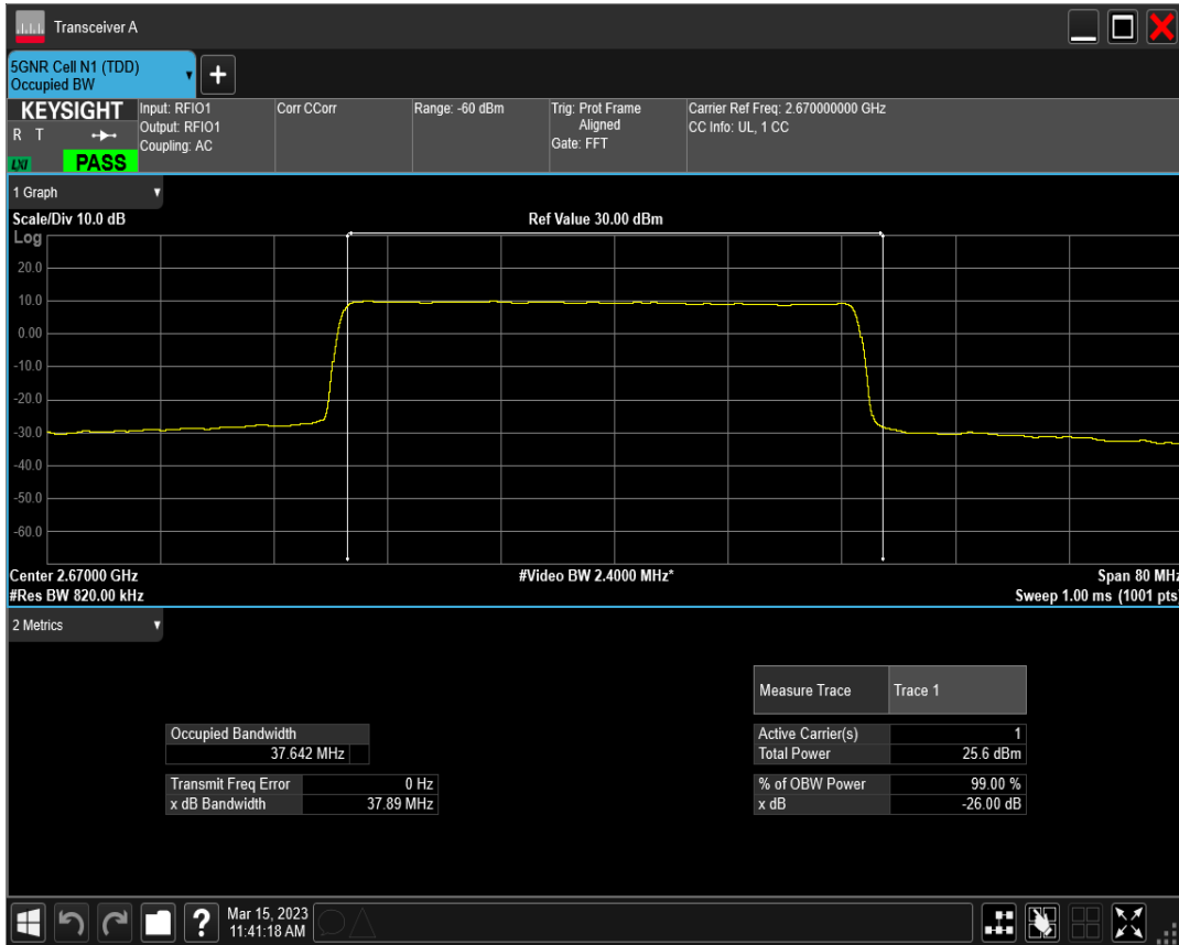
n41 SCS=30kHz DFT_QAM16 BW=40MHz Channel=534000 RB=100@0
