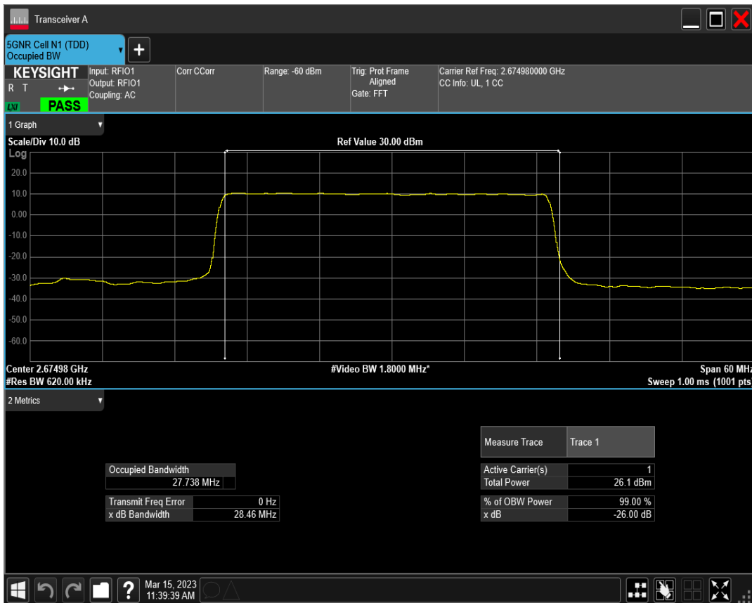
n41 SCS=30kHz DFT_QPSK BW=30MHz Channel=534996 RB=75@0
