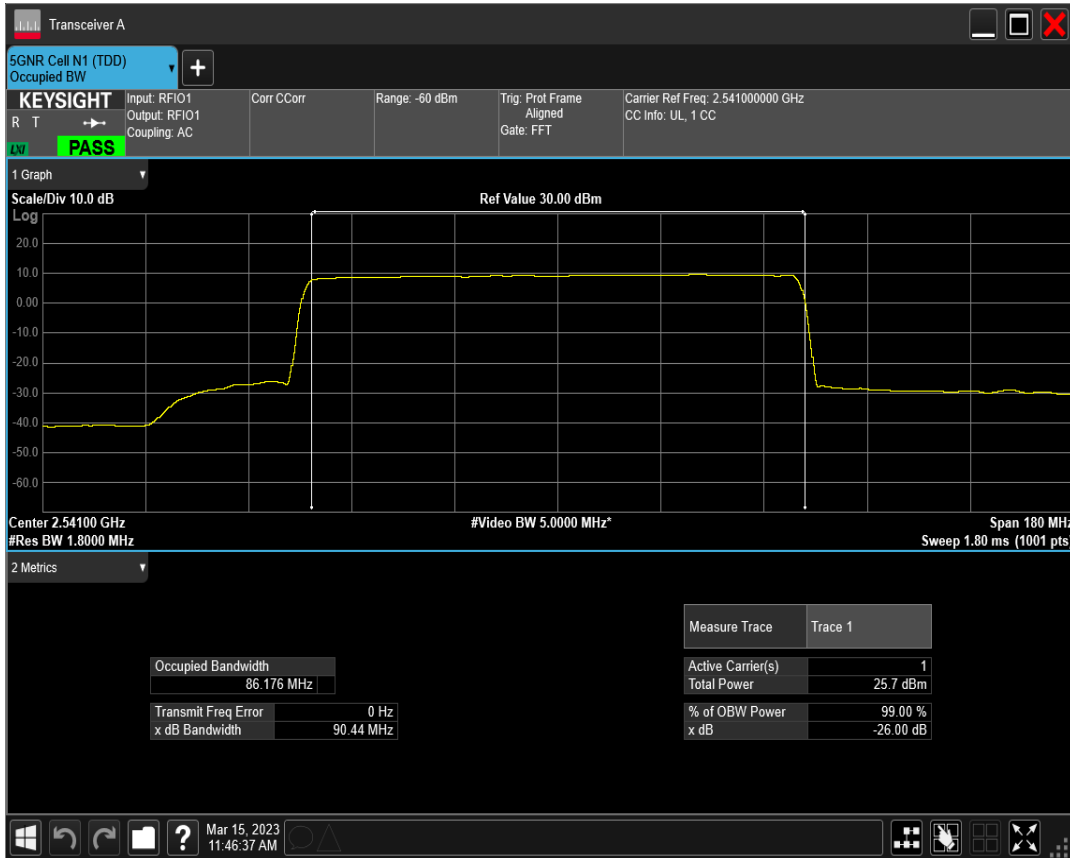
n41 SCS=30kHz DFT_QAM16 BW=90MHz Channel=508200 RB=240@0
