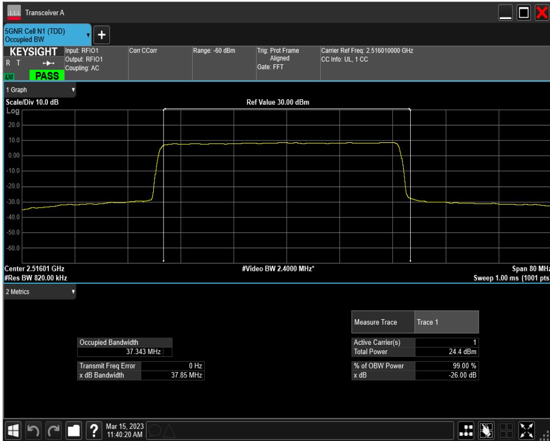
n41 SCS=30kHz DFT_QAM256 BW=40MHz Channel=503202 RB=100@0
