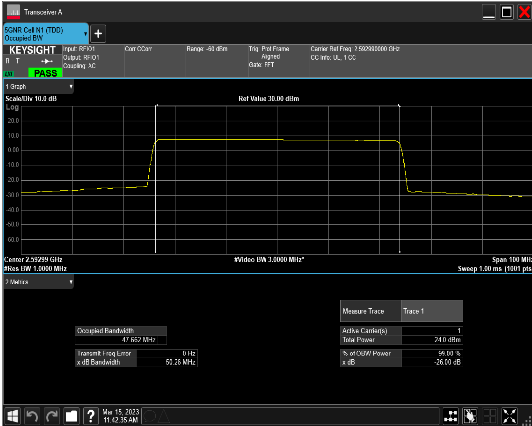
n41 SCS=30kHz DFT_BPSK BW=50MHz Channel=532998 RB=128@0
