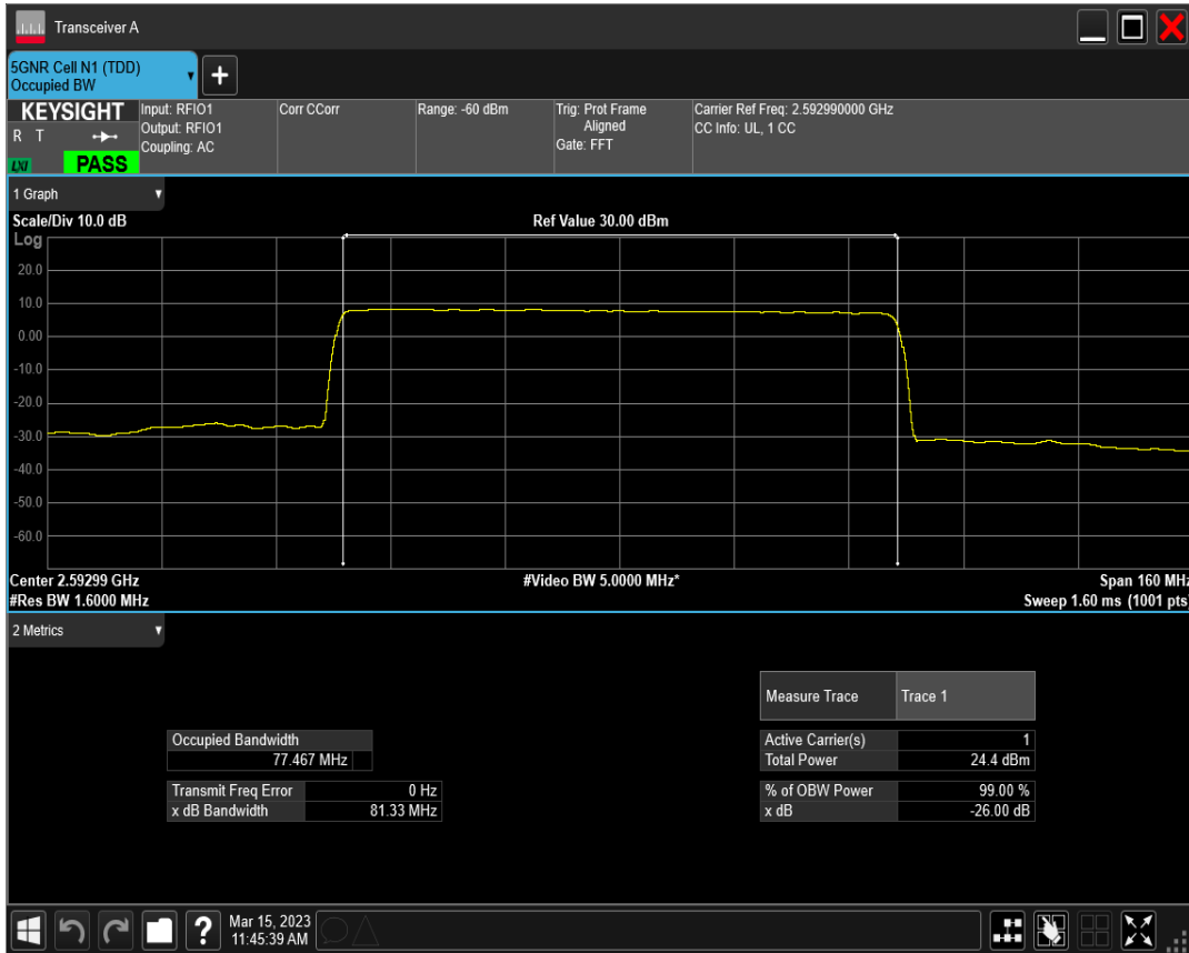
n41 SCS=30kHz DFT_QAM256 BW=80MHz Channel=518598 RB=216@0
