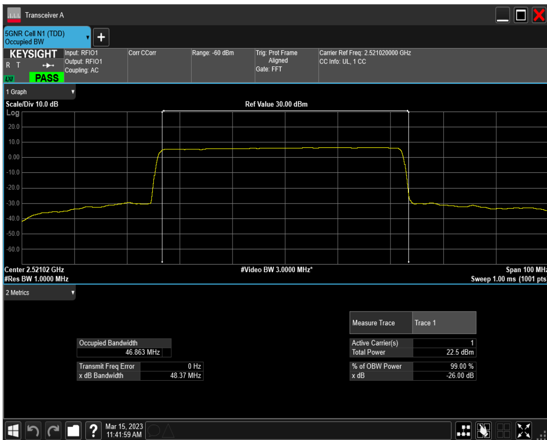
n41 SCS=30kHz CP_QPSK BW=50MHz Channel=504204 RB=133@0
