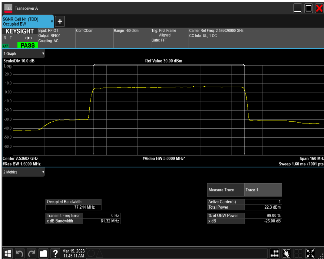
n41 SCS=30kHz CP_QPSK BW=80MHz Channel=507204 RB=217@0
