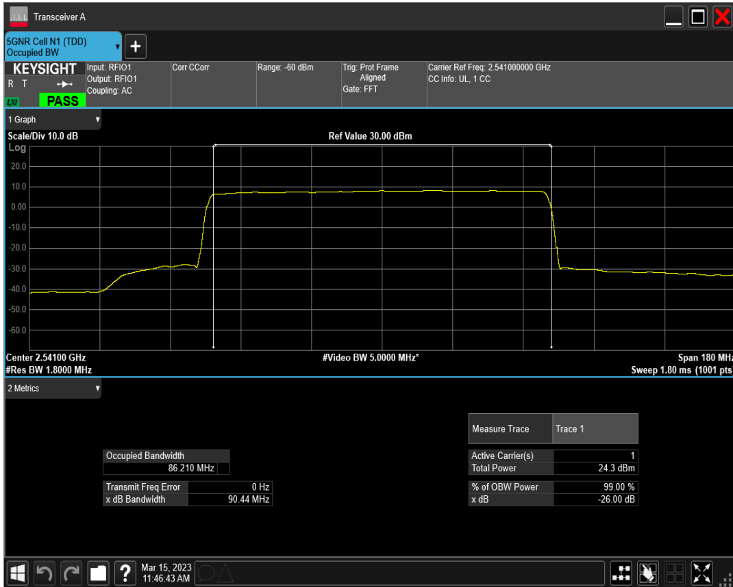
n41 SCS=30kHz DFT_QAM256 BW=90MHz Channel=508200 RB=240@0
