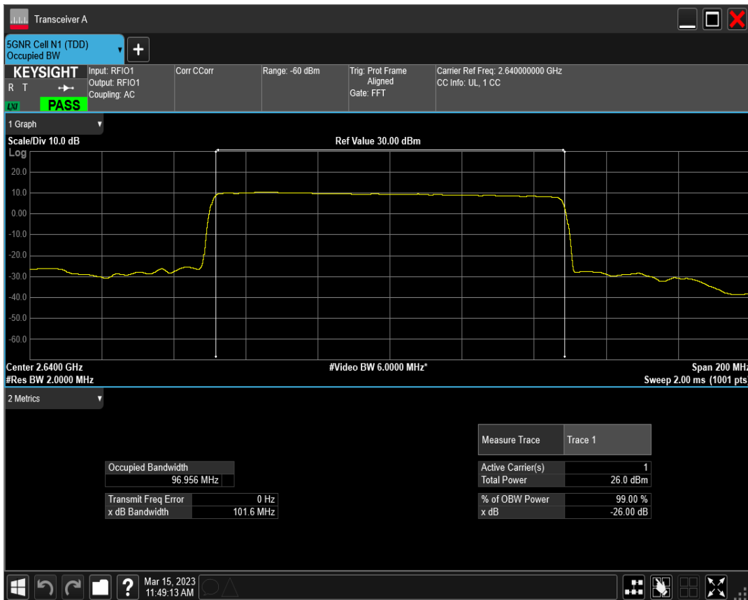
n41 SCS=30kHz DFT_QPSK BW=100MHz Channel=528000 RB=270@0
