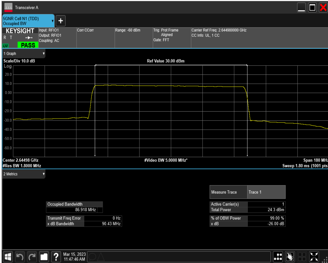
n41 SCS=30kHz DFT_QAM256 BW=90MHz Channel=528996 RB=240@0
