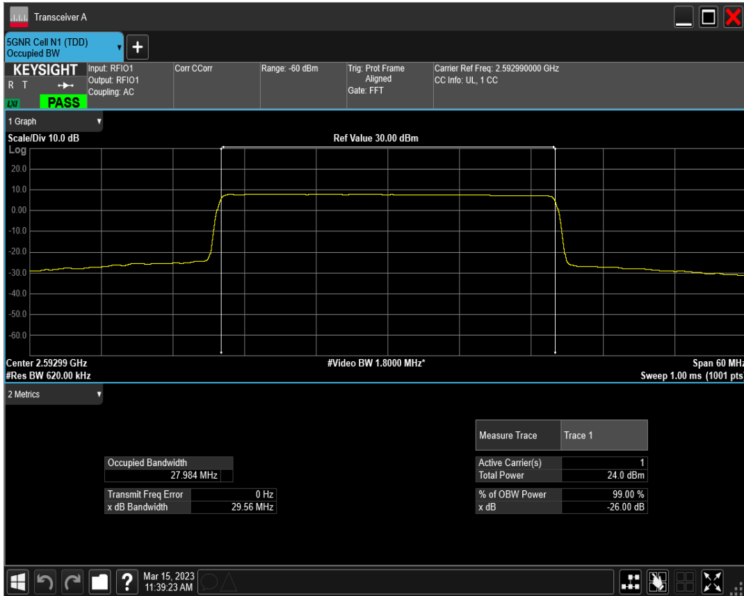
n41 SCS=30kHz DFT_BPSK BW=30MHz Channel=534996 RB=75@0
