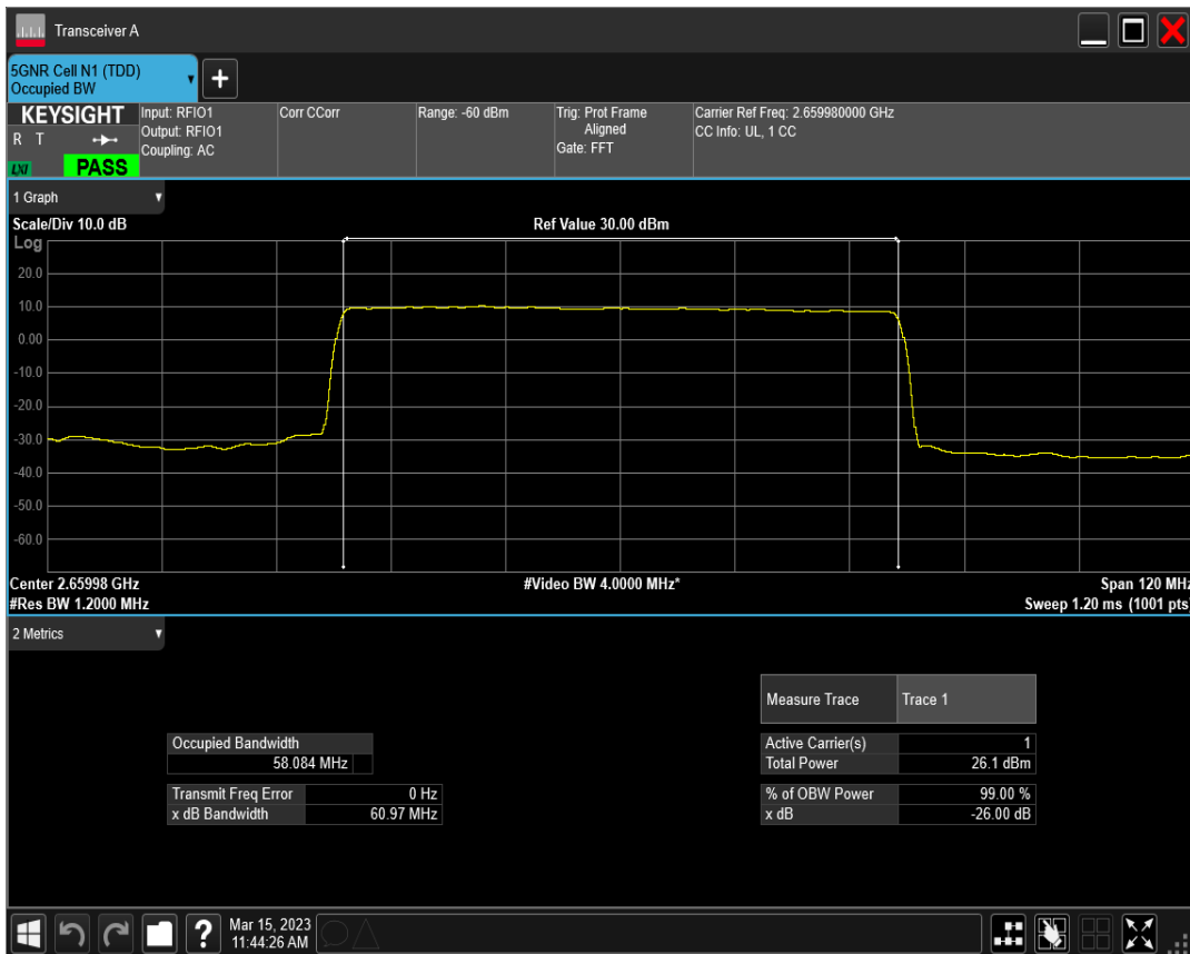
n41 SCS=30kHz DFT_QPSK BW=60MHz Channel=531996 RB=162@0
