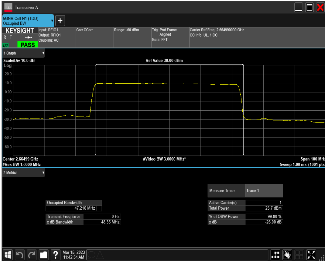
n41 SCS=30kHz DFT_QAM16 BW=50MHz Channel=532998 RB=128@0
