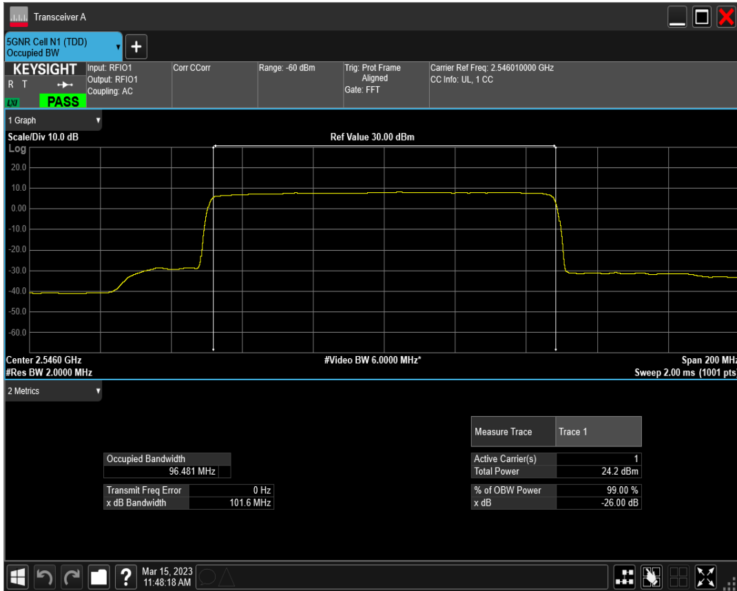
n41 SCS=30kHz DFT_QAM256 BW=100MHz Channel=509202 RB=270@0
