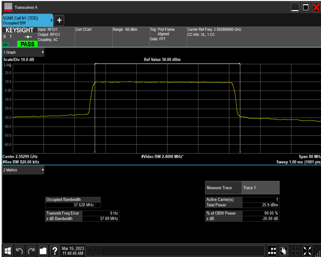
n41 SCS=30kHz DFT_QAM16 BW=40MHz Channel=518598 RB=100@0
