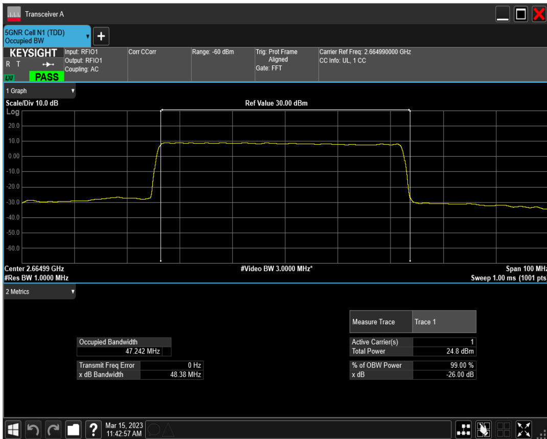
n41 SCS=30kHz DFT_QAM64 BW=50MHz Channel=532998 RB=128@0
