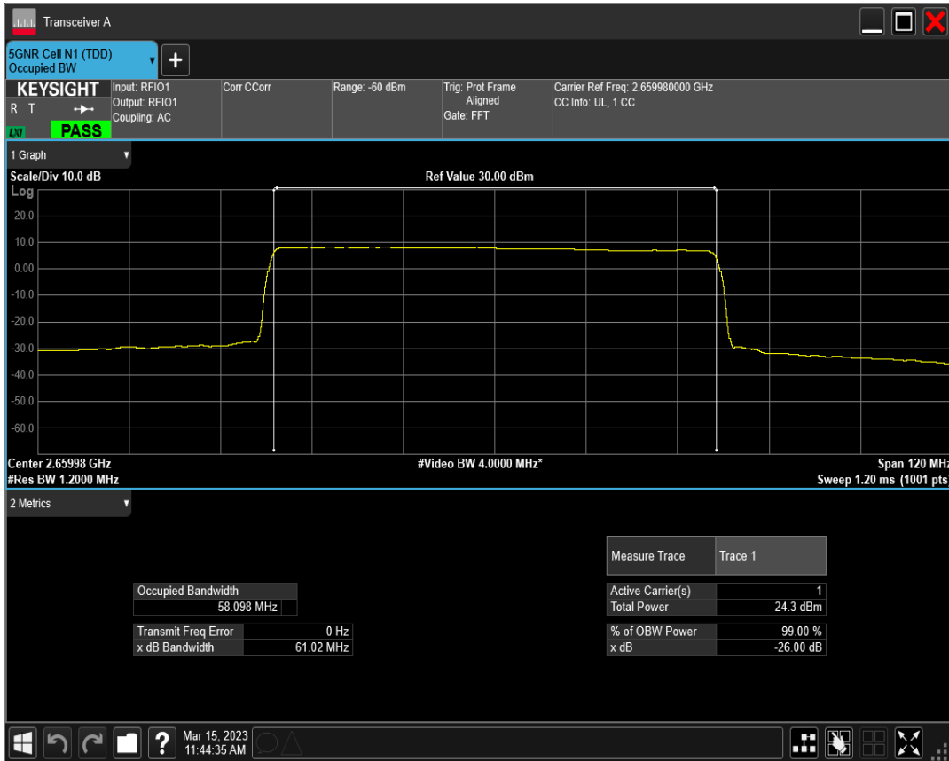
n41 SCS=30kHz DFT_QAM256 BW=60MHz Channel=531996 RB=162@0
