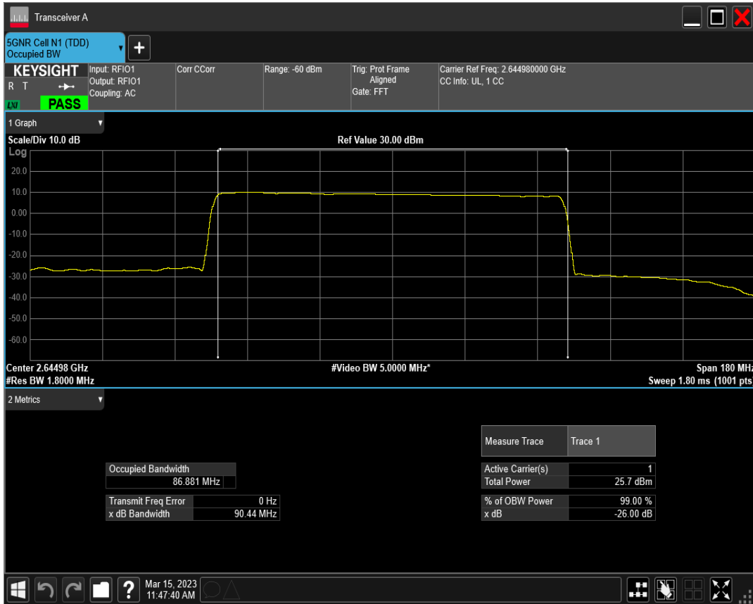
n41 SCS=30kHz DFT_QAM16 BW=90MHz Channel=528996 RB=240@0
