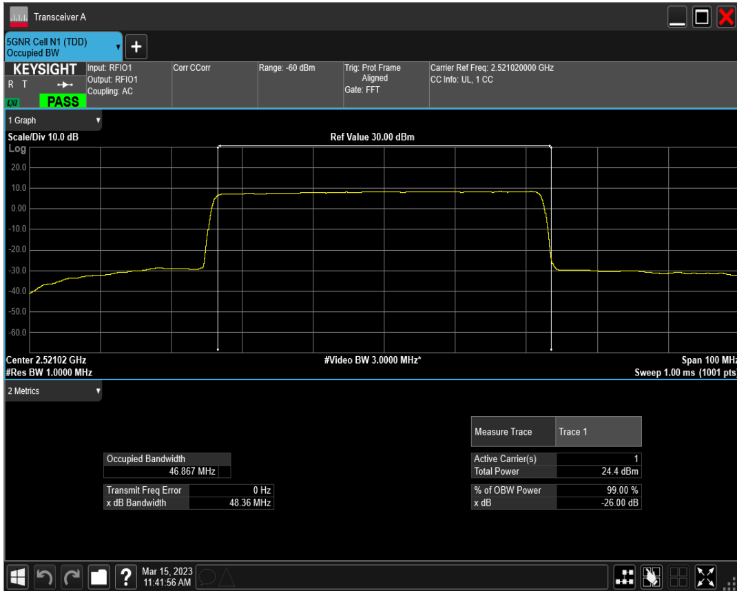
n41 SCS=30kHz DFT_QAM256 BW=50MHz Channel=504204 RB=128@0
