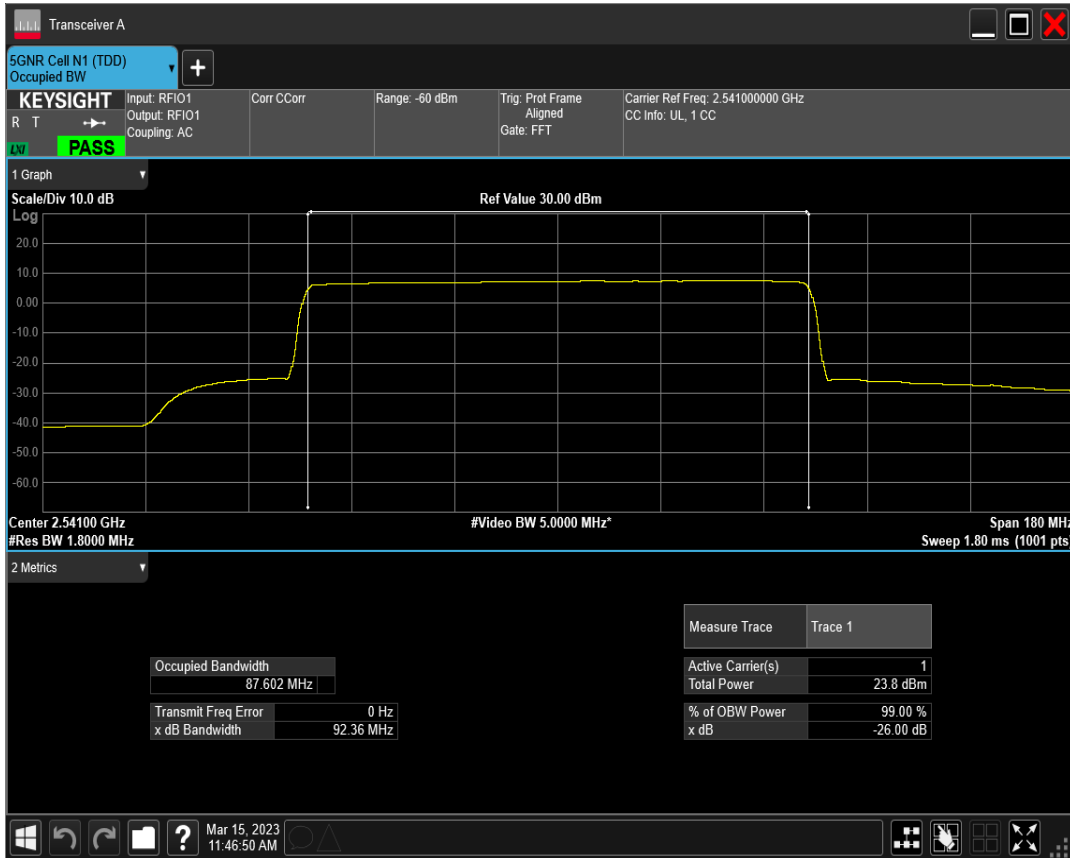
n41 SCS=30kHz DFT_BPSK BW=90MHz Channel=518598 RB=240@0
