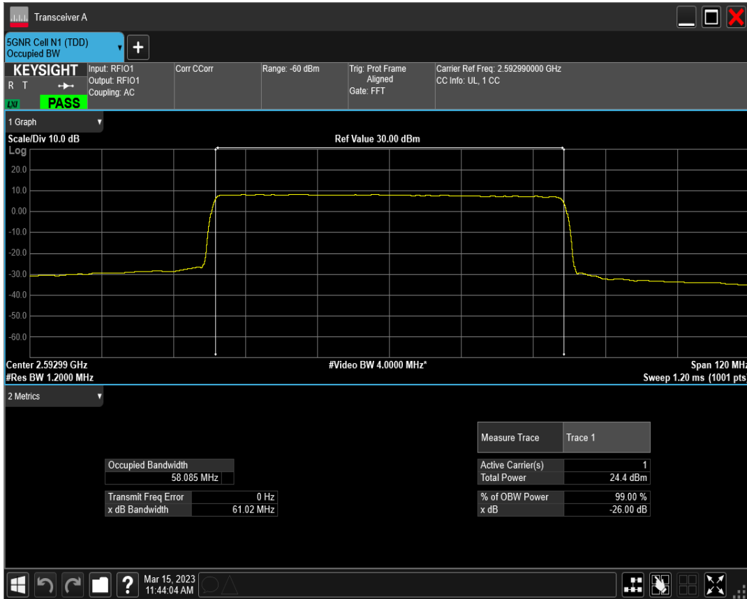
n41 SCS=30kHz DFT_QAM256 BW=60MHz Channel=518598 RB=162@0
