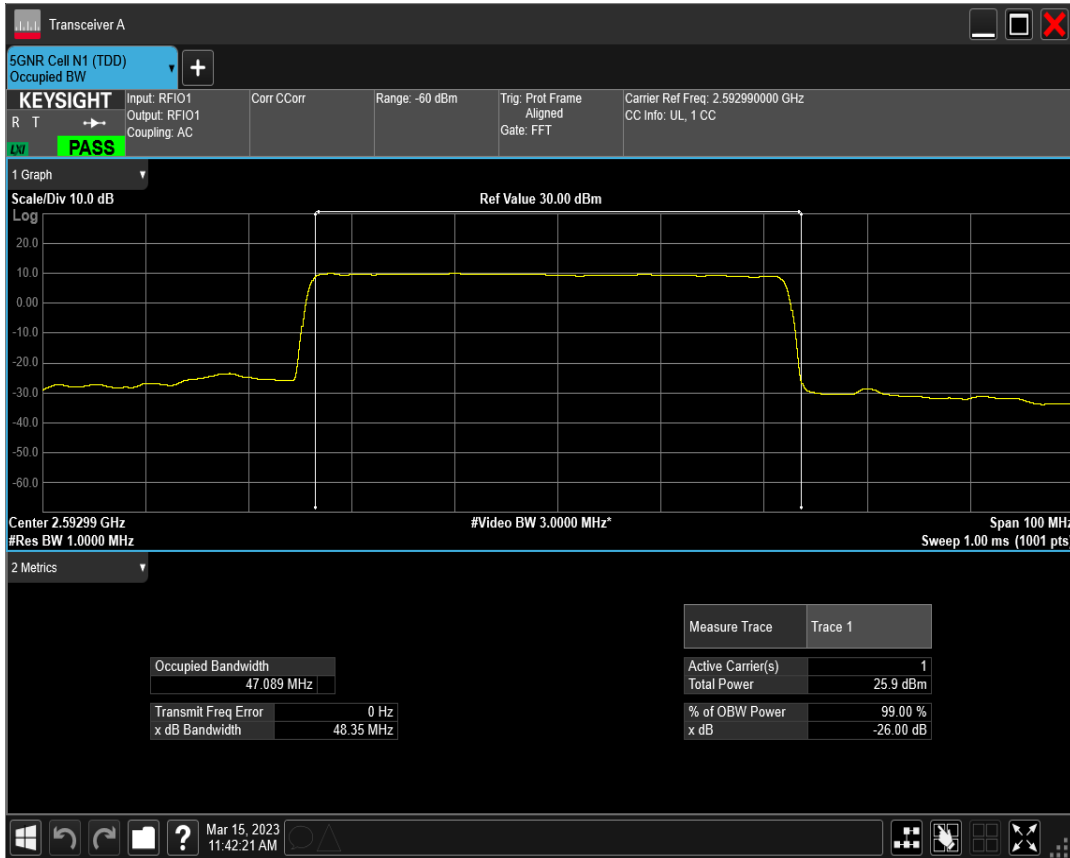
n41 SCS=30kHz DFT_QAM16 BW=50MHz Channel=518598 RB=128@0
