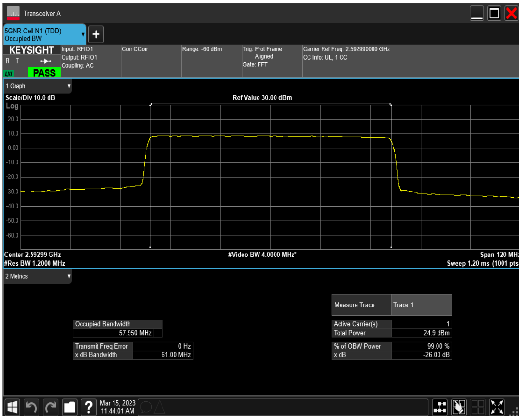
n41 SCS=30kHz DFT_QAM64 BW=60MHz Channel=518598 RB=162@0
