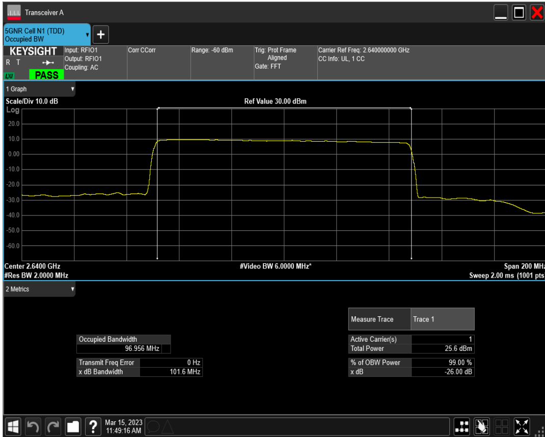
n41 SCS=30kHz DFT_QAM16 BW=100MHz Channel=528000 RB=270@0
