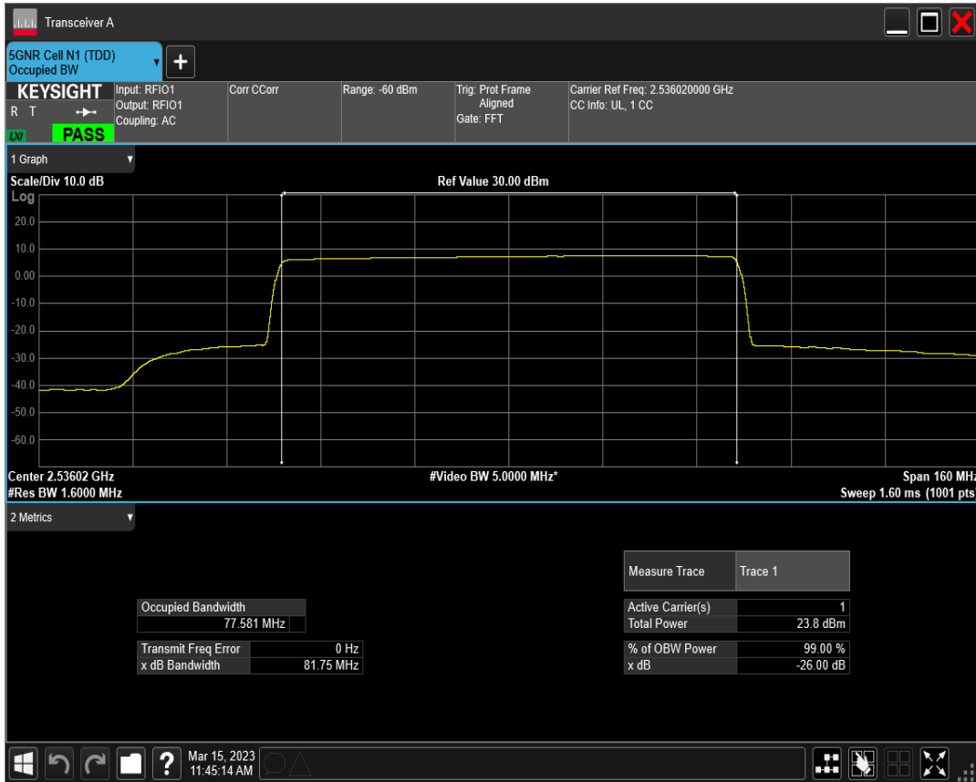
n41 SCS=30kHz DFT_BPSK BW=80MHz Channel=518598 RB=216@0
