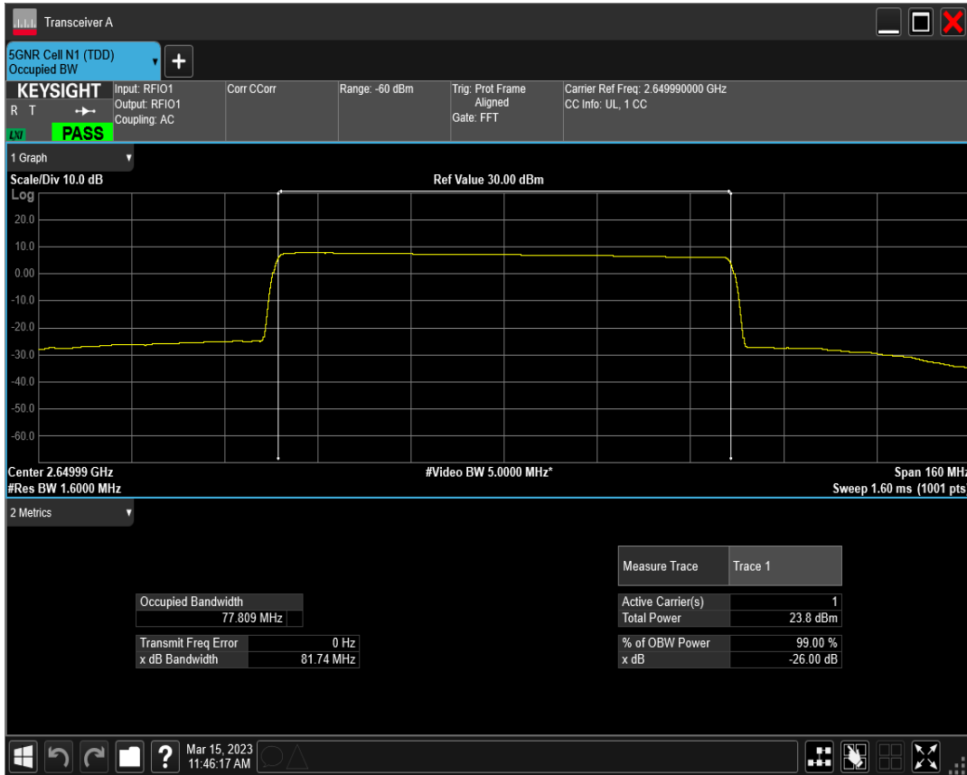
n41 SCS=30kHz DFT_BPSK BW=90MHz Channel=508200 RB=240@0
