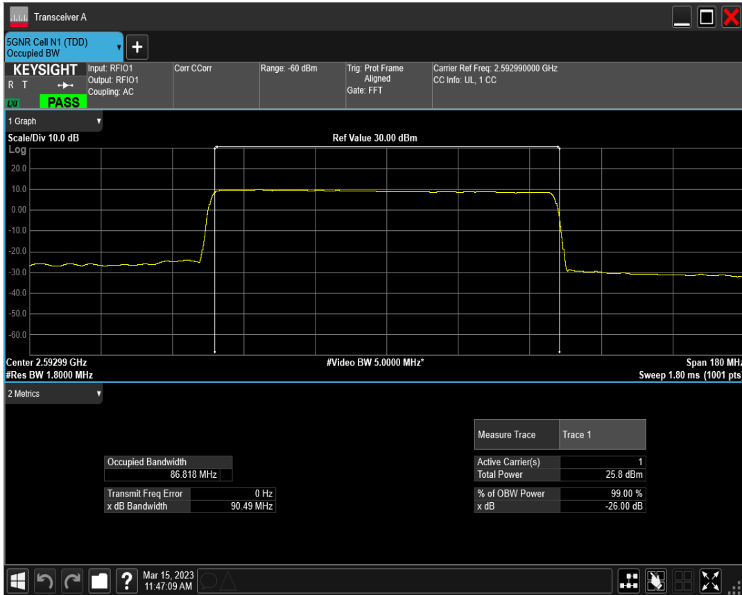
n41 SCS=30kHz DFT_QAM16 BW=90MHz Channel=518598 RB=240@0
