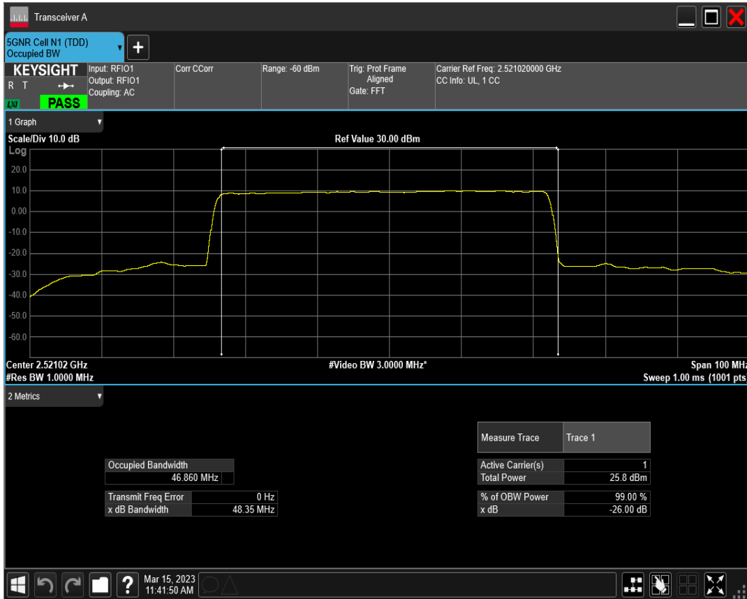
n41 SCS=30kHz DFT_QAM16 BW=50MHz Channel=504204 RB=128@0
