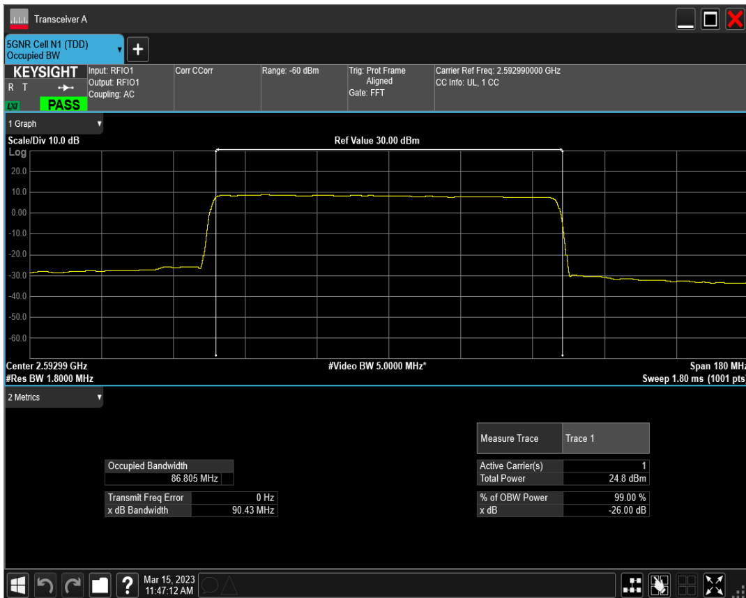
n41 SCS=30kHz DFT_QAM64 BW=90MHz Channel=518598 RB=240@0
